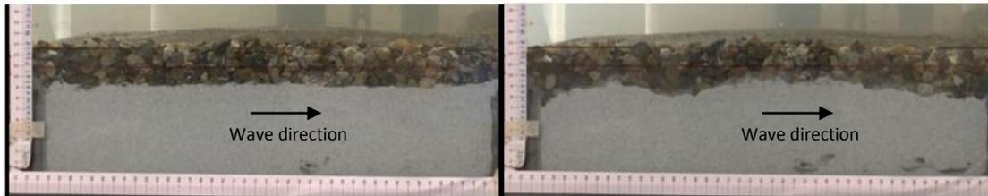
Figure 4-62 Test5b after 0 minutes (left) and after 70 minutes (right)
