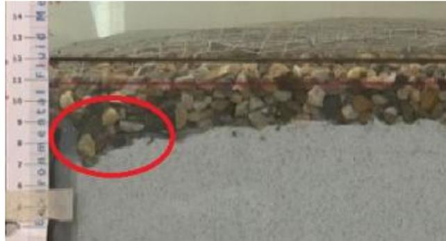
Figure 5-9 Test4d; clear water scour at the upstream side of the box
