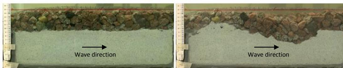
Figure 4-1 Test1a after 0 minutes (left) and after 125 minutes (right).
