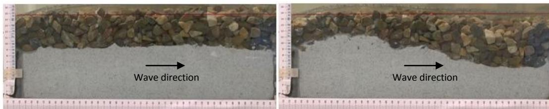
Figure 4-26 Test2d after 0 minutes (left) and after 125 minutes (right)
