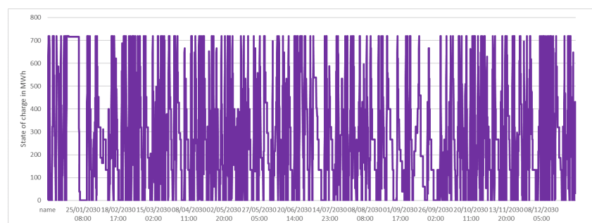
Figure 7.16: Annual trend of battery storage unit state of charge in Zeeland region
