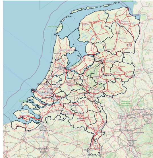
Figure 4.5: Electricity transmission lines following RES distribution made with QGIS
