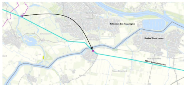
Figure 4.11: Relocation of Simonshaven substation
