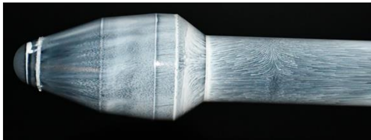
Figure 8: Oil flow visualization for Ma=0.8 , \alpha=4^\circ on Coe and Nute configuration.
