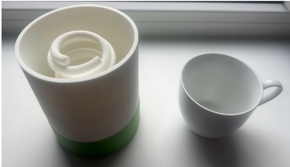
Figure 4.12: The 3D printed model of the reduced volume QWT system for final impedance tube measurements. 150 ml coffee cup for indication of scale. Masking tape applied to ensure casing fits exactly in impedance tube
