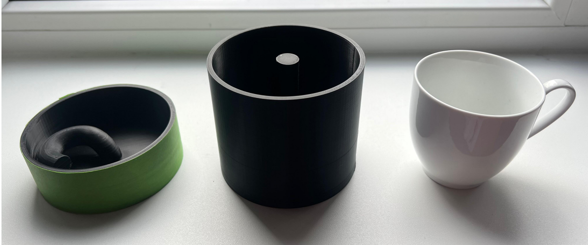
Figure 3.14: One bended and one straight 3D printed QWT with casing. L = 0.08 \text{ m} and d = 0.01 \text{ m} . 150 ml coffee cup for indication of scale. Masking tape applied to ensure casing fits exactly in impedance tube
