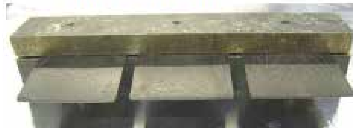
Figure 18. Deflection of the 20BS, 30BS, 40BS specimens (from left to right) at 120°C
