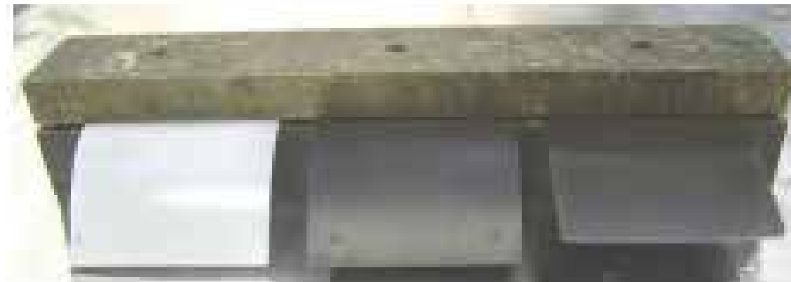
Figure 17. Deflection of the PLA, 15BN, 15BS specimens (from left to right) at 120°C
