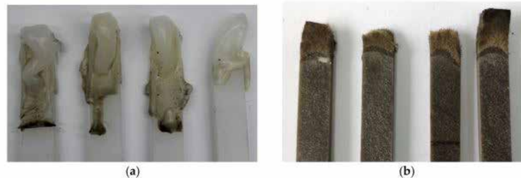
Figure 20: Dripping effect of PP vs BFRPP composite (Tang, Xu, & Li, 2019)
