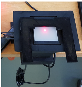
(b) The diffuser is placed on top of the PMMA plate containing the transmitting and receiving fibers. The moving object is placed over the diffuser.
