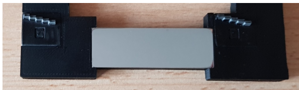
(a) The fully reflecting reference object, a metal piece polished to a mirror finish. The object is placed inside the slider.
