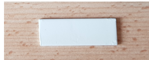
(b) The diffuser object, a metal piece with a layer of white paint.
