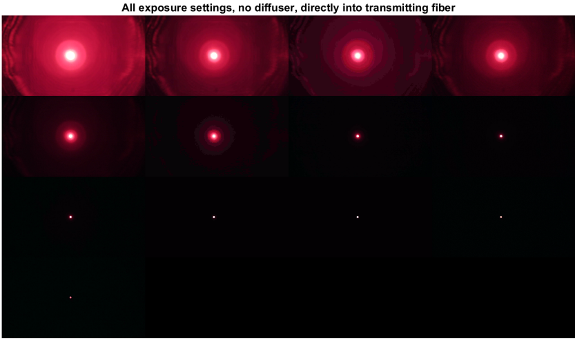
Figure 4.9: 13 images of the spot size directly looking into the transmitting fiber, without a diffuser, with all possible exposure settings. The highest exposure is the top left image, counting down from left to right and from top to bottom.
