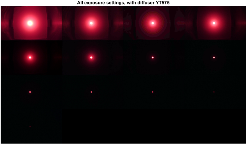
Figure 4.8: 13 images of the spot size of diffuser YT575, with all possible exposure settings. The highest exposure is the top left image, counting down from left to right and from top to bottom.
