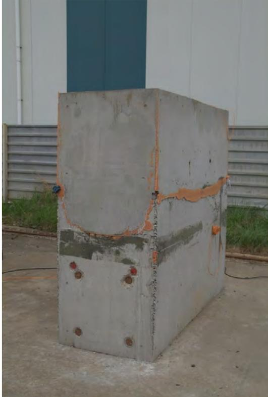
*Figure 52: Test block subjected to ER measurement*
