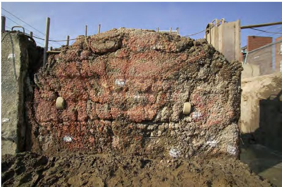
*Figure 97: Side view of the south face of panel 2 (worst parameters), the western panel 1 is just visible on the left and shows much better concrete*
