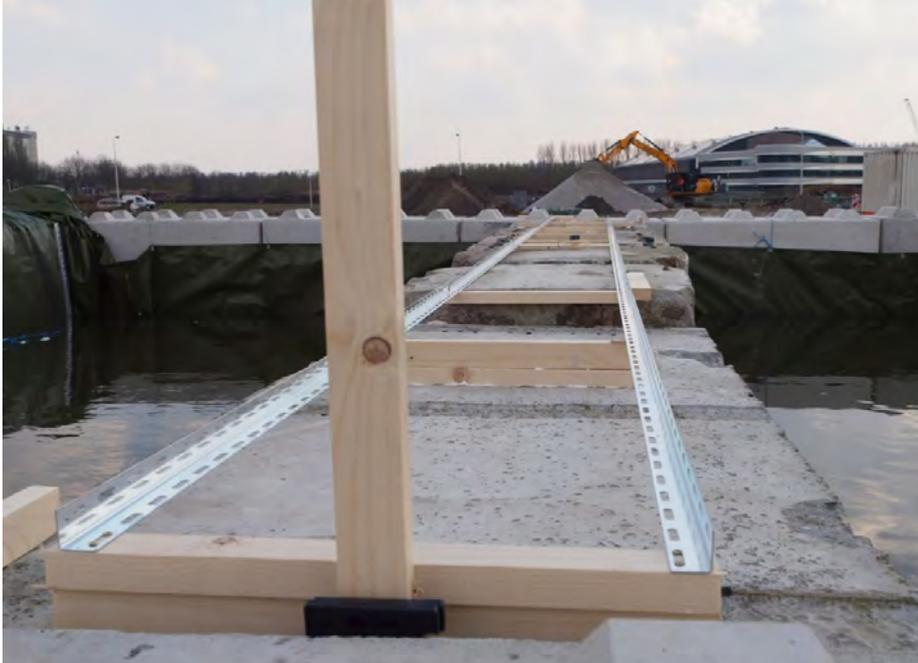
*Figure 57: Top of test wall with track for positioning the potential electrodes*
