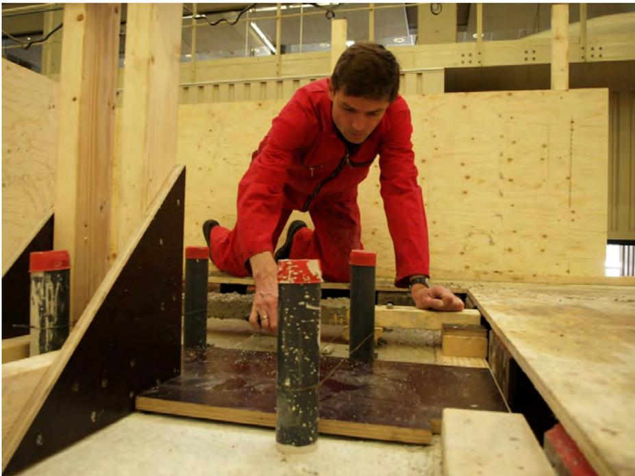
*Figure 10: Smooth finishing of the top of the test object*
