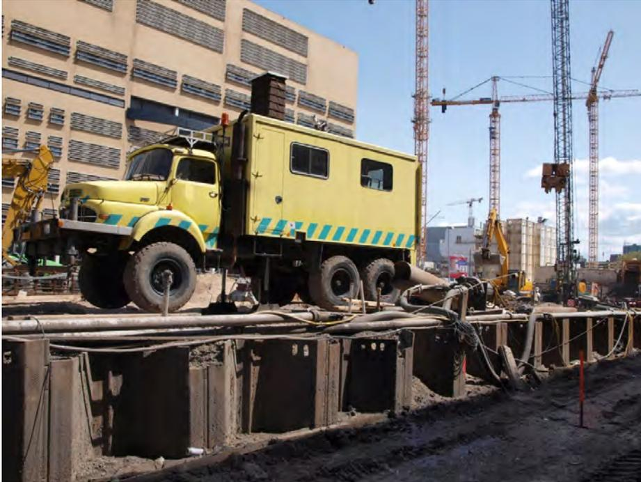
*Figure 50: CPT truck during resistivity measurements*
