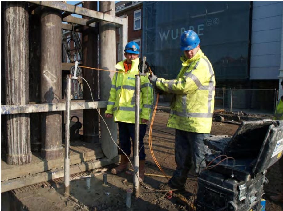
*Figure 8: CSL testing (Brem Funderingsexpertise BV) at 'Spoorzone' Delft*
