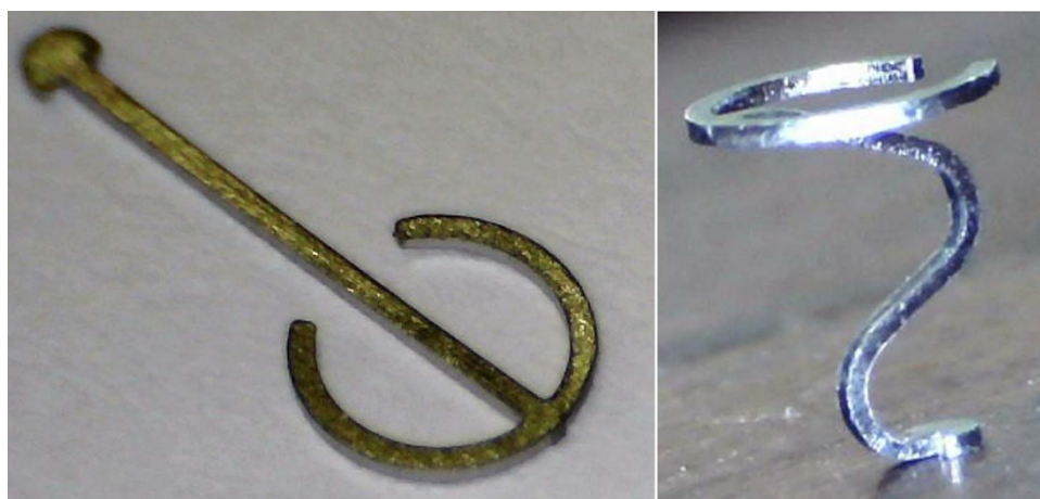
Figure 6. Unformed SM-T prototype (left) and a fully formed SM-T balancing on its footplate (right).
