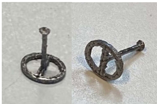
Figure 5. The 3DP-T prototype, after cleaning of support material and applying manual surface finishing.
