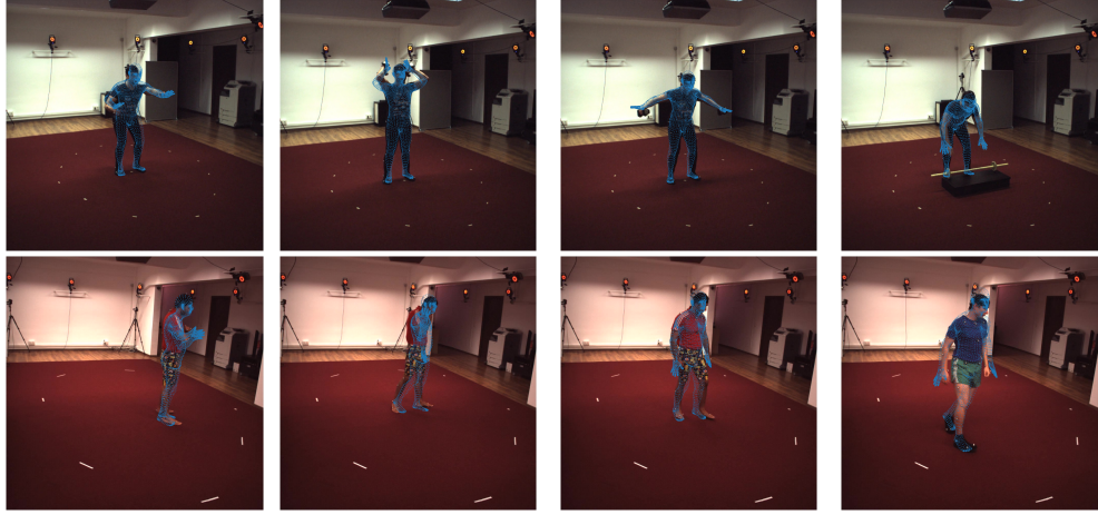
Figure 7: Qualitative results when projecting the SMPL body model from the OSDCap poses back to the input 2D images. The overlayed SMPL models are shown in sparse blue point cloud to maximize the visibility of the input human pose.
