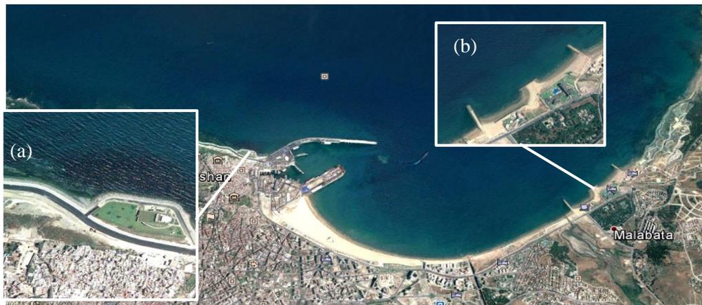
Figure 3-15 LST interruption structures (a) and shore protection structures (b) around Port of Tangier, Morocco
