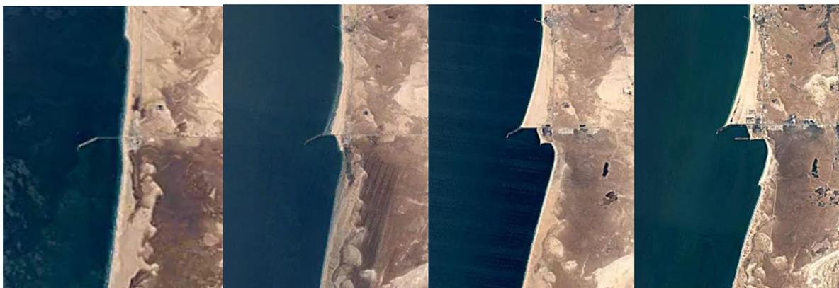
Figure 1-1 Satellite images of coastline evolution around Port of Nouakchott, Mauritania in 1984, 1994, 2004 and 2014 respectively (from left to right).
