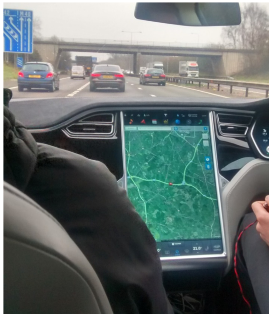
Fig. 3. Photo taken during the experiment: the participant on the right presses the handheld button when detecting a bridge. The safety driver is sitting in the left (passenger) seat. The vehicle in front is the lead vehicle the participant had to follow during the experiment.
