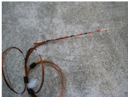
Figure 3-3. A series of thermocouples mounted on a wooden stick
