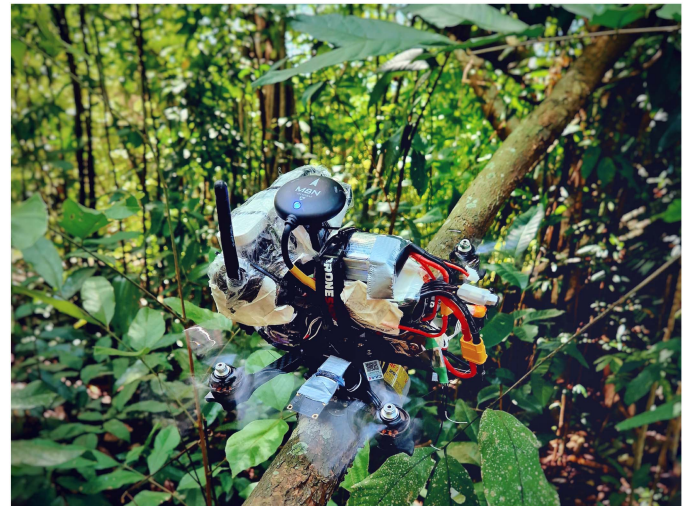
Fig. 1. Agile quadrotor perching on tree branches of steep incline during XPRIZE Rainforest semifinals, Singapore July 2023.
