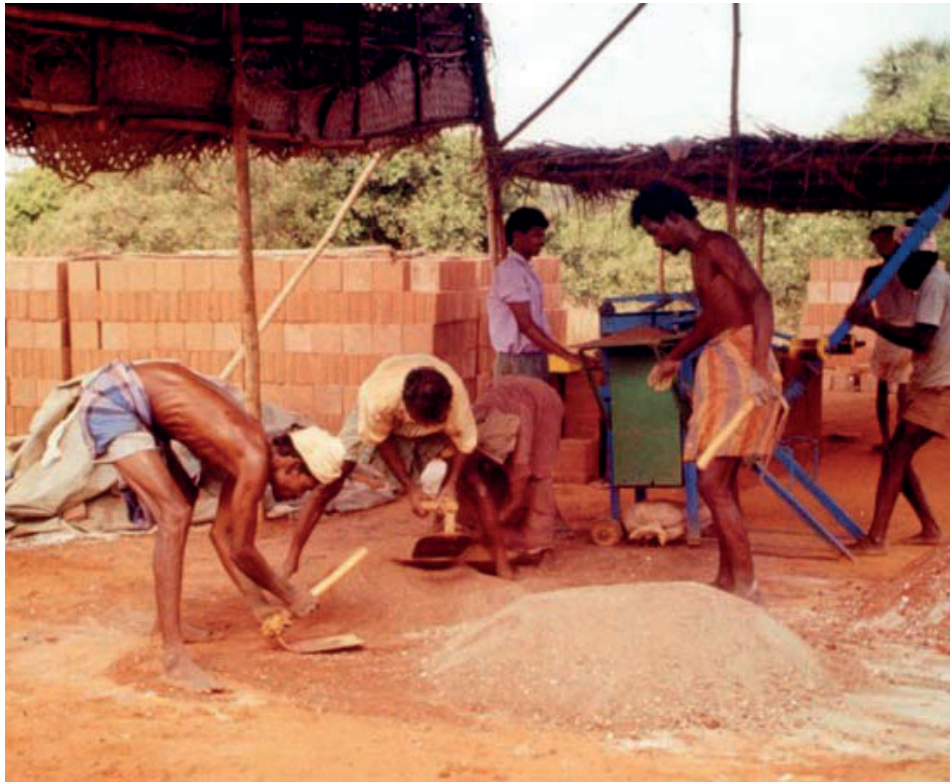
producing stabilized earth bricks on site
