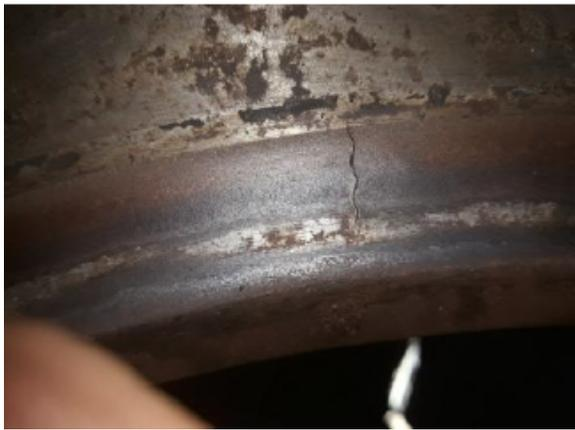
(a) Cylinder block contact surface crack
