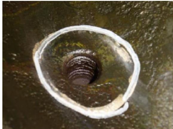
(b) Worn out threads of the piston crown
