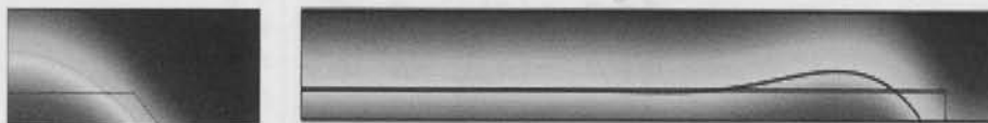
Figure 4.6. Final time step of FEM simulation, the value of level set function changes from 1 to zero from resist to air.
