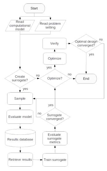
Figure 1: Diagram of the proposed framework
