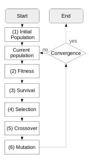
Figure 4: A generic flowchart of a genetic algorithm
