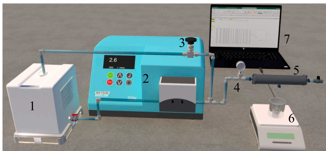
Fig. 1. Constant-flux setup for membrane filtration with components labeled as follows: (1) feed tank, (2) peristaltic pump, (3) needle valve, (4) pressure gauge, (5) membrane module, (6) balance, and (7) computer.
