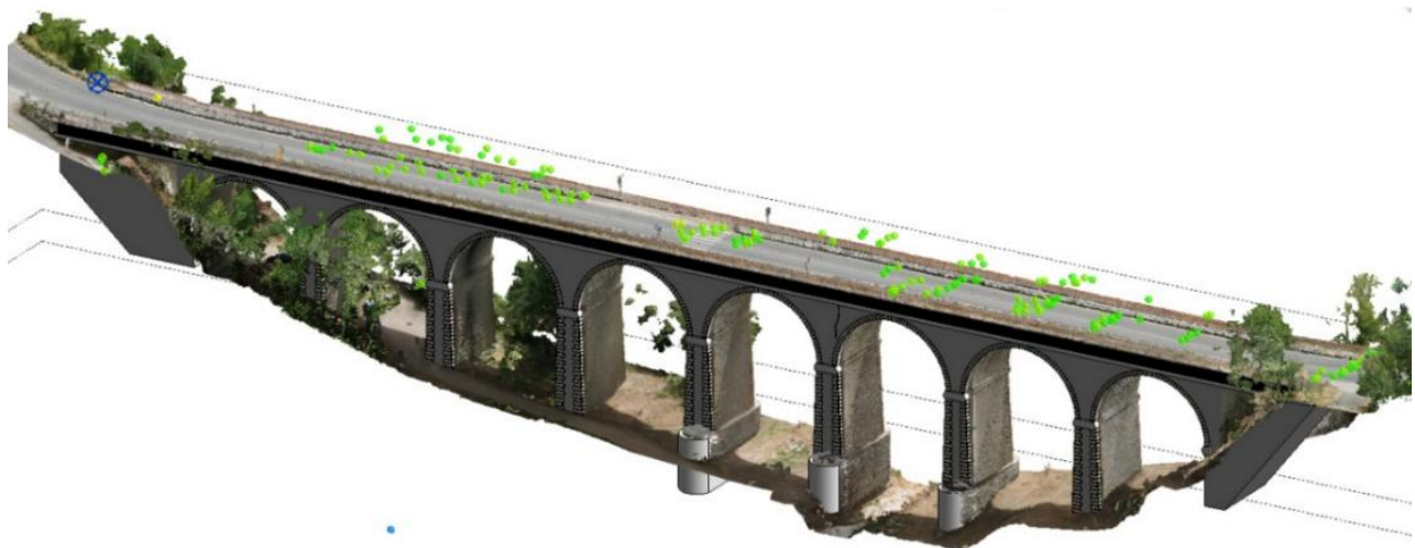
Fig. 5 Final BIM model enriched by PS data
