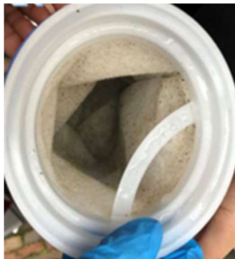
Figure 4-25 Visual observation of the 50 microns filter bag inner surface in Schuwacht (Jiaxing, 2017)
