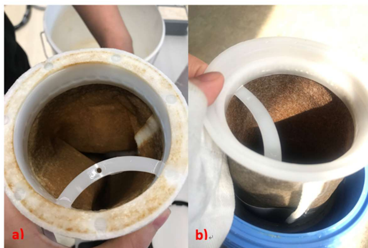
Figure 4-24 Visual observation of the filter bag after simulating for six month's water; a) TU Delft b) Kamerik.
