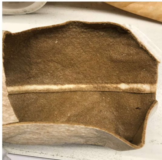
Figure 4-5 25 microns filter bag after running 177 hours.
