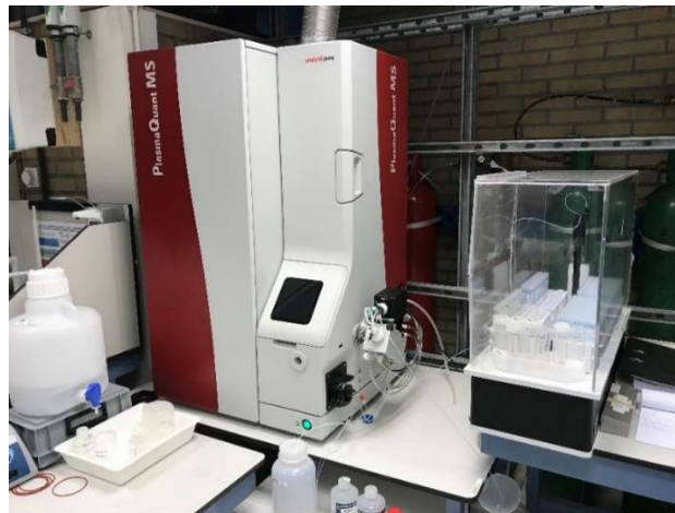
Figure 3-6 Inductively coupled plasma mass spectrometry (ICP-MS).
