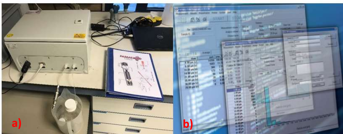
Figure 3-3 a) Pamas particle analyzer b) Software PAMAS PMA.
