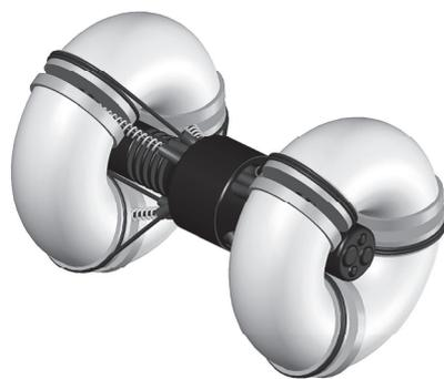
Fig. 2.16: An endoscopic device propelled by donuts constructed of metal gauze stents. (Adapted from [98].)
