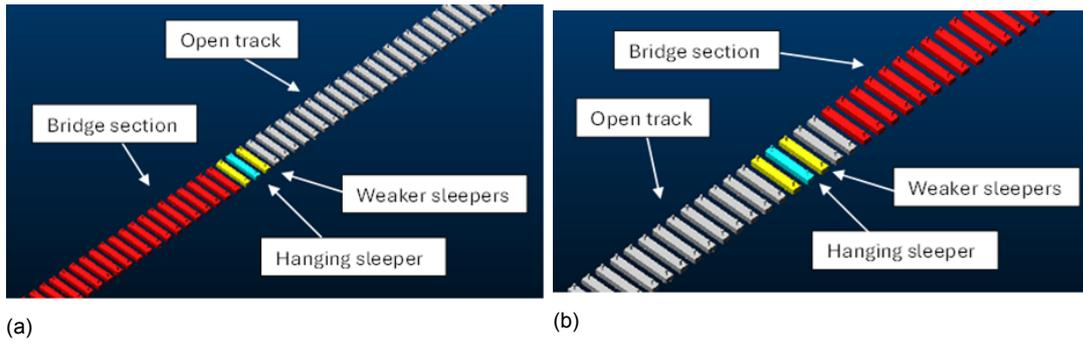
Figure F.14: Models of the (a) EB and (b) BE transition zones
