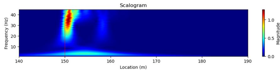
(c) Scalogram of the acceleration results. The red line marks the bridge ending
