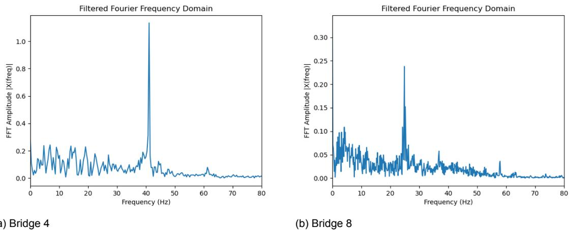
Figure 3.6: Fast Fourier Transform of filtered data
