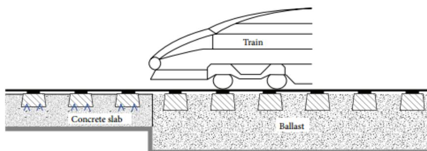
Figure 2.2: Ballast and slab track (Basirat, R., et al., 2017)
