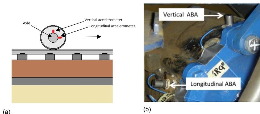
Figure 2.3: ABA setup. (a) schematic view of accelerometers of the axle. (b) in practise (Z. Li et al., 2015)
