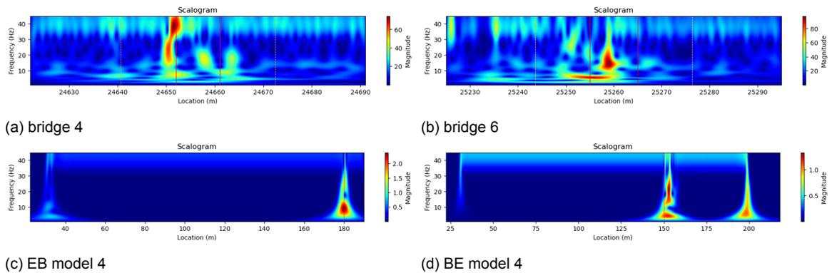
Figure 5.2: scalogram comparison between (a) bridge 4, (b) bridge 6, (c) EB of model 4 of the flextrack analysis and (d) BE of model 4 of the flextrack analysis
