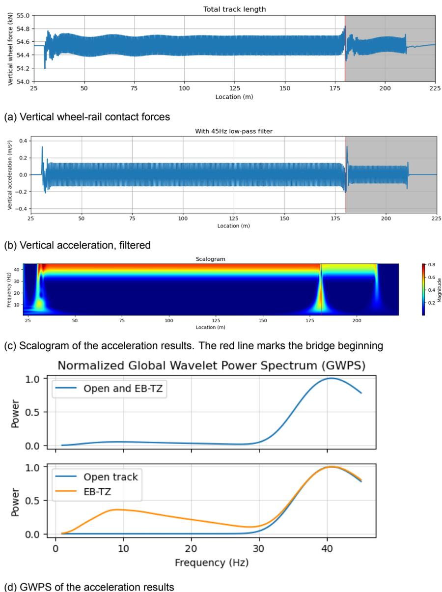
Figure F.2: Results from the differential stiffness EB model. In gray the rigid bridge section is plotted
