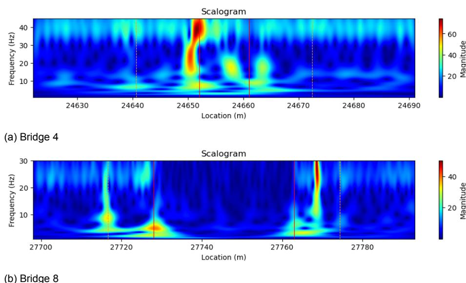
Figure 3.7: Continuous Wavelet Transform of filtered data. Red lines show bridge location, orange lines show assumed transition zone beginning and ending, respectively
