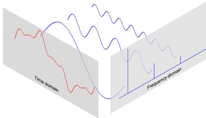
Figure 2.4: Fourier Transform visualisation (Kong, Q., et al., 2020)
