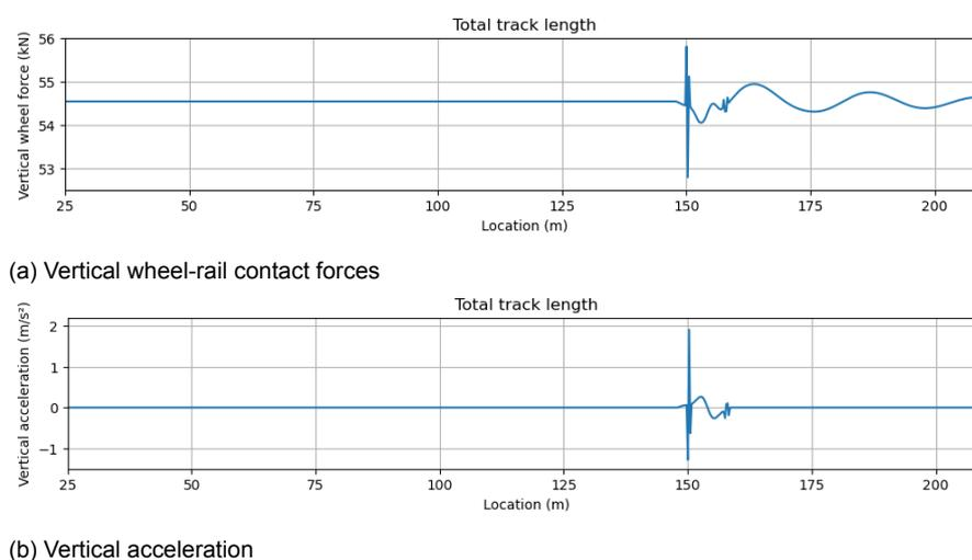
Figure 4.9: Results from the differential settlement model using the moving track
