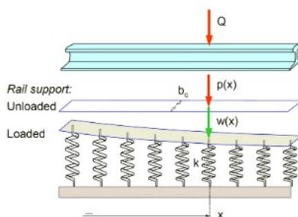
Figure E.1: A rail on an elastic foundation as stated by Zimmermann (TU Delft, 2020a)
