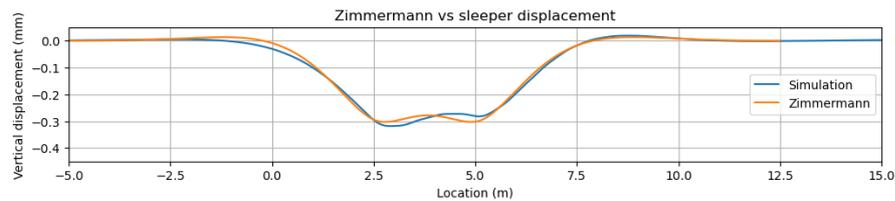
Figure 4.6: Analytical Zimmermann calculation vs the sleeper displacement of the normal track model
