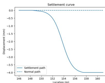
Figure 4.7: Introduced settlement curve starting at 150 meters (BE transition zone)
