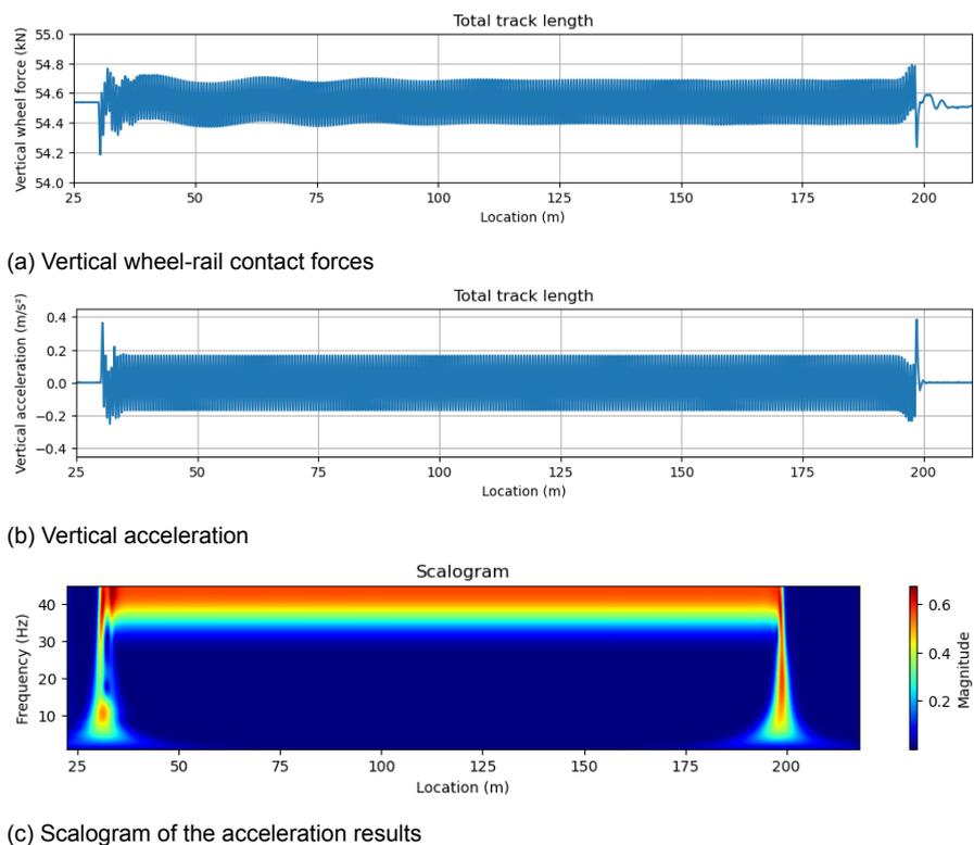
Figure 4.8: Results from the differential settlement model
