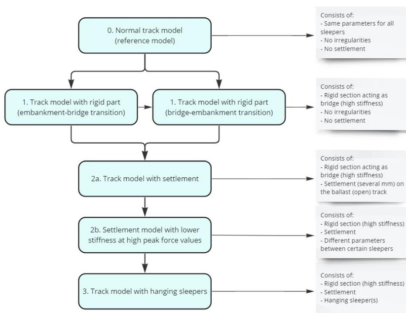
Figure 4.3: Track models. Each new model consists of the old model including its adjustments
