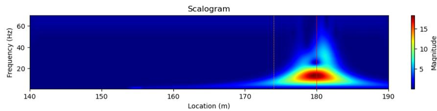
(c) Scalogram of the acceleration results. The red line marks the bridge beginning, the orange line the transition zone
