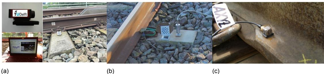
Figure A.1: a) VGS/DIC device set up (Wang, Markine, & Liu, 2018) b) Geophone (Le Pen, L., et al., 2018) c) Accelerometer (Vukušičová, D., 2017)
