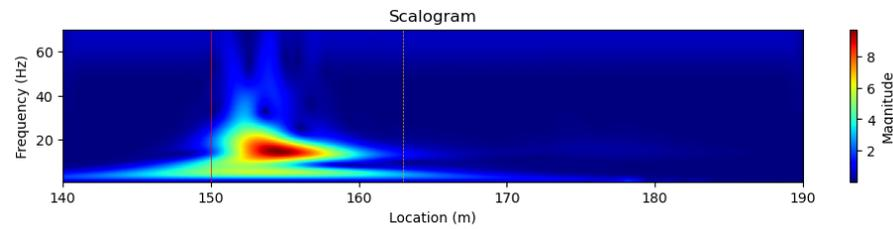
(c) Scalogram of the acceleration results. The red line marks the bridge ending, the orange line the transition zone
