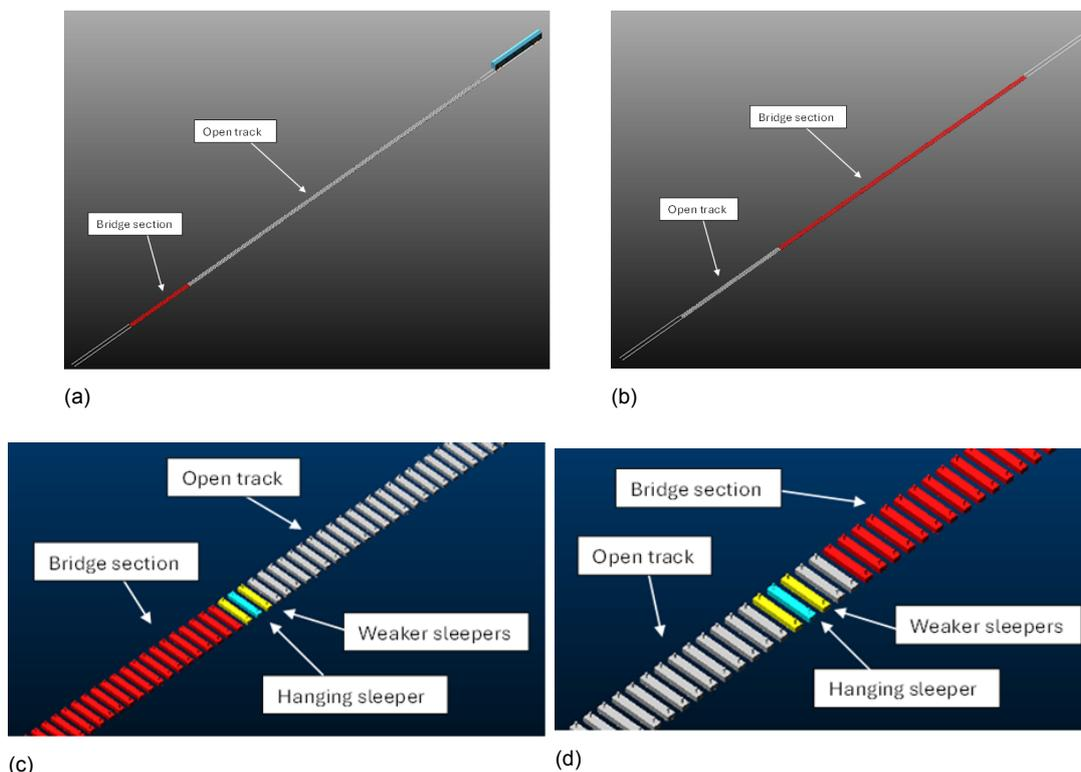
Figure 4.17: (a) Embankment-bridge model and (b) Bridge-embankment model. Close up for model 4 of the (c) EB and (d) BE transition zones
