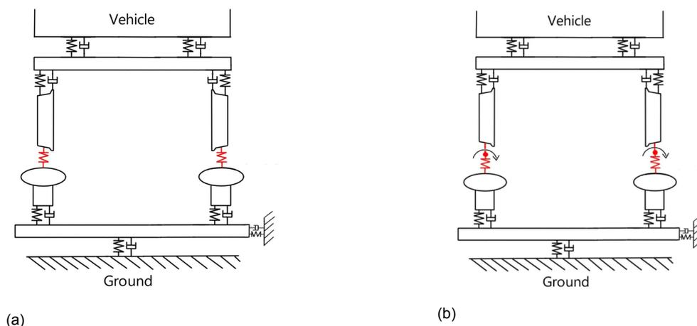
Figure 4.1: Schematic view of the moving track analysis MBS setup (left) and flextrack setup (right)
