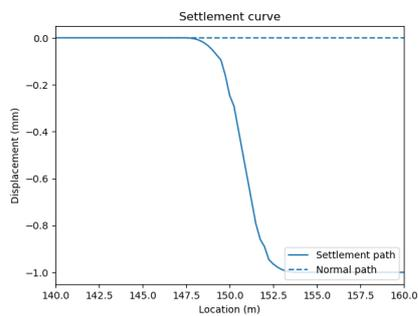
Figure F.4: Introduced settlement curve starting at 150 meters (BE transition zone)
