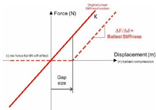
Figure 4.10: Relationship deformation and force (Bezin et al., 2009)
