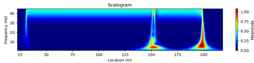
(c) Scalogram of the acceleration results. The red line marks the bridge ending
