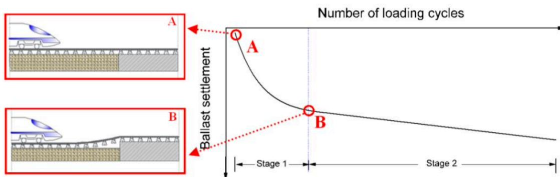
Figure 1.3: Permanent settlement process of the ballast during loading cycles (Wang, 2018)
