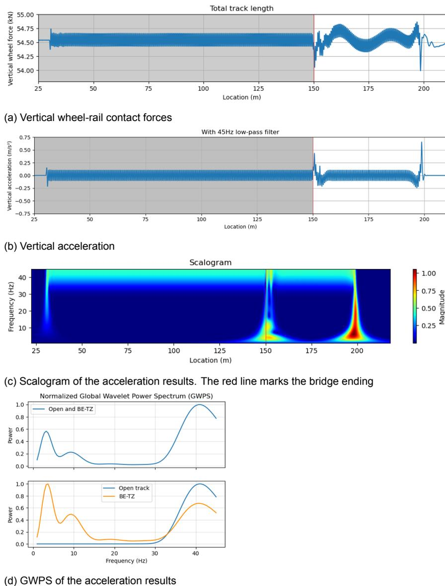
Figure F.11: Results from the BE model 2 using flextrack. In gray the rigid bridge section is plotted
