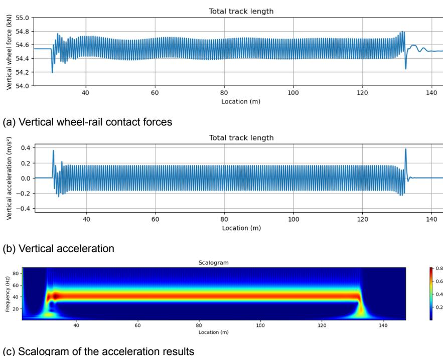
Figure 4.5: Results from the normal track model
