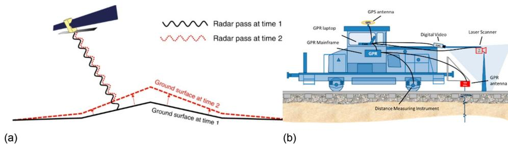
Figure A.3: a) InSAR principle (Biggs, J., et al., 2020) b) GPR principle (Wang, H., et al., 2017)
