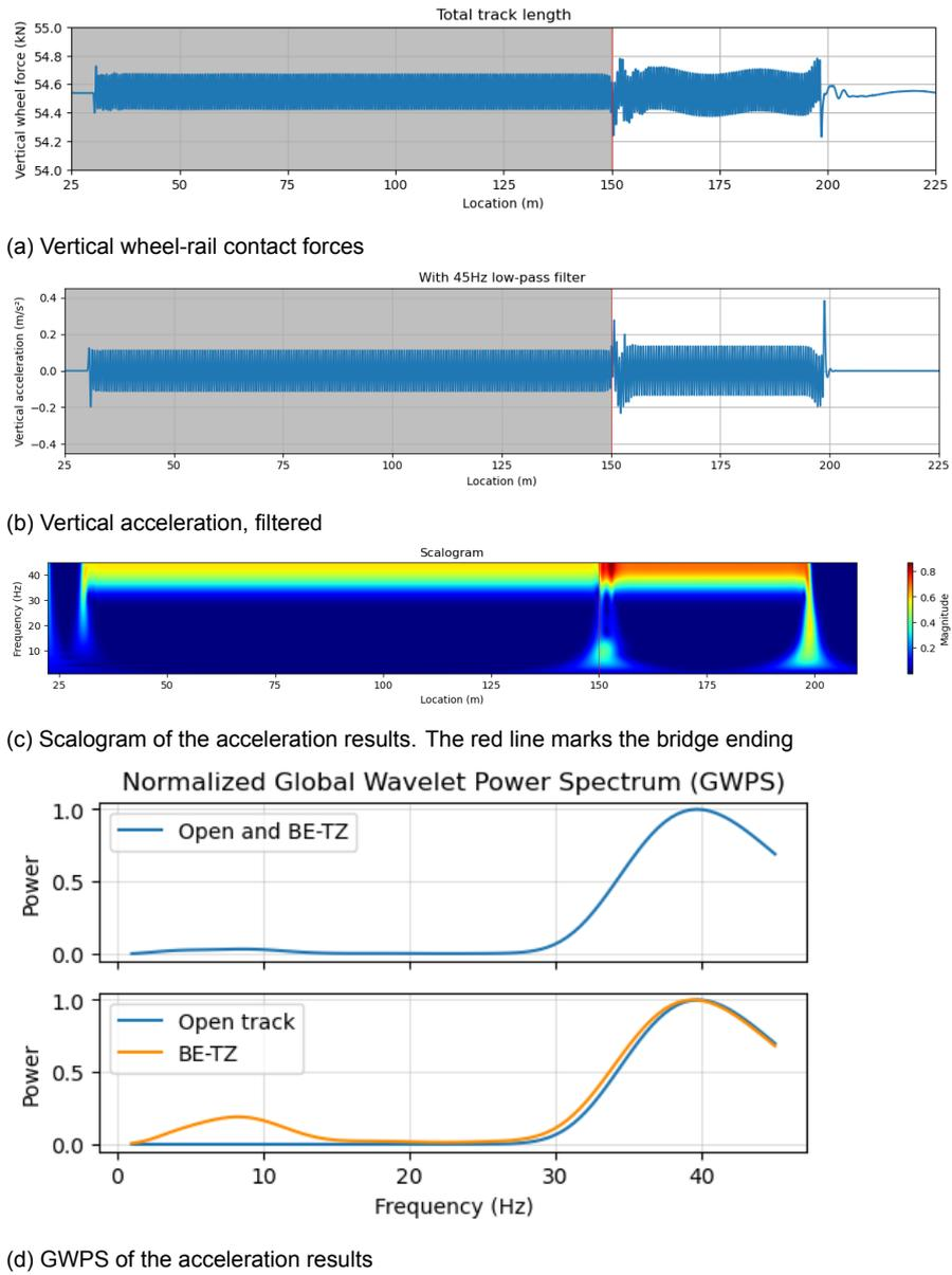
Figure F.3: Results from the differential stiffness BE model. In gray the rigid bridge section is plotted
