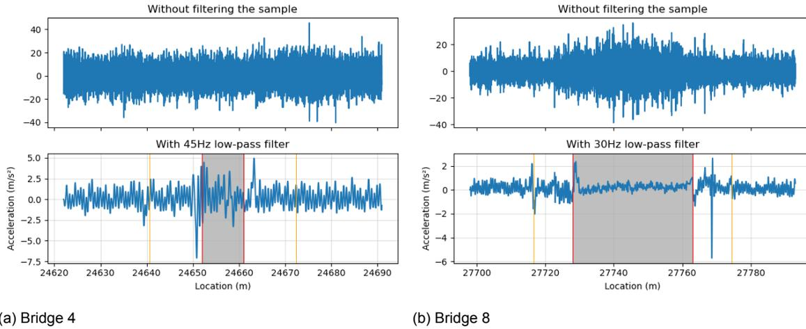
Figure 3.3: Selected data from bridge 4 (a) and 8 (b). The red lines mark the start and end of bridge and orange lines mark the start and end of the transition zone
