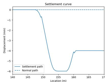
Figure 4.14: Introduced settlement curve starting at 150 meters (BE transition zone)
