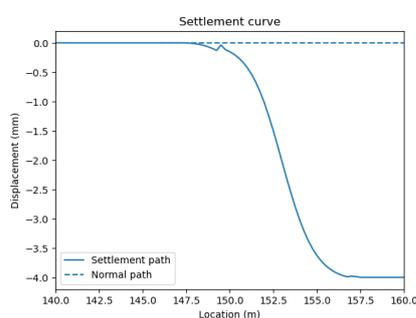
Figure F.7: Introduced settlement curve starting at 150 meters (BE transition zone)
