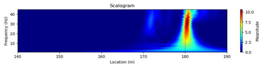
(c) Scalogram of the acceleration results. The red line marks the bridge beginning
