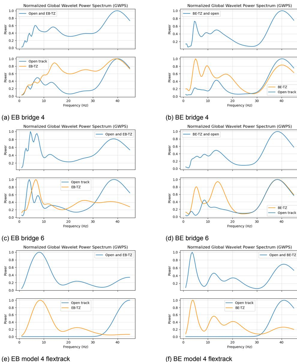
Figure 5.3: GWPS comparison between (a) EB of bridge 4, (b) BE of bridge 4, (c) EB of bridge 6, (d) BE of bridge 6, and (e) EB of model 4 of the flextrack analysis and (f) BE of model 4 of the flextrack analysis
