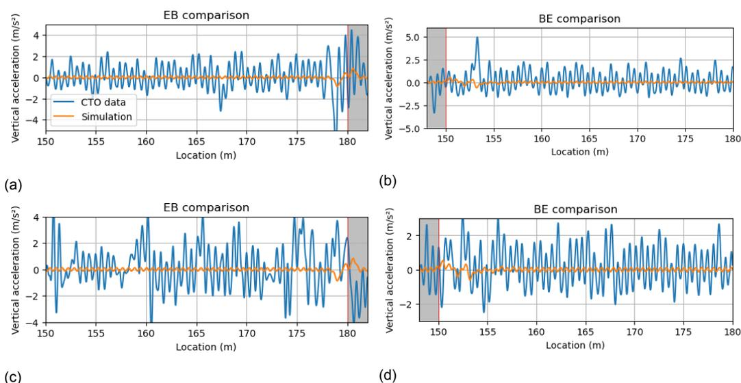
Figure 5.1: Comparison of the simulation and measurement data for (a) bridge 4 EB transition zone, (b) bridge 4 BE transition zone, (c) bridge 6 EB transition zone, (d) and bridge 6 BE transition zone
