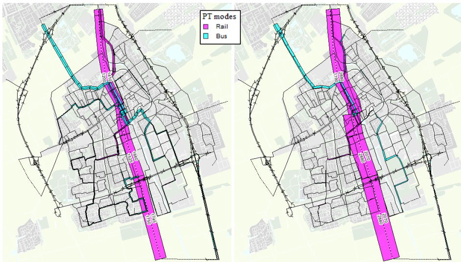
Figure 2.9. Average public transport flows ( \text{h}^{-1} ) between 17:30 and 18:00 for the Delft case study on a normal day (left) and in the evacuation scenario (right). Bar widths are proportional to flow, colours indicate public transport mode.
