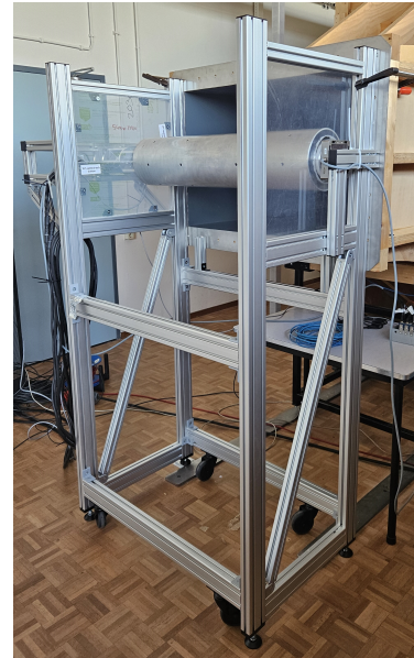
(b) Installed model and supports in the SLT facility.
