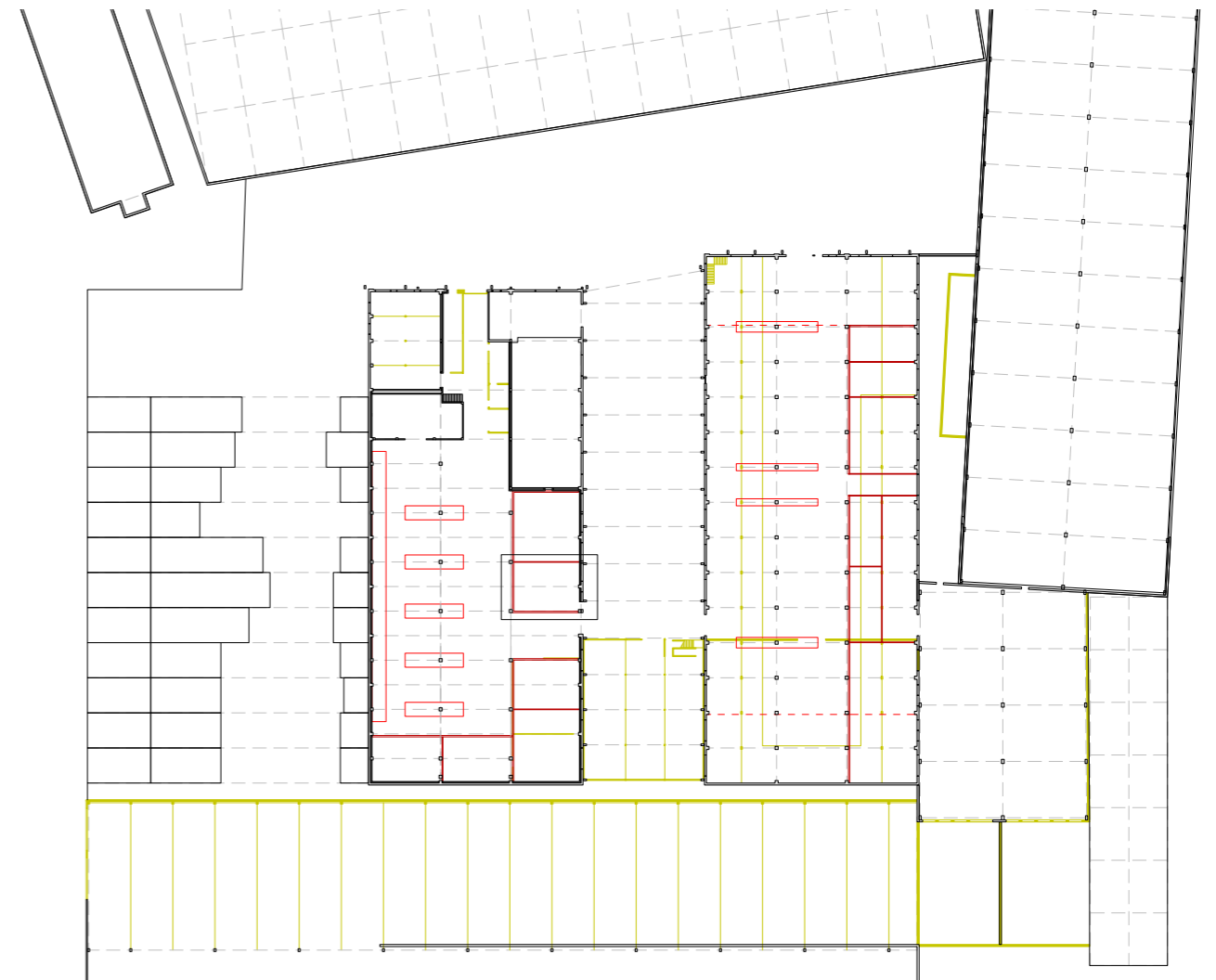
Ground floor plan black (existing), yellow (dismantled), red (added), scale 1 : 500 (scaled to 1 : 1000)
