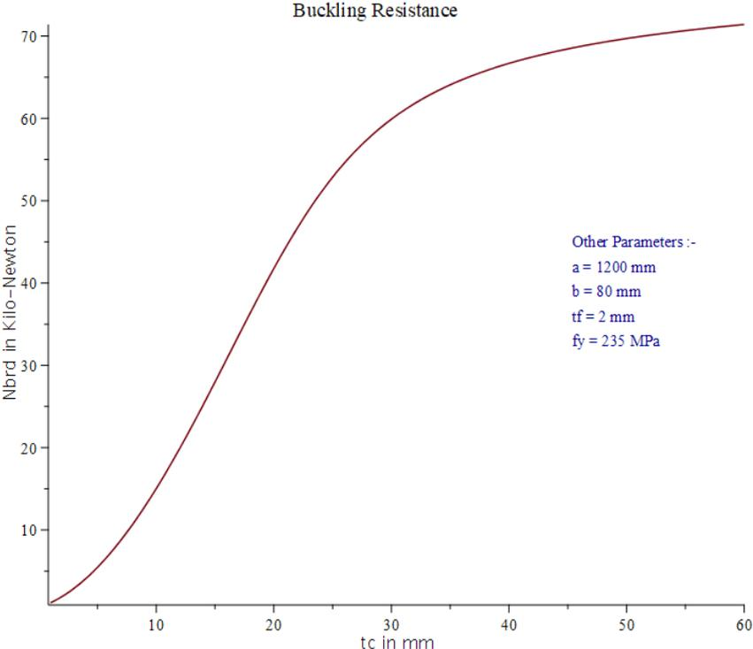
Figure 3.13 Effect of thickness of core on the buckling load
