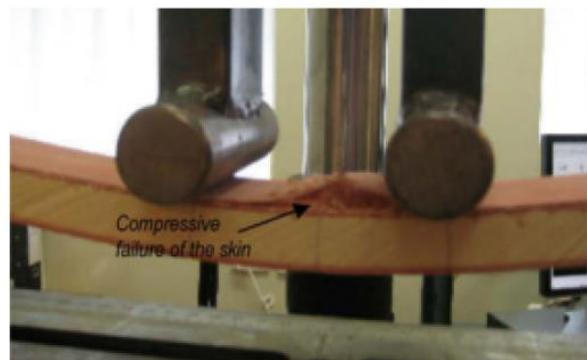
B. Compressive facing failure in flatwise bending.
