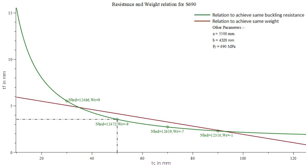
Figure 4.13 Relation between the thickness of faceplate and core for buckling resistance and weight
