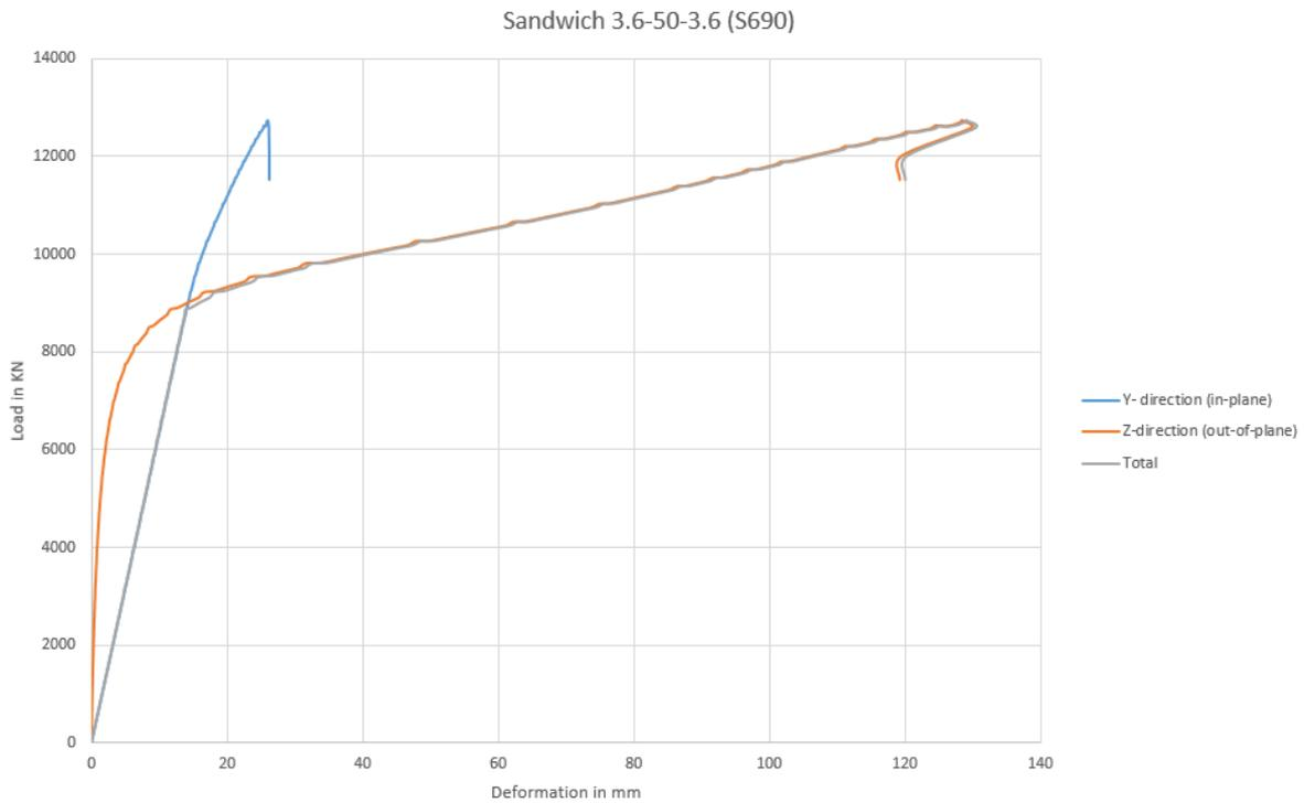
Figure D.8 Nonlinear Buckling Analysis of Sandwich S690
