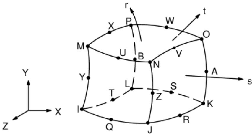
Figure A.2 ANSYS element type SOLID186 [9]
