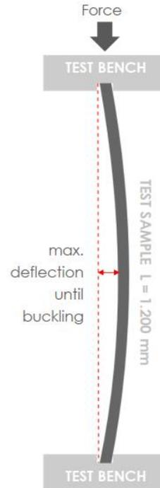
Figure 3.20 Test setup and apparatus of Havel experiment
