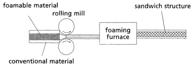
Figure 2.8 Schematic processes for of production of steel sandwich with aluminium foam core [18]
