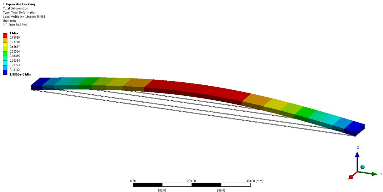
Figure A.8 First Eigen buckling load calculated with ANSYS
