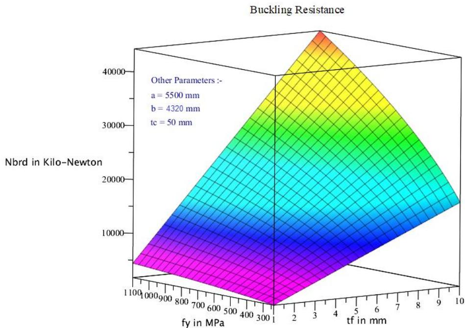
Figure 5.5 Effect of thickness and yield strength of faceplate on buckling load simultaneously
