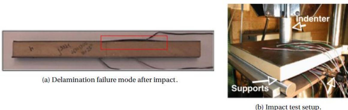
Figure 2.10 Indentation and Impact Failure [38]
