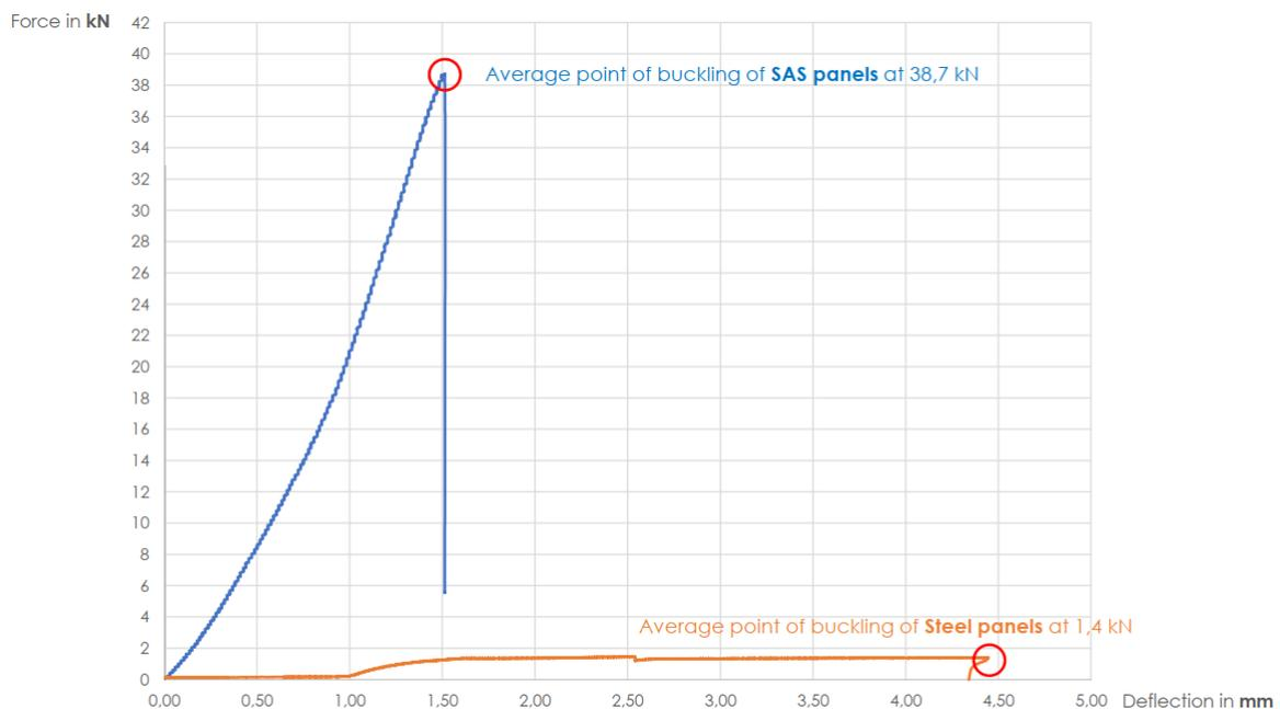
Figure 3.21. Graph between applied load and corresponding displacement
