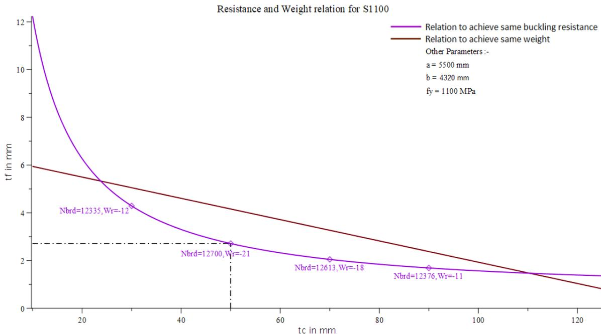
Figure 4.15 Relation between the thickness of faceplate and core for buckling resistance and weight
