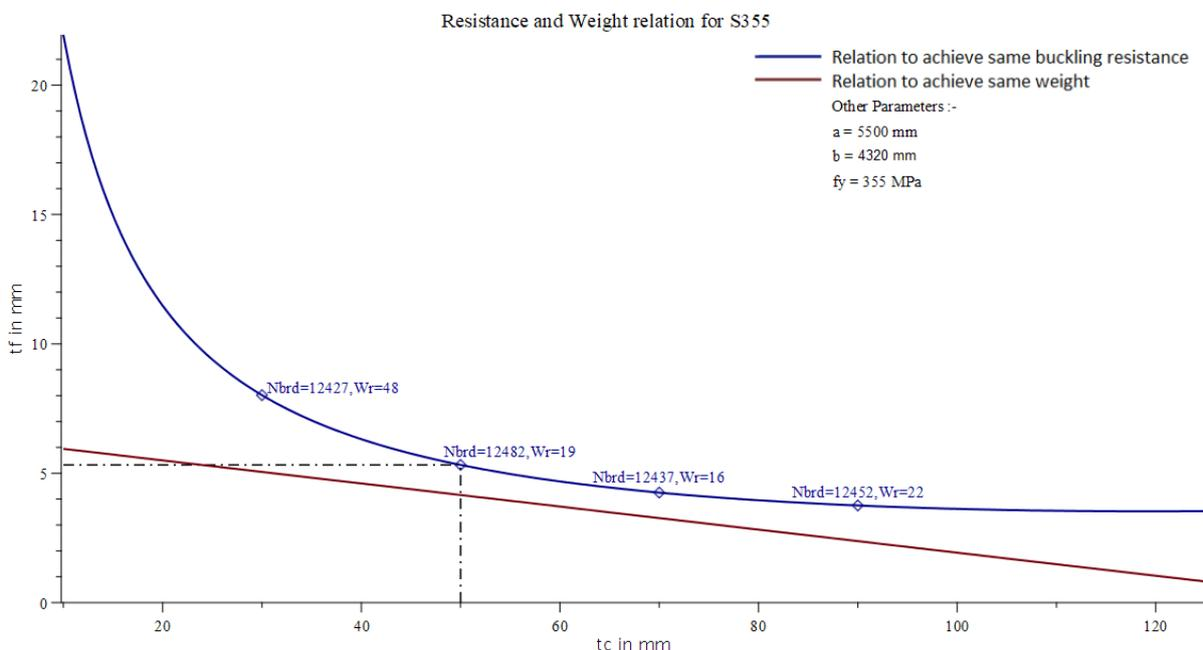
Figure 4.11 Relation between the thickness of faceplate and core for buckling resistance and weight
