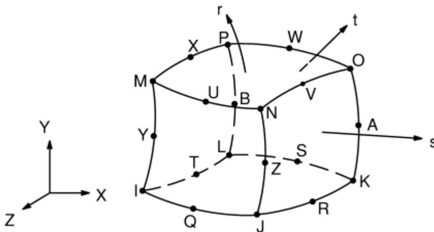
Figure D.2 ANSYS element type SOLID186 [9]
