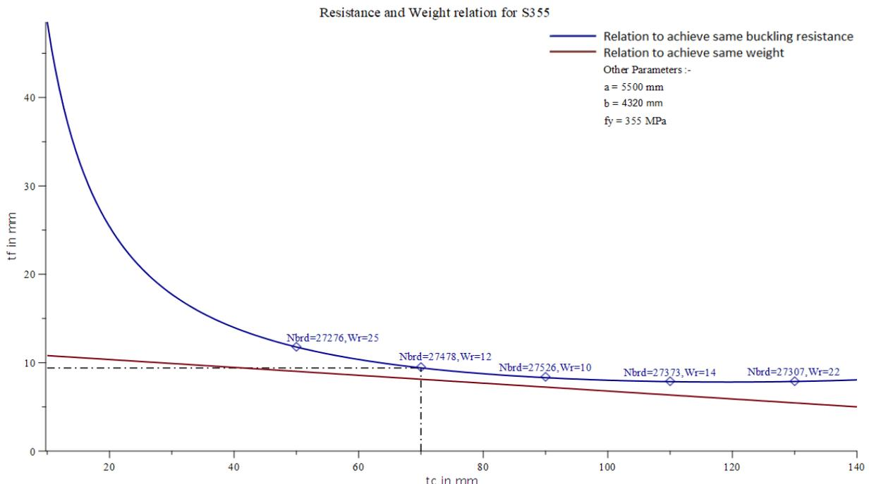
Figure G.3 Relation between the thickness of faceplate and core for buckling resistance and weight
