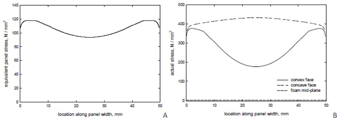
Figure 2.6 Resistance mechanism of sandwich panels: A. integral through-thickness (effective compressive resistance) expressed in terms of equivalent smeared stress, B. stress distribution in convex steel face, concave steel face and foam mid-plane.
