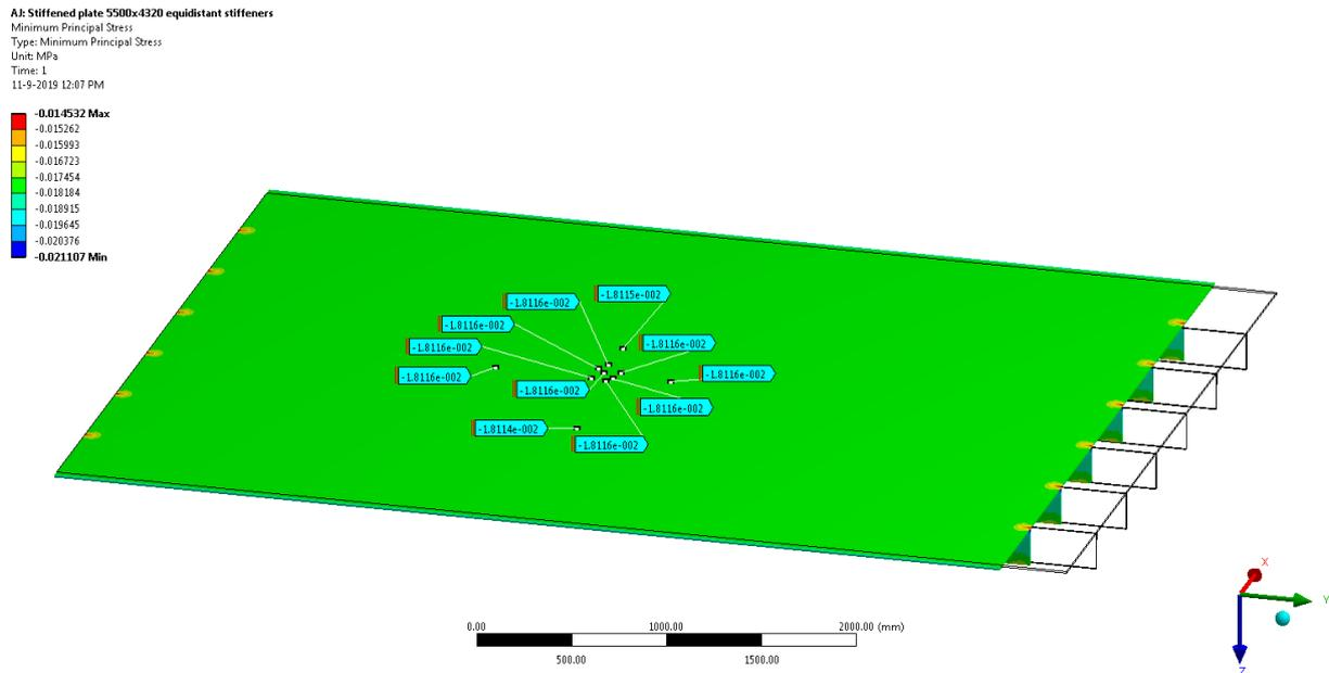
Figure B.7 Minimum principle stress calculated with ANSYS
