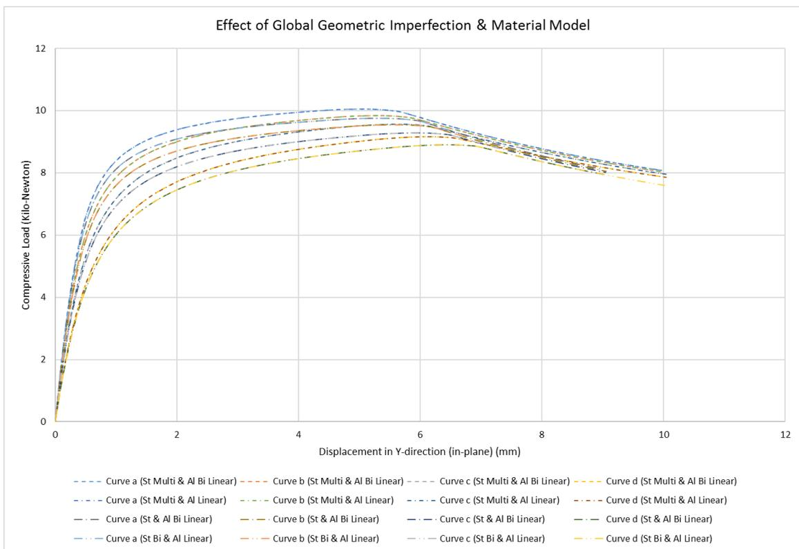
Figure 3.7 Graph between In-plane displacement vs Compressive Load (Global Imperfection)
