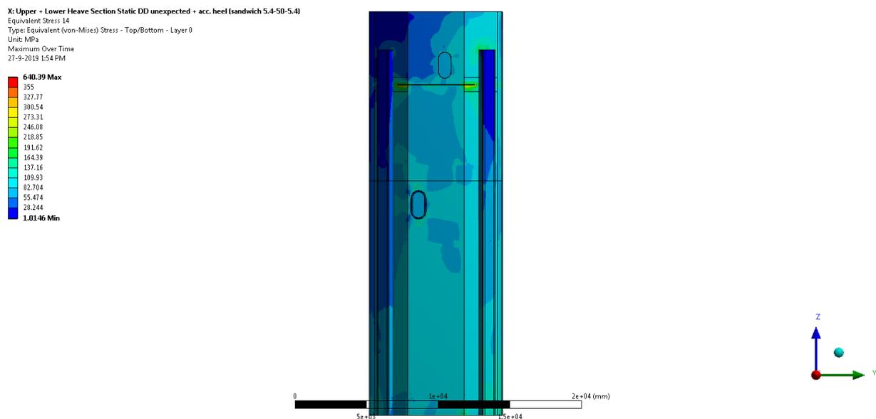
Figure 6.4 Von Mises stress (front view)
