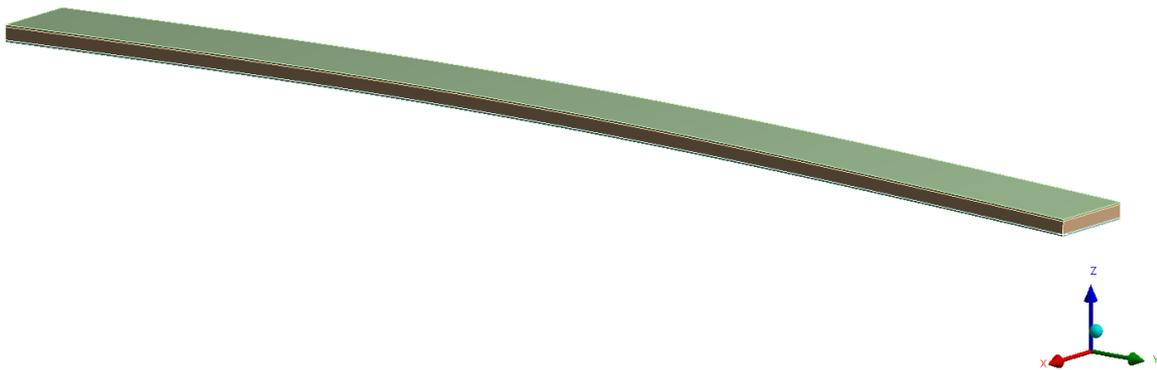
Figure A.6 Model of sandwich panel with global geometric imperfection
