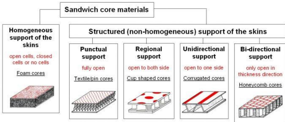
Figure 2.4 Types of material used for core [25]
