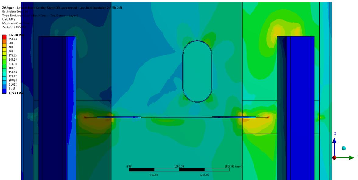
Figure 6.24 Von Mises stresses at joints
