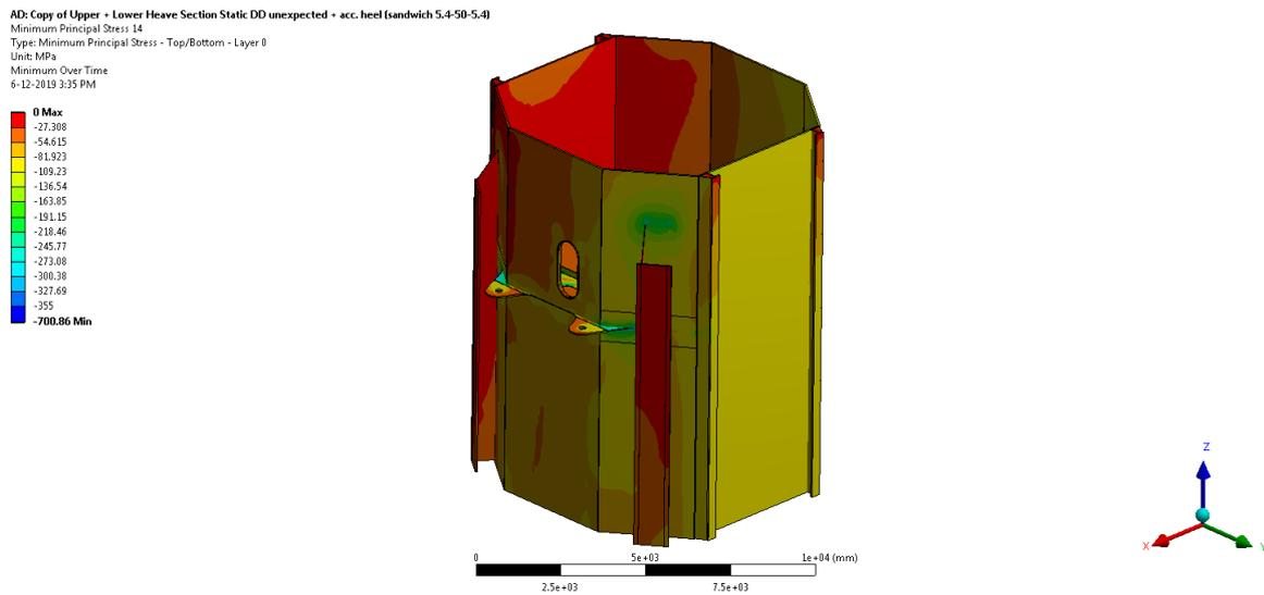
Figure 6.7 Minimum principle stress (upper part)
