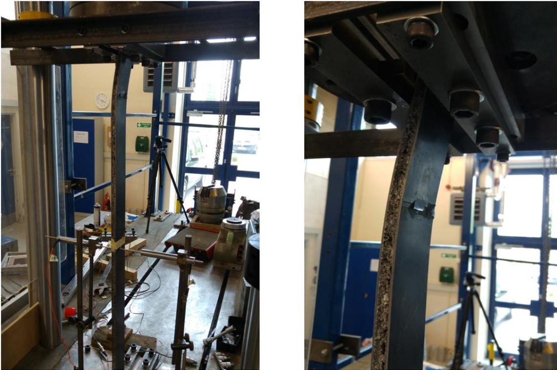
Figure 3.22 Buckling mode of sandwich panel
