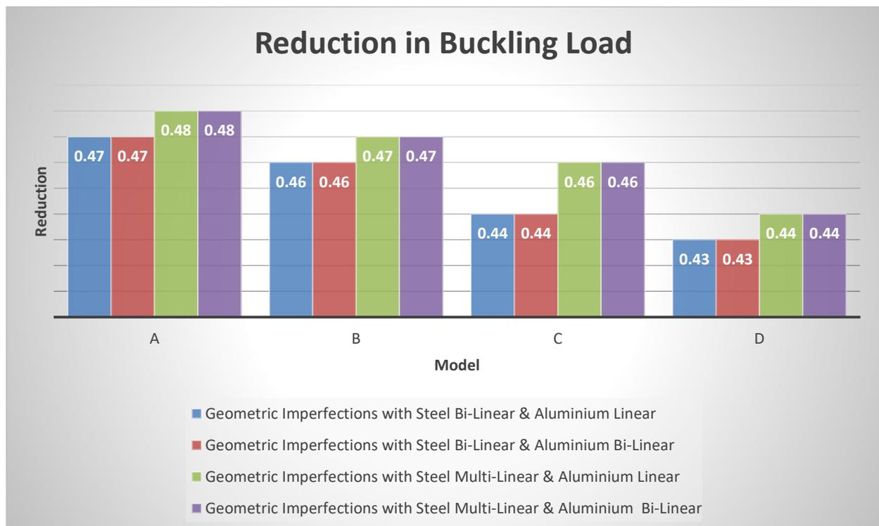
Figure 3.15 Graphical representation of reduction in buckling load for considered global geometric imperfection & material models
