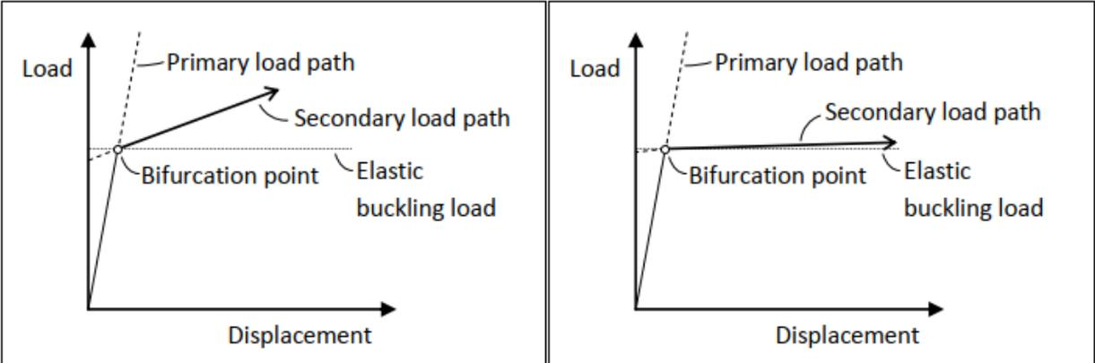
Figure 2.19 load-displacement diagram for elastic buckling (left: plate, right: column).[10]
