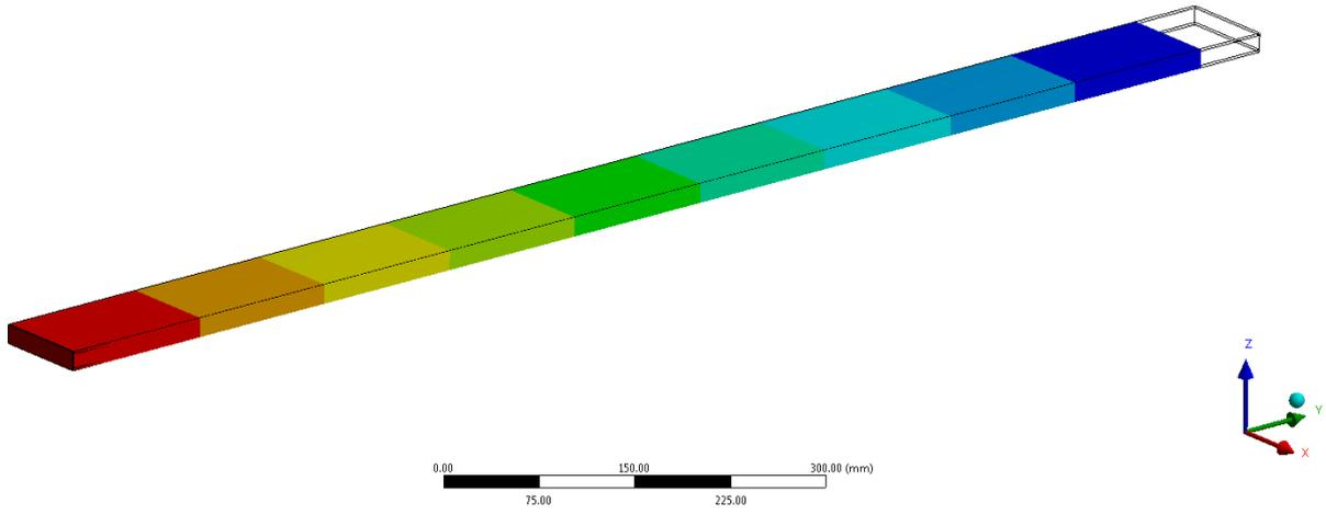
Figure 3.8 In-plane displacement of sandwich panel
