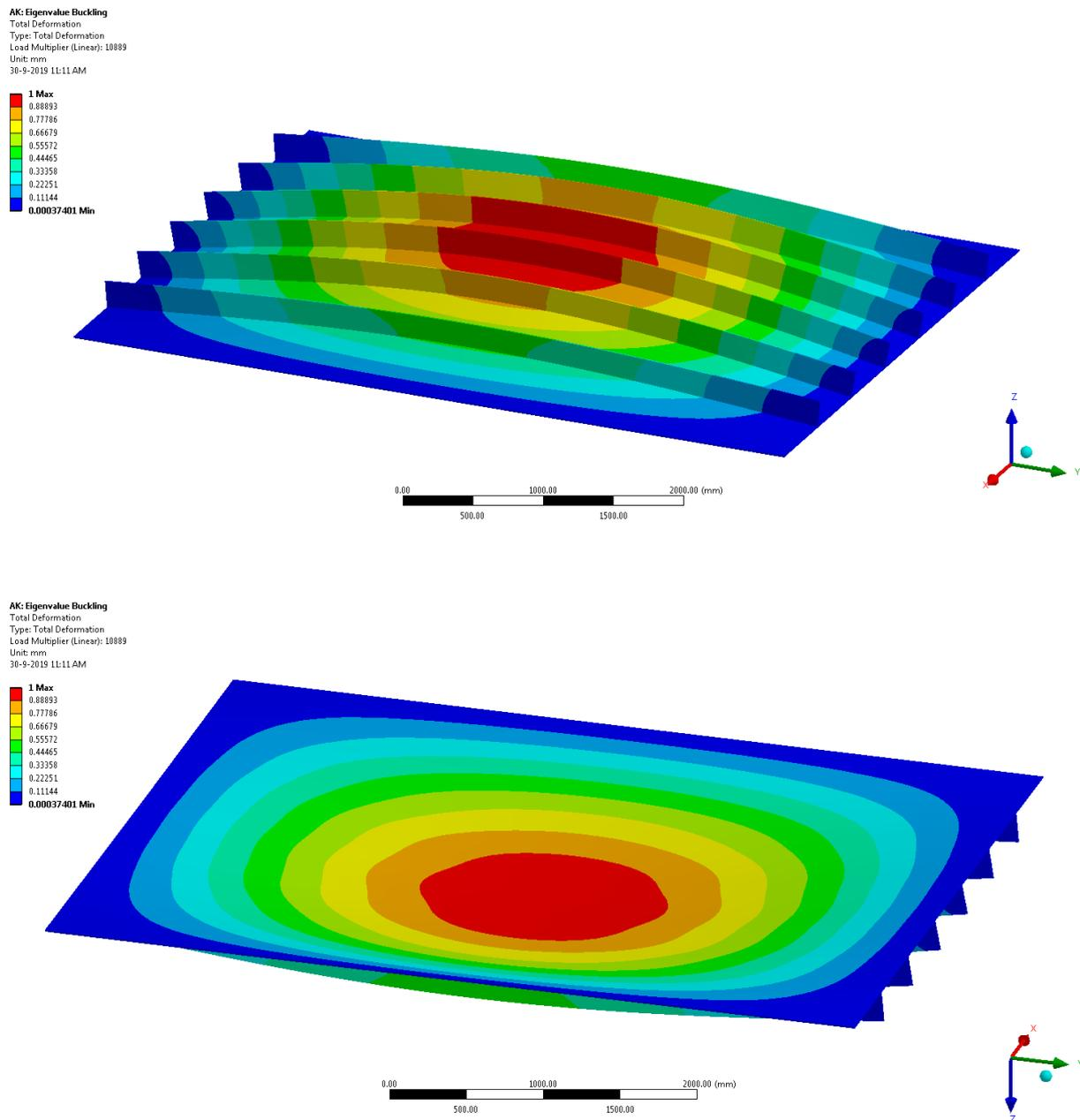
Figure B.6 First Eigen buckling load calculated with ANSYS
