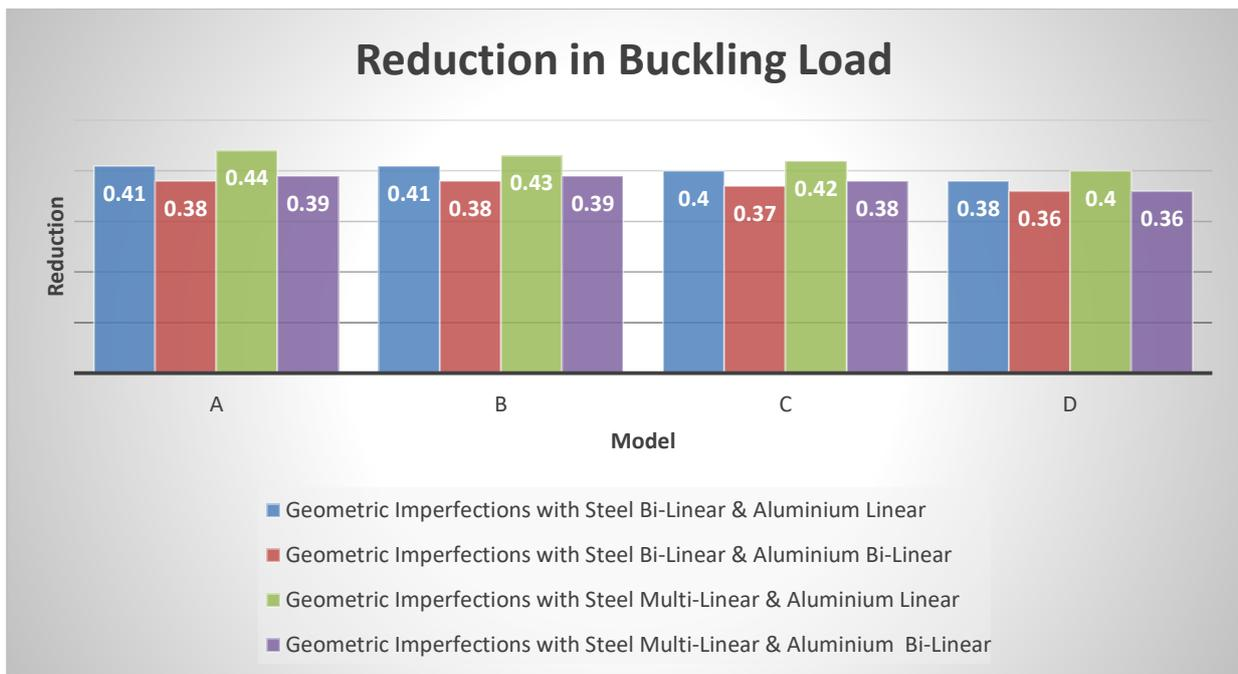
Figure 3.16 Graphical representation of reduction in buckling load for considered global & local geometric imperfection and material models
