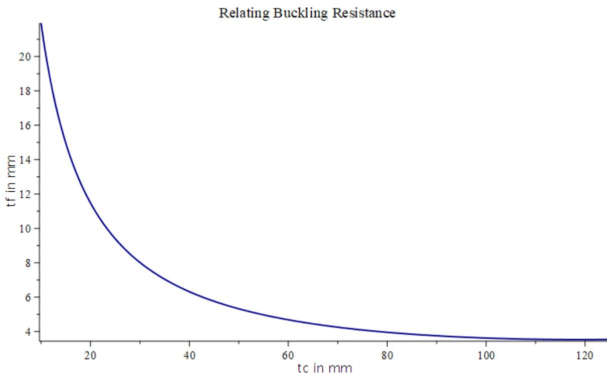
Figure 4.9 Relation between the thickness of the core and faceplate to achieve the same buckling resistance of the stiffened plate
