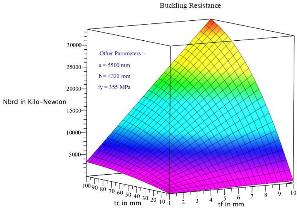
Figure 5.4 Effect of thickness of faceplate and core on buckling load simultaneously
