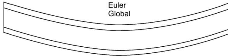
Figure 4.4 Global buckling of the sandwich panel under compressive loading [8]
