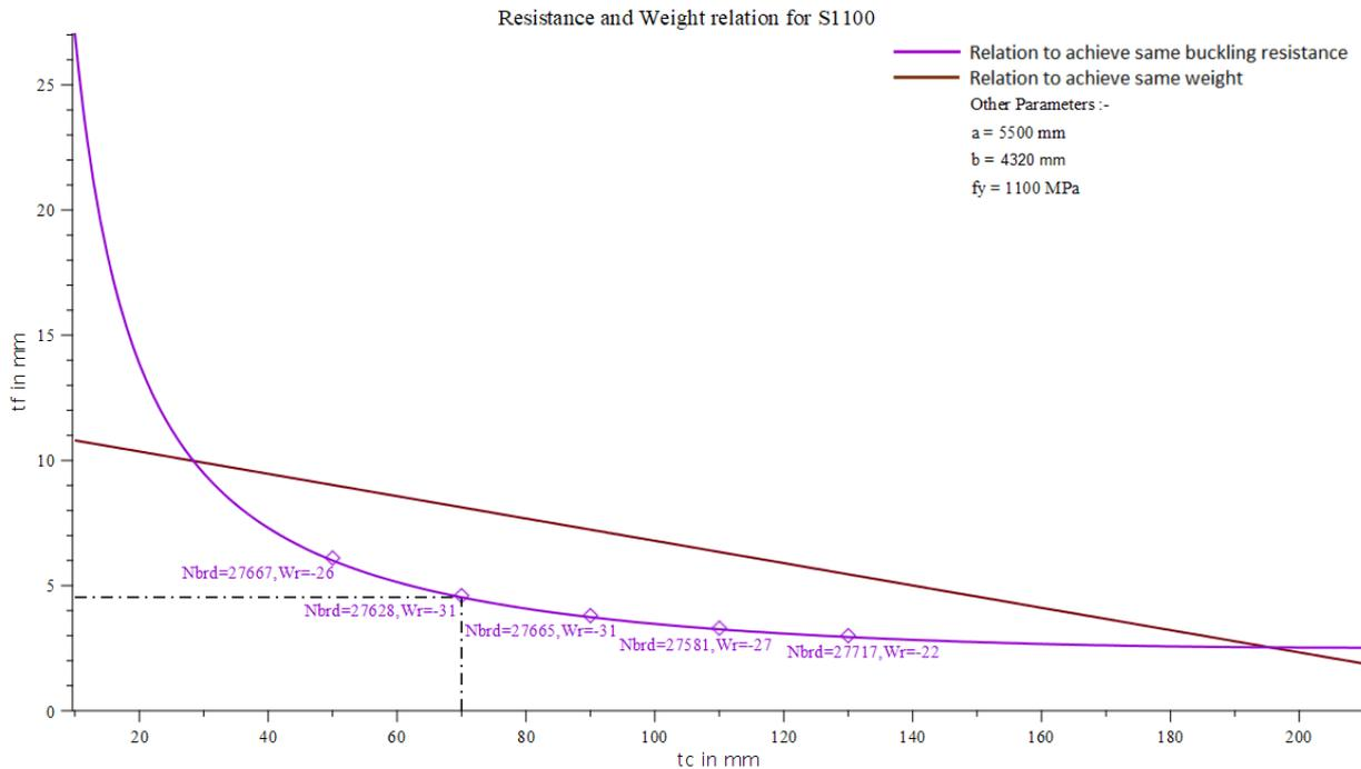
Figure G.7 Relation between the thickness of faceplate and core for buckling resistance and weight
