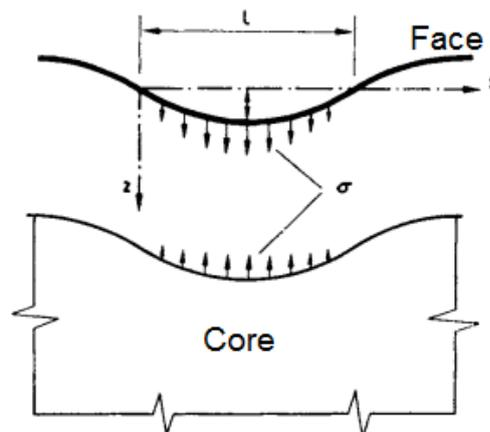
Figure 3.23 Stress between the faceplate and supporting elastic medium (core)
