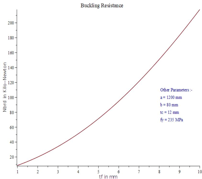
Figure 3.12 Effect of thickness of faceplate on the buckling load
