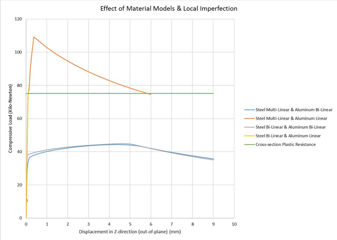
Figure 3.11 Graph between Out-plane displacement vs Compressive Load (Local Imperfection)
