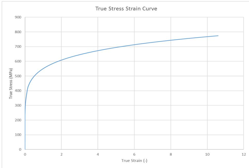
Figure 3.2 Steel material model Multi-linear
