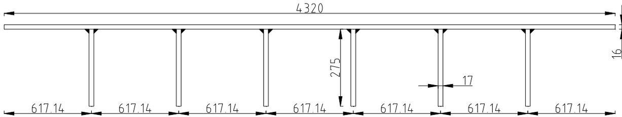
Figure G.2 Cross-section of stiffened plate
