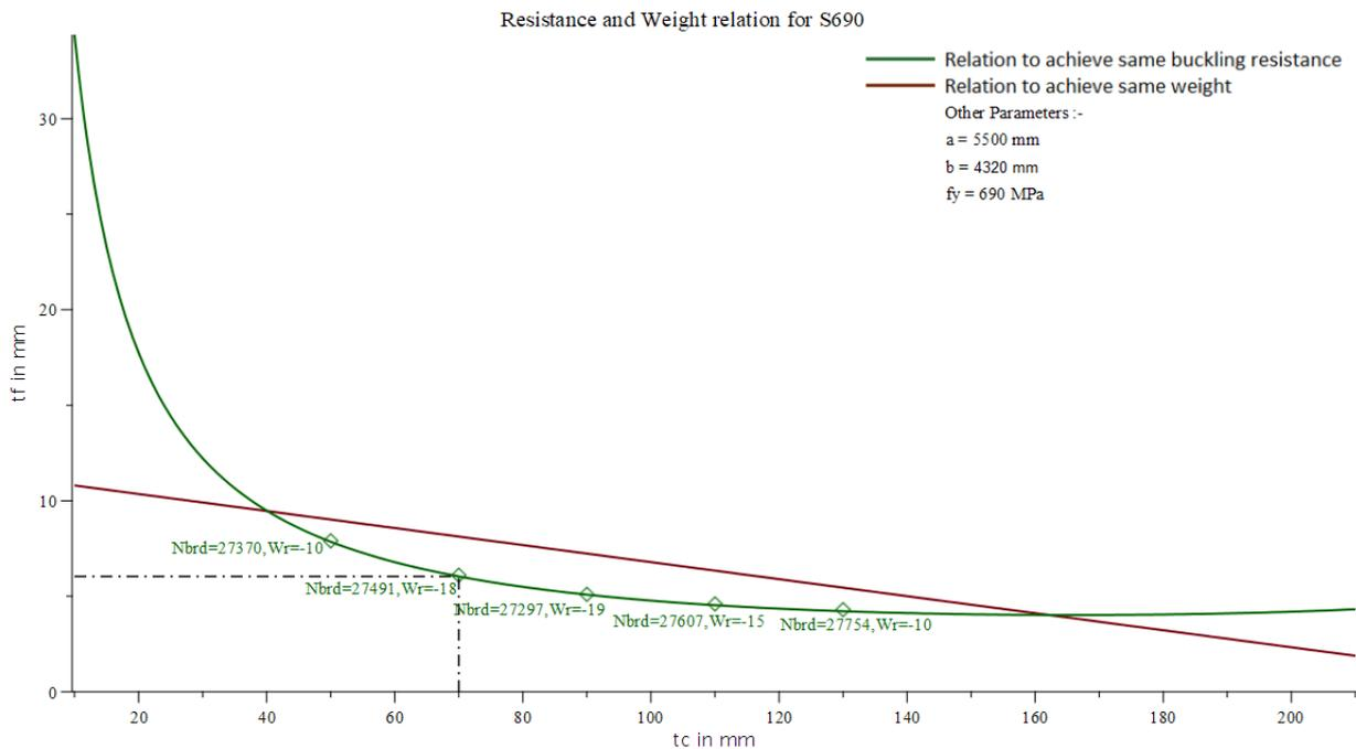
Figure G.5 Relation between the thickness of faceplate and core for buckling resistance and weight
