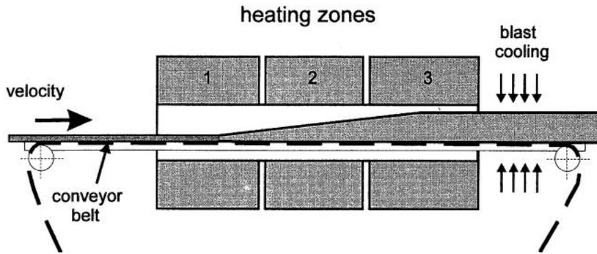
Figure 2.9 Schematic principle of continuous belt furnace for foaming of the core layer [36]
