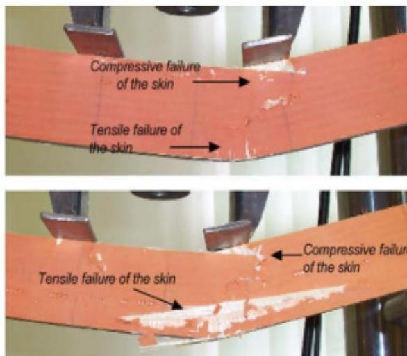
A. Compressive and tensile facing failure in edgewise bending.
