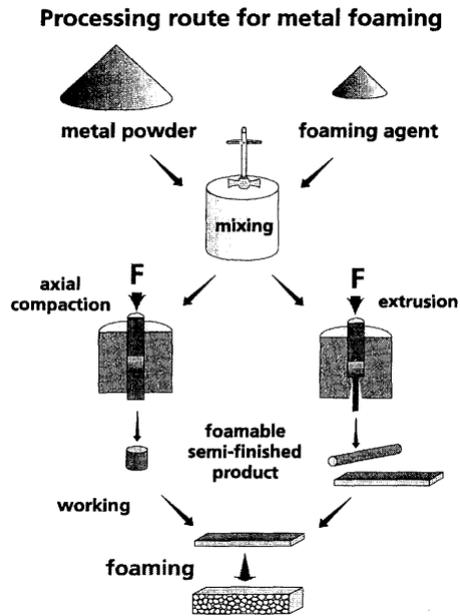
Figure 2.7 Production of metal foams (powder metallurgical IFAM-Process) [16]
