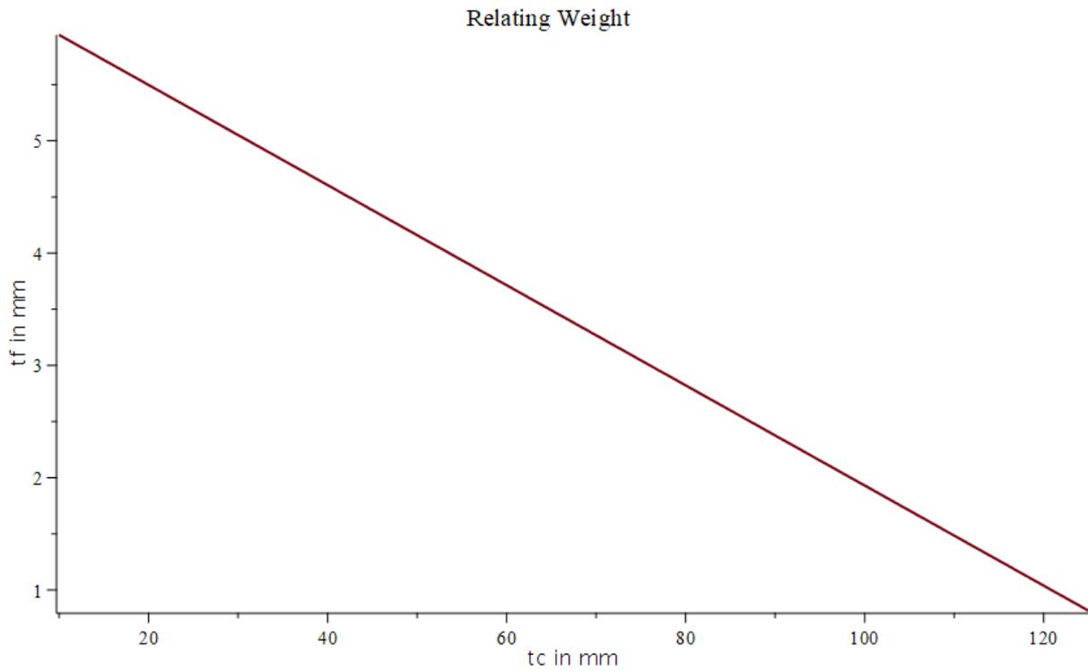
Figure 4.10 Relation between the thickness of the core and faceplate to achieve the same weight as that of stiffened plate
