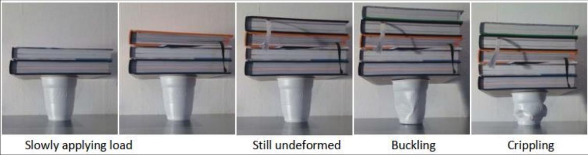
Figure 2.18 Simple example of shell buckling [10]
