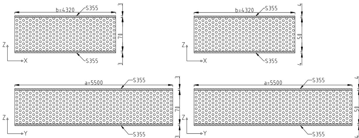
Figure 4.7 Sandwich Panel with arbitrary configuration 3-70-3 and 4-50-4
