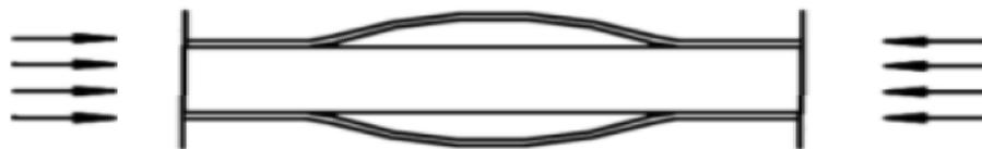
Figure 4.6 Face wrinkling of a sandwich panel under compressive loading [15]
