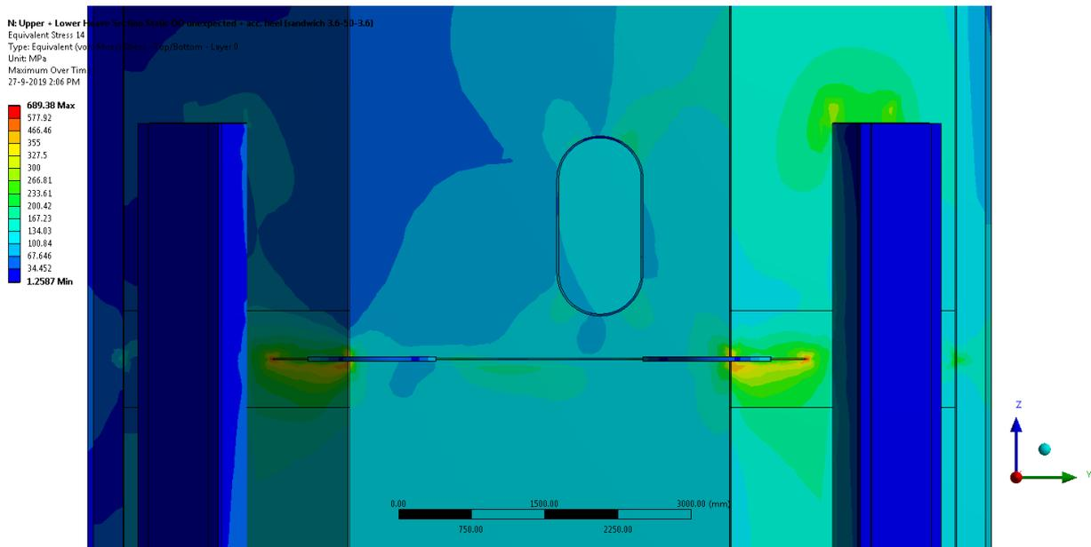
Figure 6.15 Von Mises stresses at joints
