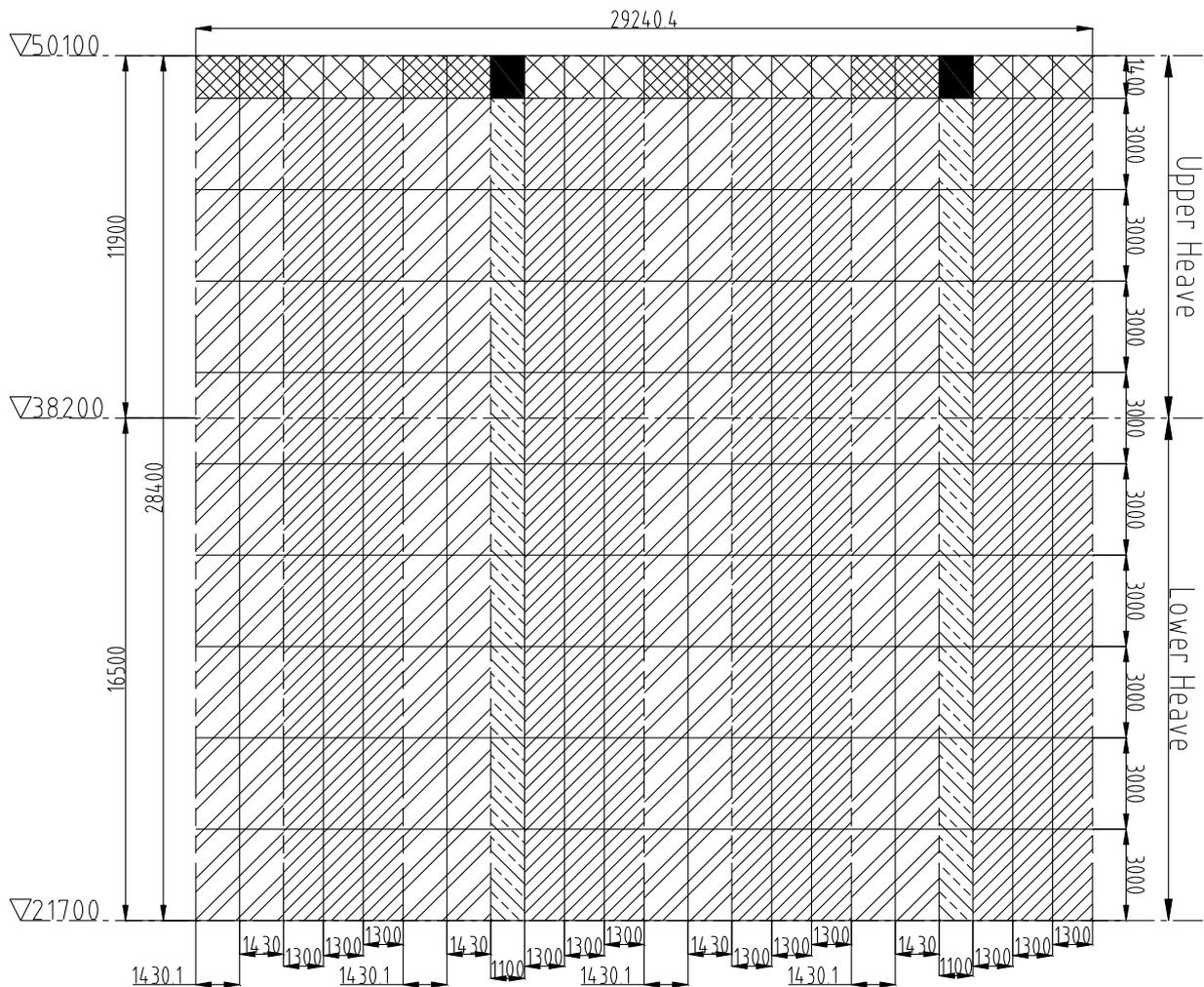
Figure 6.30 Heave section with sandwich panel
