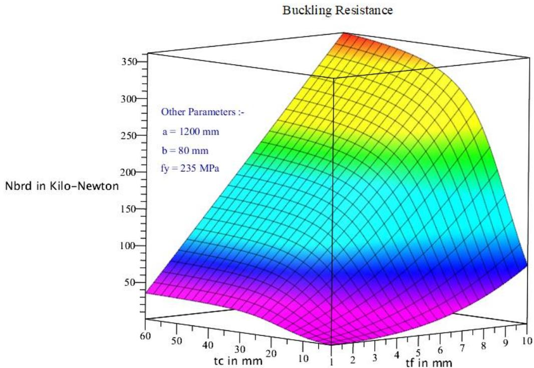
Figure 3.14 Effect of thickness of faceplate and core on the buckling load
