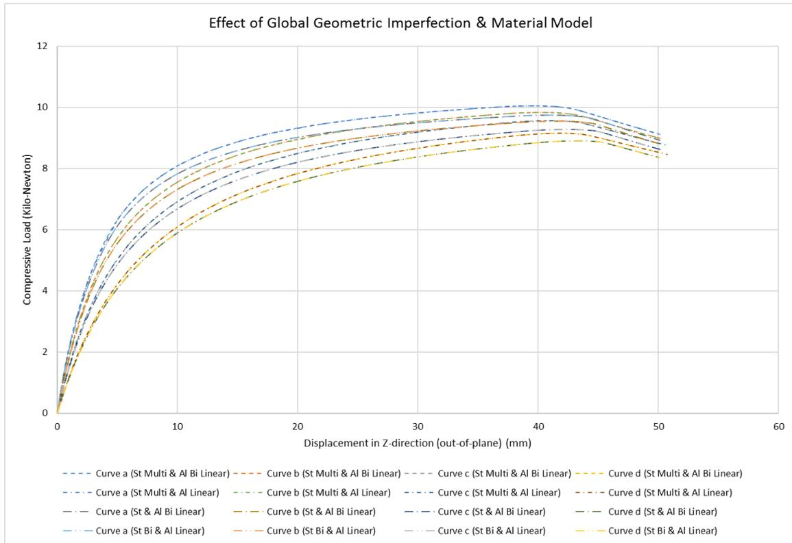
Figure 3.10 Graph between Out-plane displacement vs Compressive Load (Global Imperfection)
