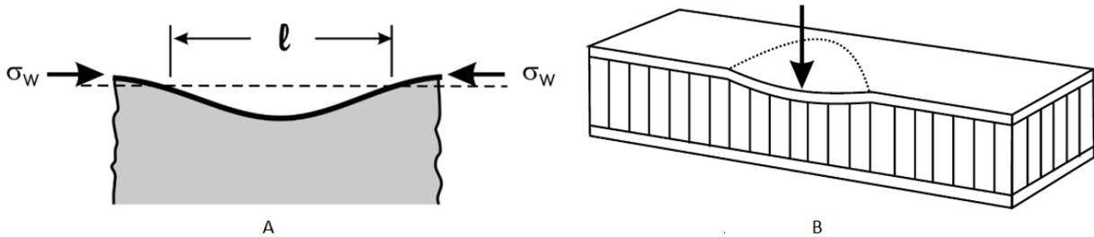
Figure 2.2 A) Wrinkling of face sheets loaded in compression B) Local indentation failure due to concentrated load [8]
