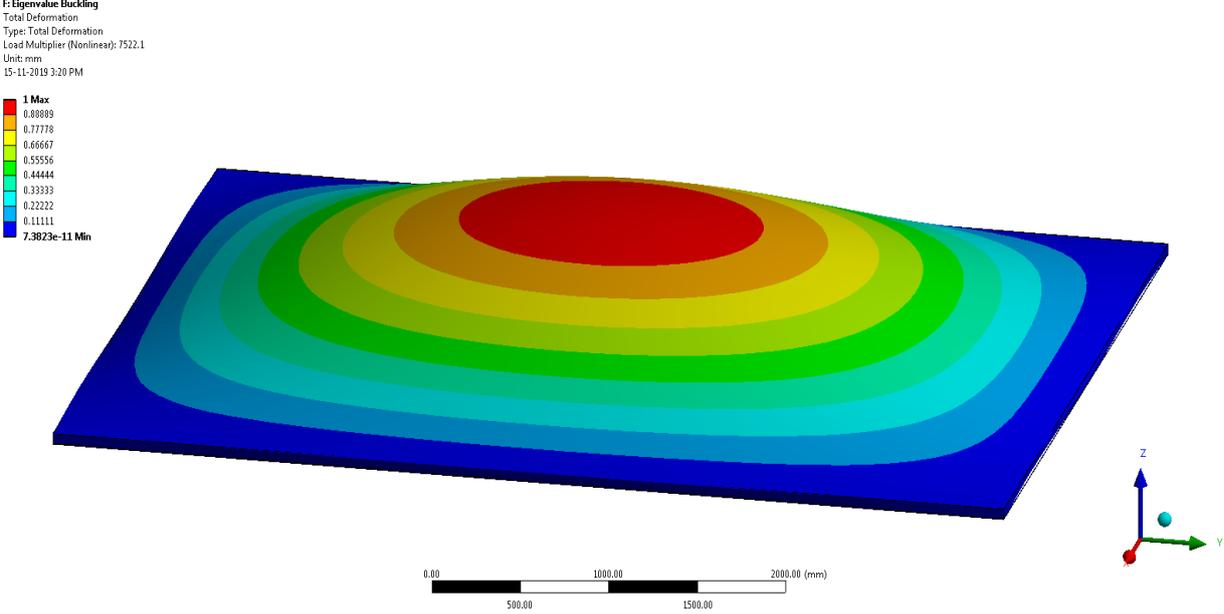
Figure D.14 First Eigen buckling load calculated with ANSYS
