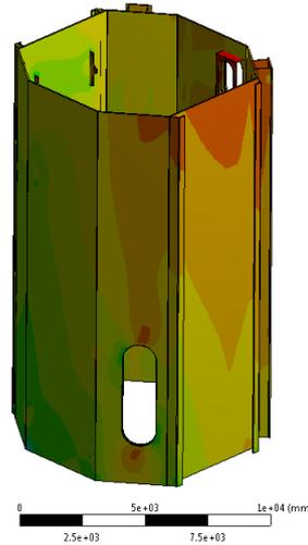
Figure 6.10 Minimum principle stress (lower part)
