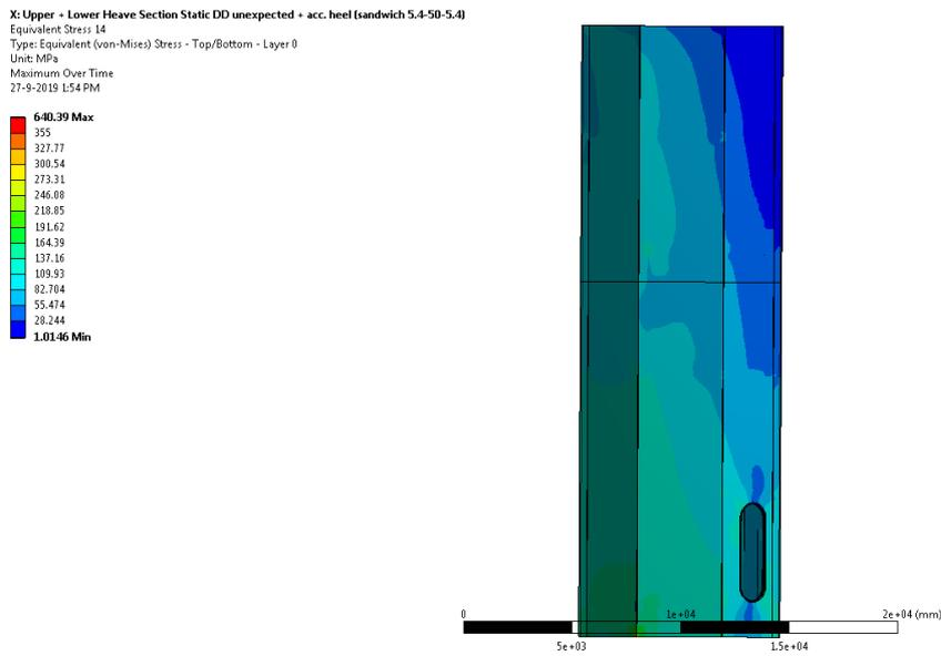
Figure 6.5 Von Mises stress (back view)
