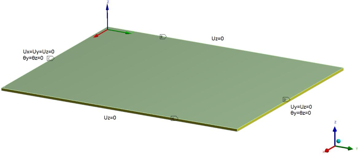
Figure D.4 Boundary conditions of sandwich panel
