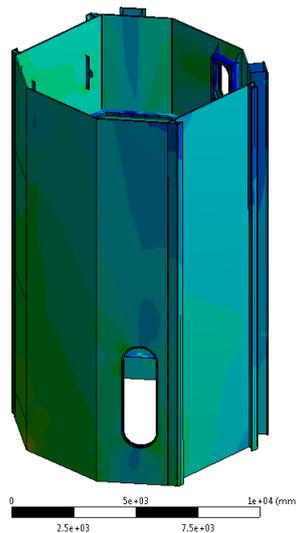
Figure 6.19 Minimum principle stress (lower part)
