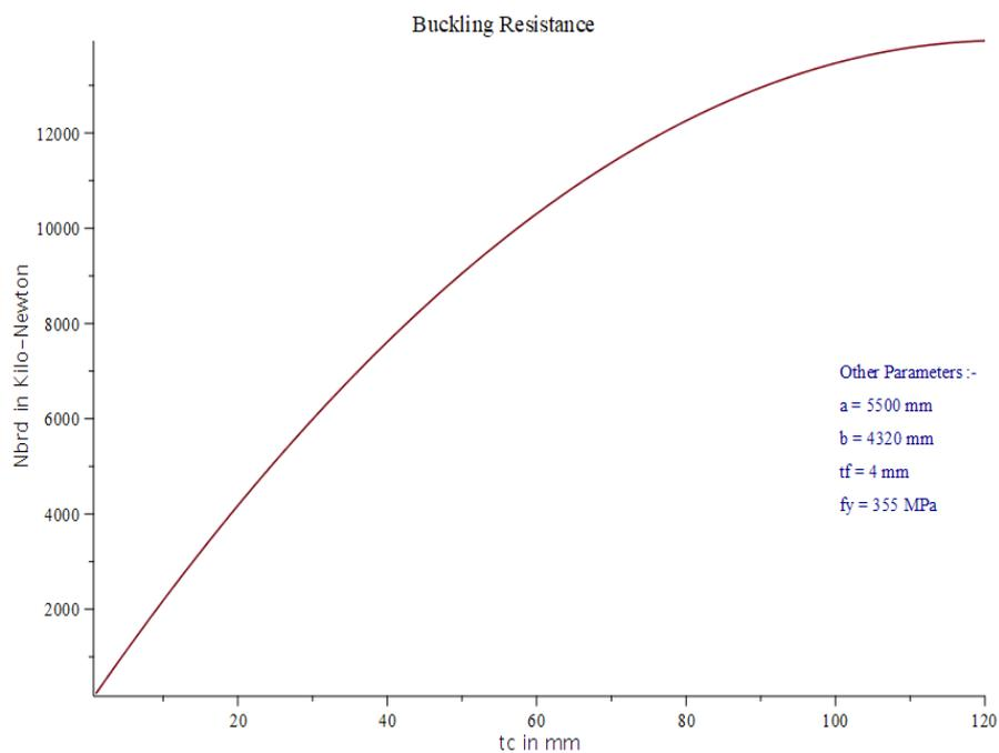
Figure 5.2 Effect of thickness of core on the buckling load
