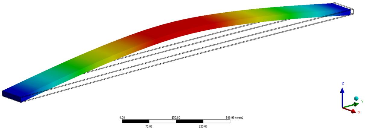
Figure 3.9 Out-of-plane displacement of sandwich panel
