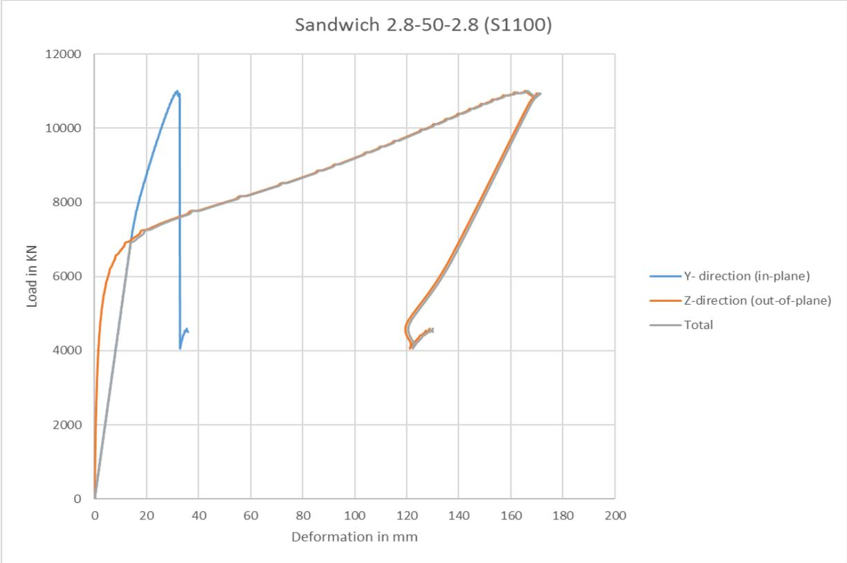
Figure D.16 Nonlinear Buckling Analysis of Sandwich S1100
