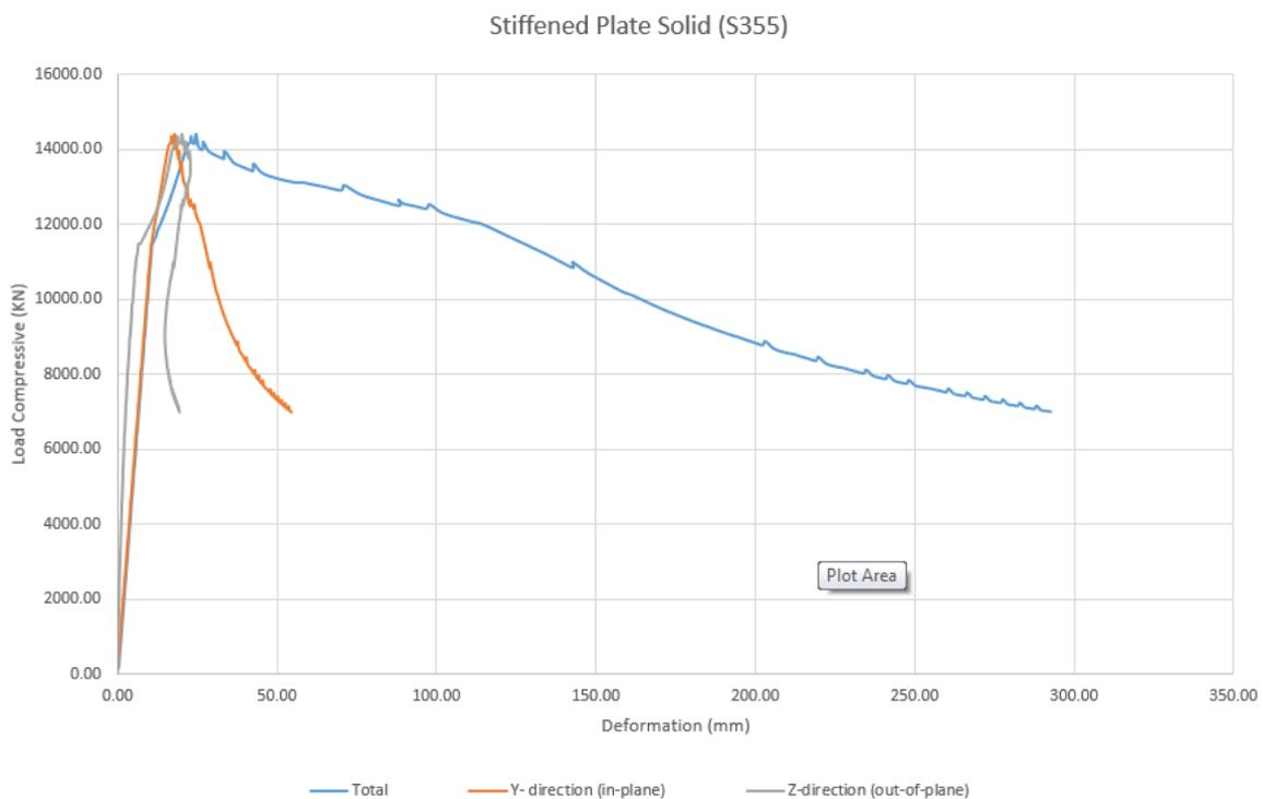
Figure B.8 Nonlinear Buckling Analysis of Stiffened Plate S355
