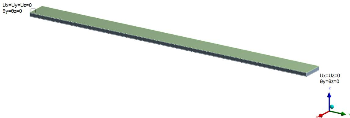
Figure A.4 Boundary conditions of sandwich panel
