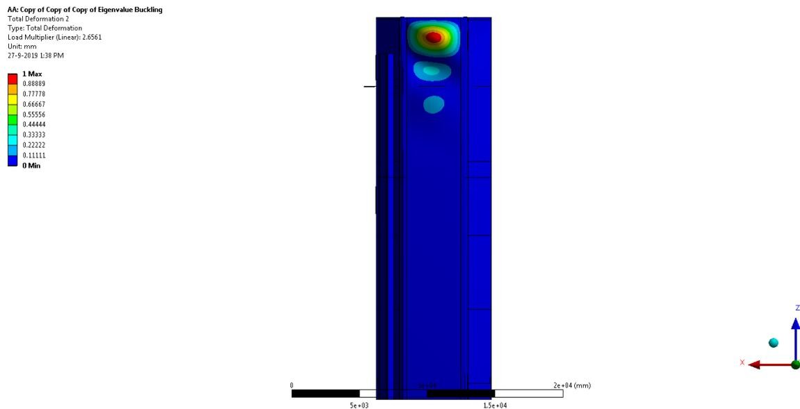
Figure 6.20 Buckling of heave section
