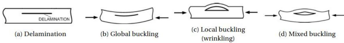
Figure 2.14 Delamination and possible subsequent buckling failure modes [47]
