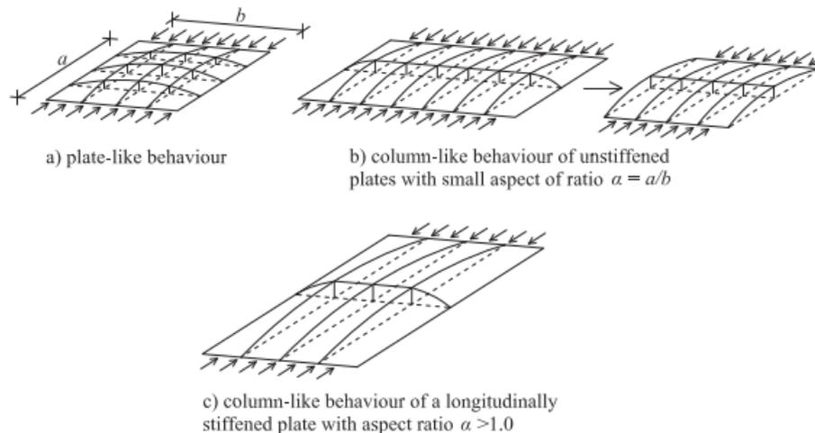
Figure 2.20 Plate-like and column-like buckling of the plate in compression [11]
