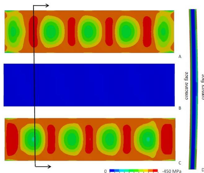
Figure 2.5 In-plane stress distribution in a panel: A. top face (steel plate), B. mid-plane (foam plate), C. top face (steel plate), D. cross-section (top steel - steel foam - bottom steel face) [5]
