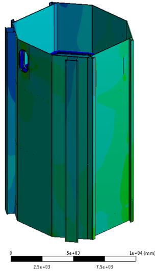
Figure 6.18 Minimum principle stress (lower part)
