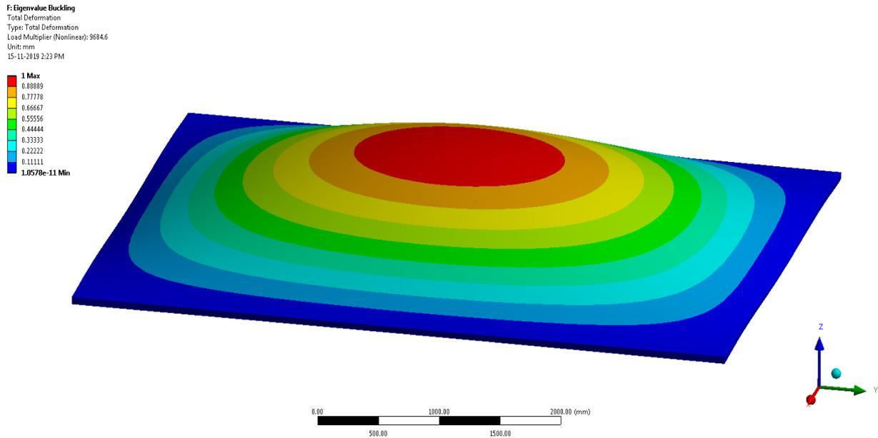
Figure D.6 First Eigen buckling load calculated with ANSYS
