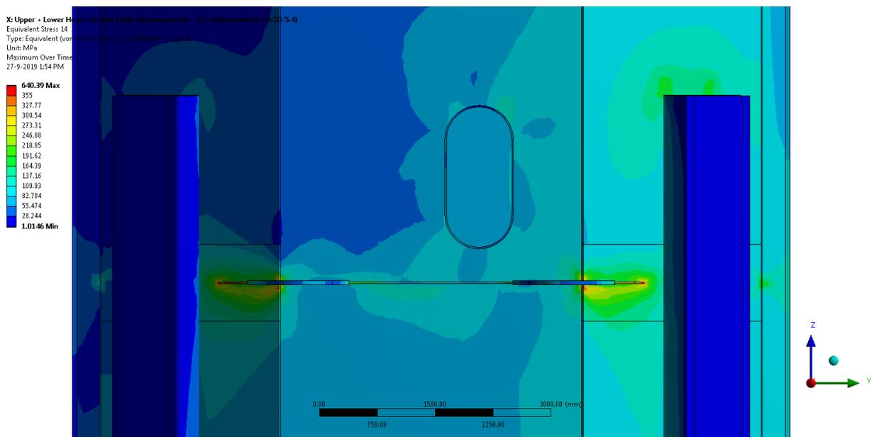
Figure 6.6 Von Mises stresses at joints
