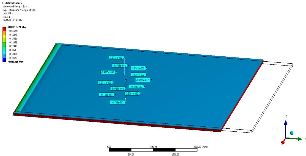
Figure D.15 Minimum principle stress calculated with ANSYS
