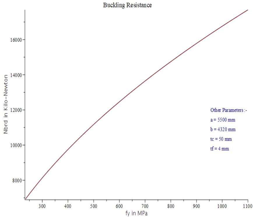
Figure 5.3 Effect of yield on the buckling load
