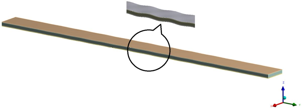
Figure A.7 Model of sandwich panel with local geometric imperfection
