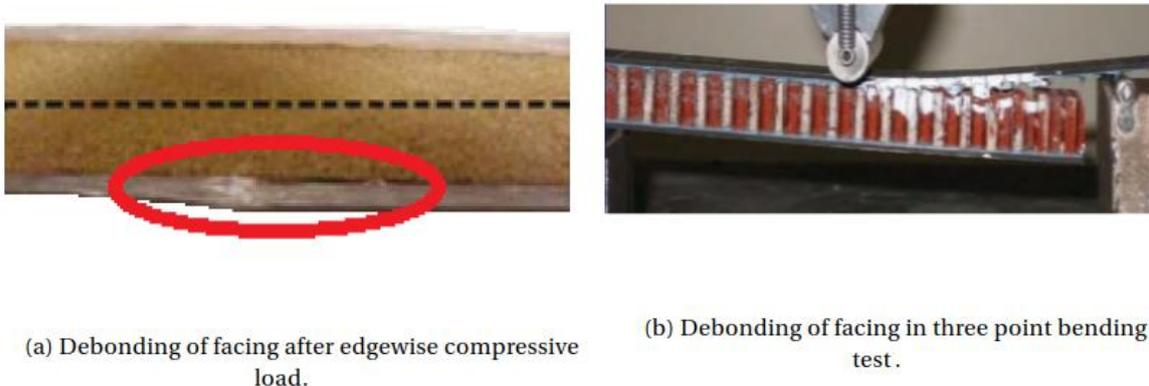
Figure 2.12 Face-core debonding under three-point bending and edgewise compressive load [44]
