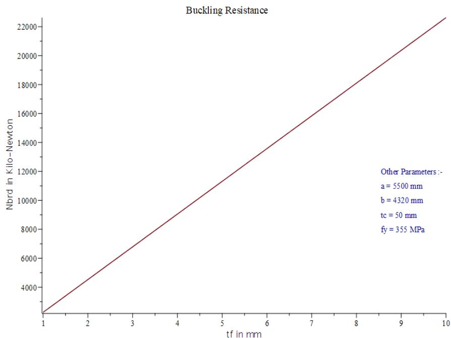
Figure 5.1 Effect of thickness of faceplate on the buckling load
