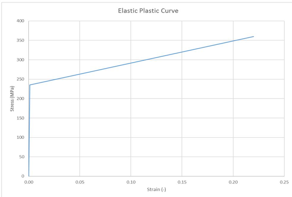
Figure 3.3 Steel material model Bi-linear
