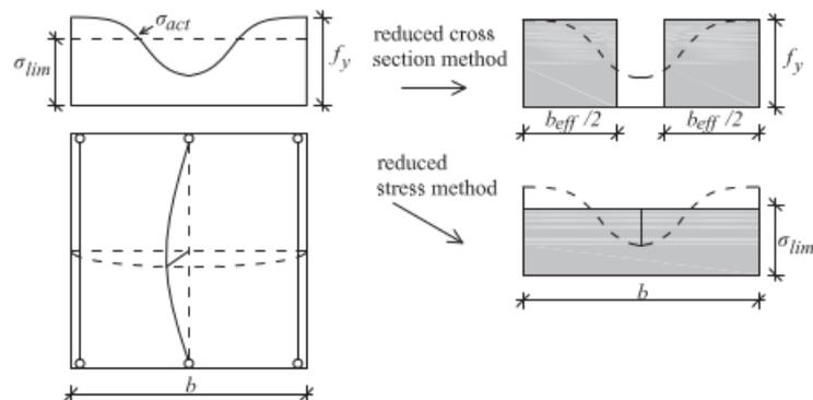
Figure 2.22 Basic idea of reduced stress method and reduced cross-section method [11]
