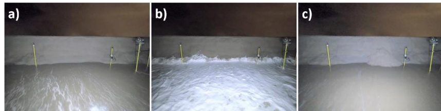
Fig. 3. Dune face during the December storm before (a), during (b) and after (c) wave impact causing a slump to slide down the dune face
