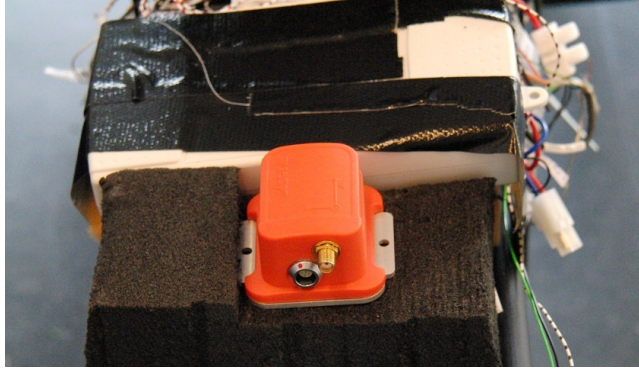
Figure 6.7: The Xsens MTI-g orientation sensor on the location where it was connected to the measurement bicycle. The sensor was fixed rigidly to bicycle frame using duct tape with the foam material from the picture between the frame and the sensor. The purpose of the foam material is to provide some damping for the vibrations caused by the road's surface.
