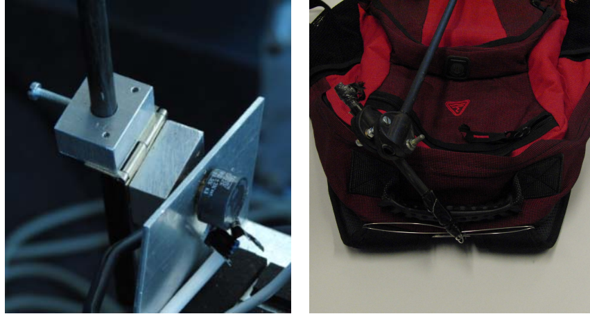
(a) The potentiometer which is used in order to measure the body movement of the rider, the arm that is also connected to the backpack is also shown. (b) The arm connected to the backpack. The arm is connected to the backpack as rigidly as possible using iron wire. Figure 6.1 shows an overview of this system.
