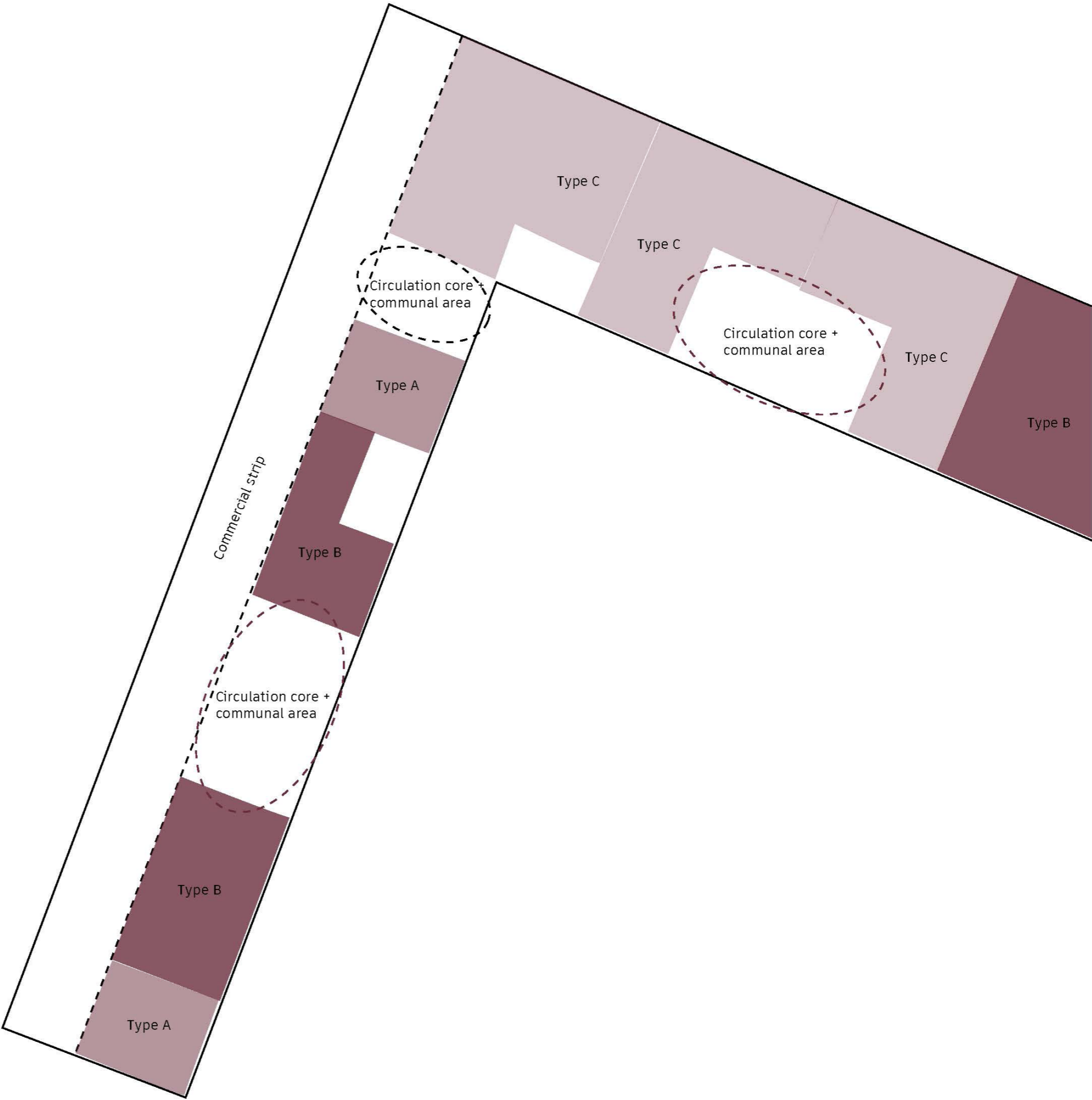
Fig. 89. Possible alternation of apartment types on the groundfloor of the family housing building (author's work, 2026)
