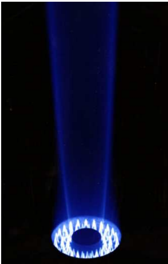
Figure 3.1: Close up of Sandia flame [2]
