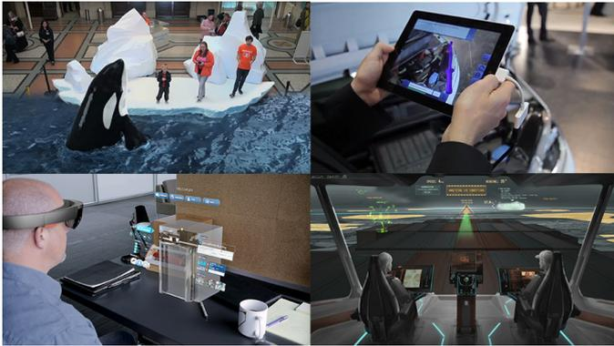
**Figure 57:** Different AR hardware platforms. Clockwise from top left: stationary AR [Industry, 2013], handheld AR [Vroegop, 2013], heads-up display [Lavrinc, 2014], wearable AR [Erickson, 2016].
