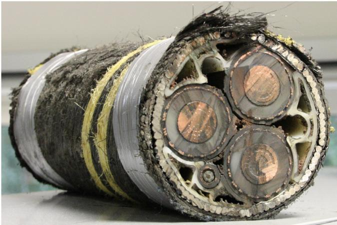
**Figure 4:** Subsea power export cable with  $D = 0.155\text{m}$ .
