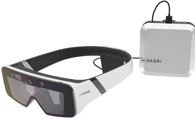
**Figure 55:** State-of-the-art wearable AR device: *Daqri Smart Glasses* [DAQRI, 2017].
