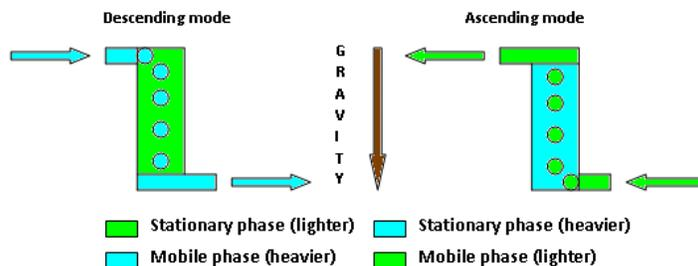
**Figure 2.9: Counter-current chromatography scheme**
