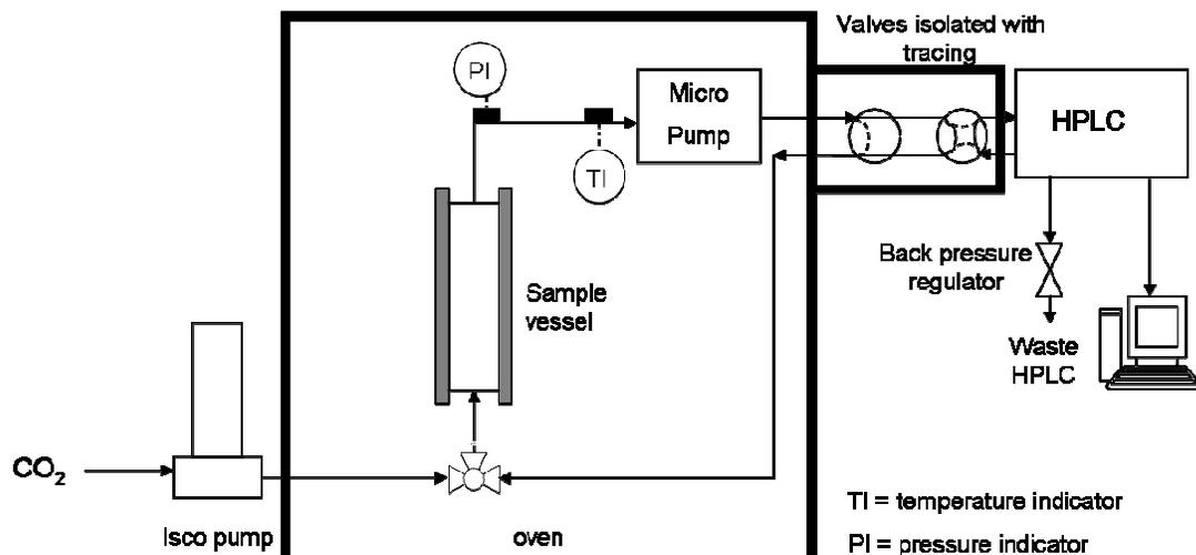
**Figure 4.2: Schematic drawing of the solubility cell**
