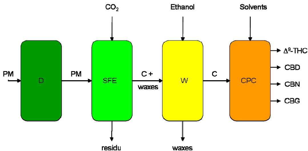
PM = Plant Material - D = Decarboxylation - SFE = Supercritical Fluid Extraction
