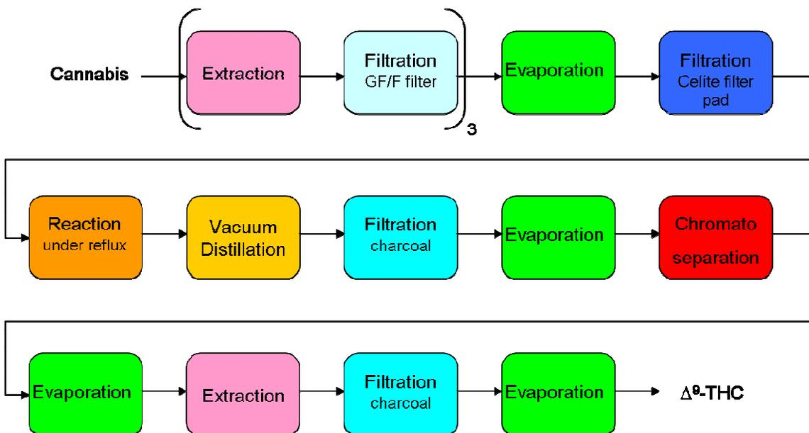
**Figure 9.4: Flow diagram of the  $\Delta^9$ -THC Production according to patent US 2009 / 133376**
