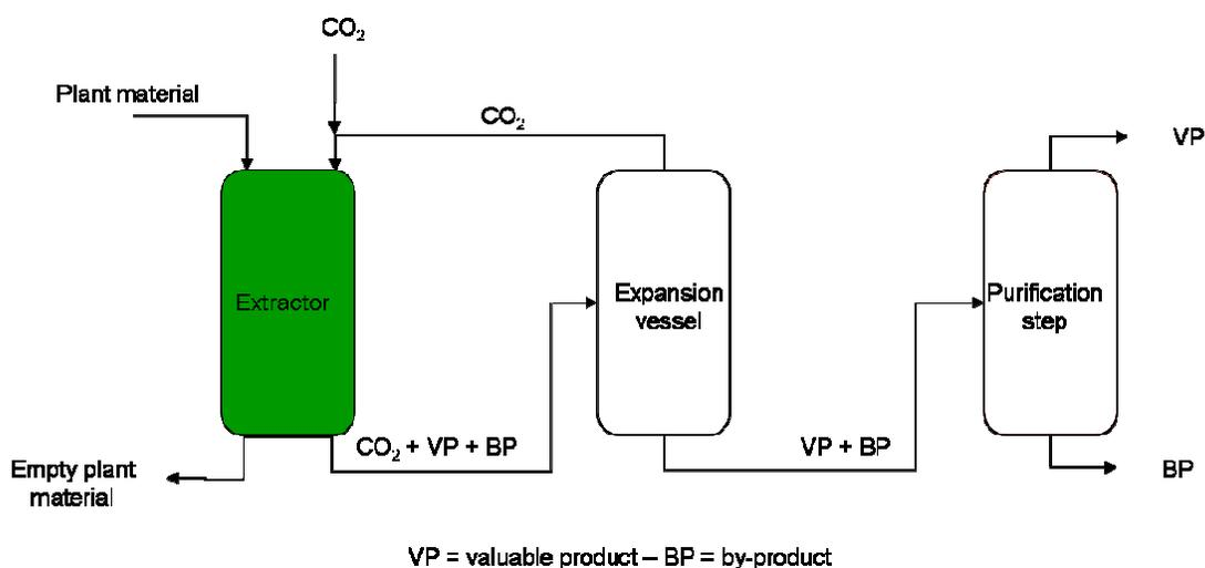
**Figure 1.2 Schematic drawing of supercritical fluid extraction equipment**
