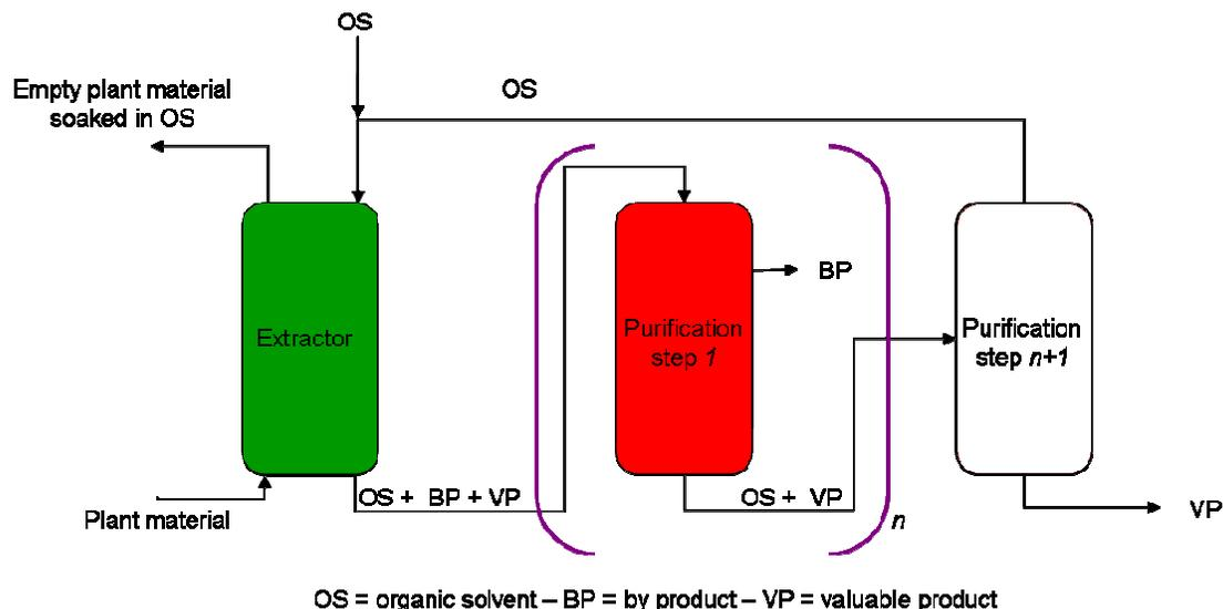
**Figure 1.1 Schematic drawing of an extraction process with organic solvents**
