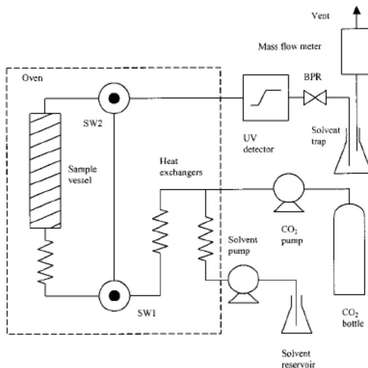
**Figure 2.4: Apparatus for the determination of solubility using a dynamic method.**
