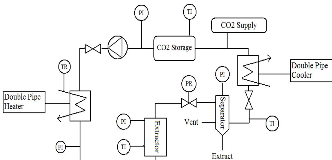
**Figure 2.5: Schematic drawing of typical SFE set-up - PI = Pressure Indicator, TI = temperature Indicator, PR = Pressure regulator, FI = Flow Indicator, TR = Temperature Regulator**
