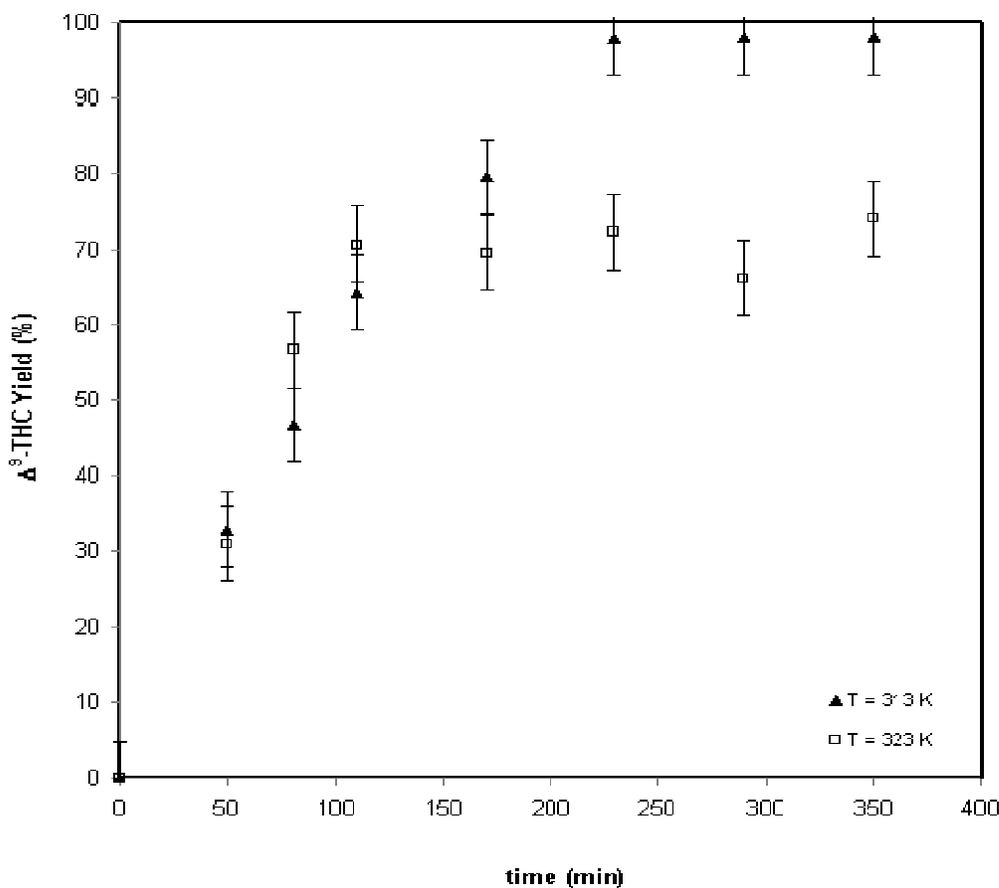
Figure 7.6:  $\Delta^9$ -THC yield as a function of time at 18 MPa
