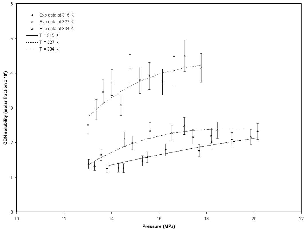
**Figure 5.2. CBN solubility in SC CO<sub>2</sub>: experimental results (points) and results from modeling with PR EoS (lines)**
