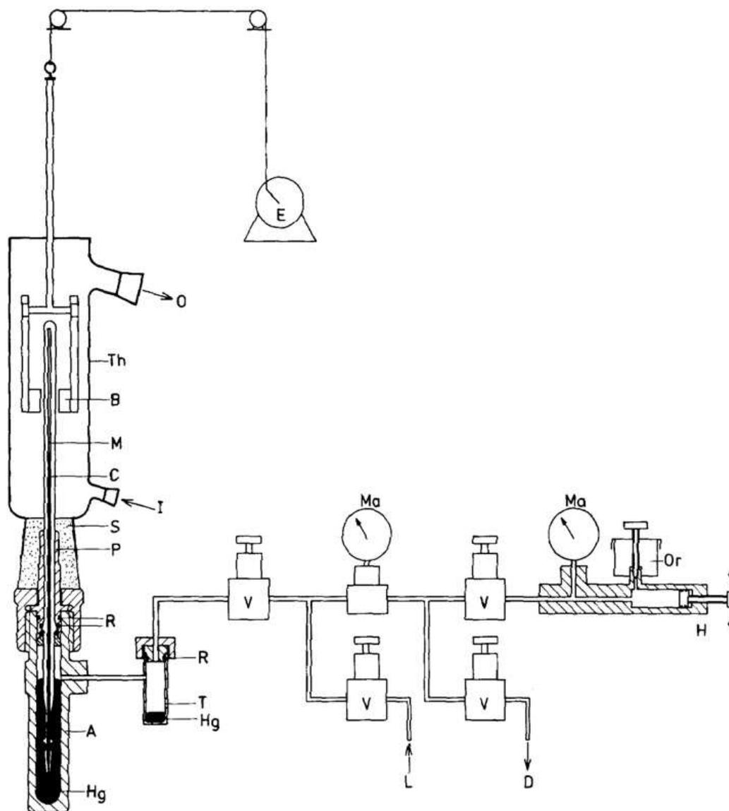
**Figure 2.3: Cailletet apparatus; A, autoclave; B, magnets; C, capillary glass tube; D, drain; E, motor; H, rotating hand pump; Hg, mercury; I, thermostat liquid in; L, line to dead weight pressure gauge; M, mixture being investigated; Ma, manometers; O, thermostat liquid out; Or, hydraulic oil reservoir; P, closing plug; R, Viton-O-rings; S, silicone rubber stopper; T, mercury trap; Th, glass thermostat; V, valve. [14].**
