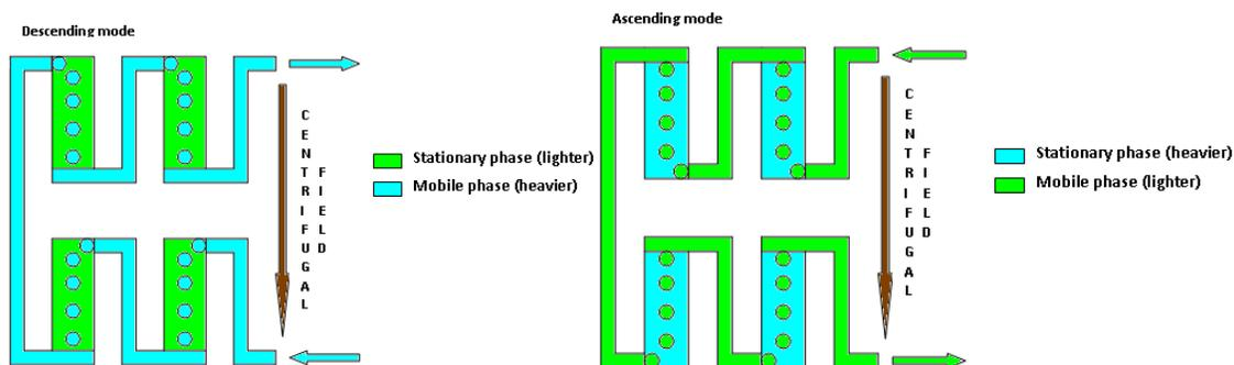
**Figure 2.10: Centrifugal partition chromatography scheme.**
