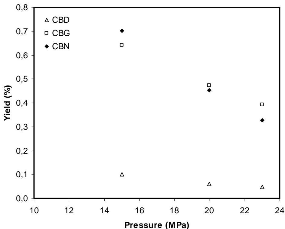
**Figure 7.9: Cannabinoids yields as a function of pressure at 313 K**
