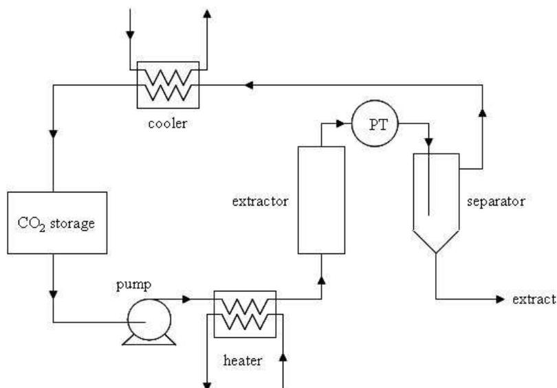
**Figure 7.2: Schematic overview of the experimental set-up for the supercritical extraction of cannabis**
