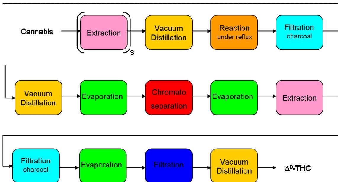
**Figure 9.3: Flow diagram for the  $\Delta^9$ -THC Production according to patent US 2005 / 0171361**
