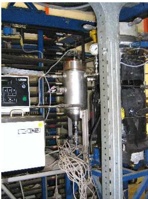
**Figure 2.7: Separator of the SFE set-up**
