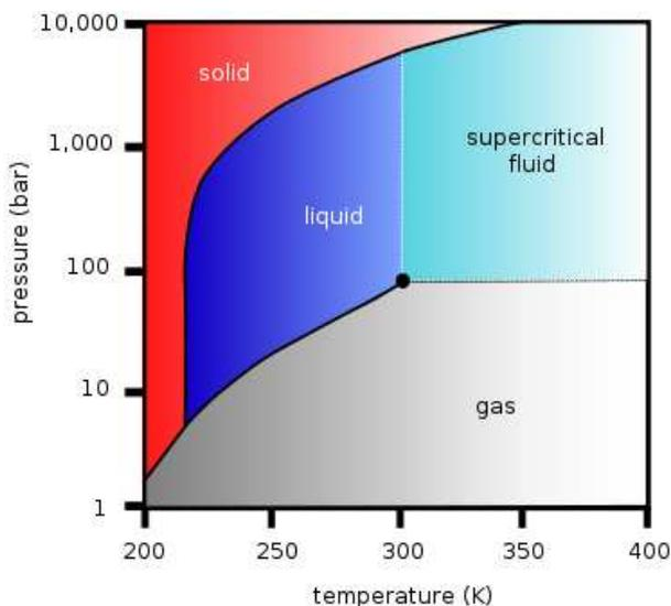
**Figure 2.1: Phase diagram of carbon dioxide**
