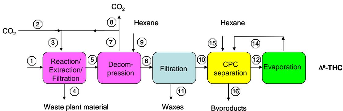
**Figure 9.3: Block diagram of the alternative process**
