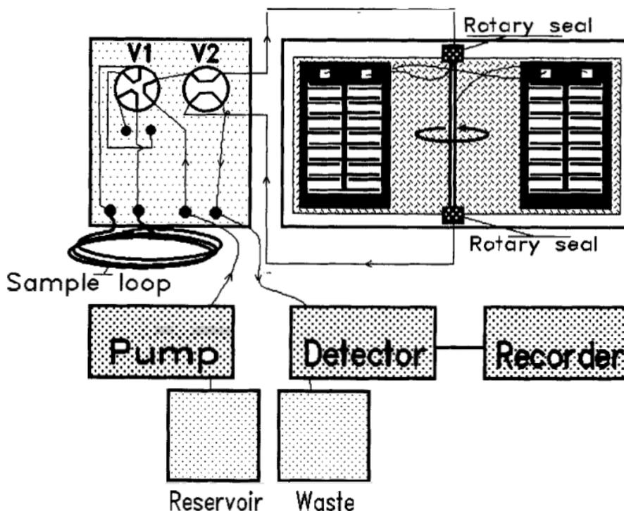
**Figure 8.1: the general set-up in the descending mode. V1 = infection valve - V2 = switching valve (ascending or descending mode) [4]**
