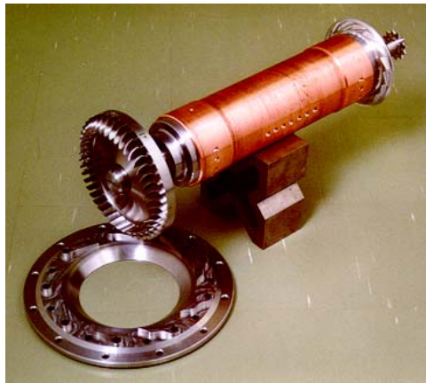
Figure 1.1: Photograph of the high-temperature low capacity ORC turbogenerator rotor commercialized by a Dutch company. The purely radial expander wheel is visible on the left end of the generator shaft, and one half of the disassembled stator ring rests on the table top. Courtesy of Triogen [11].
