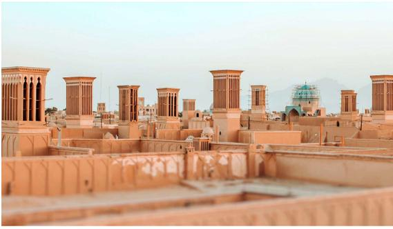
**Figure 3.2:** Bagdir or windcatcher, a traditional persian architectural element to create natural ventilation [26]
