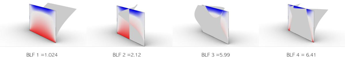
**Figure 7.10:** The first four buckling modes for the wall upper bound models unstabilised and cement stabilised
