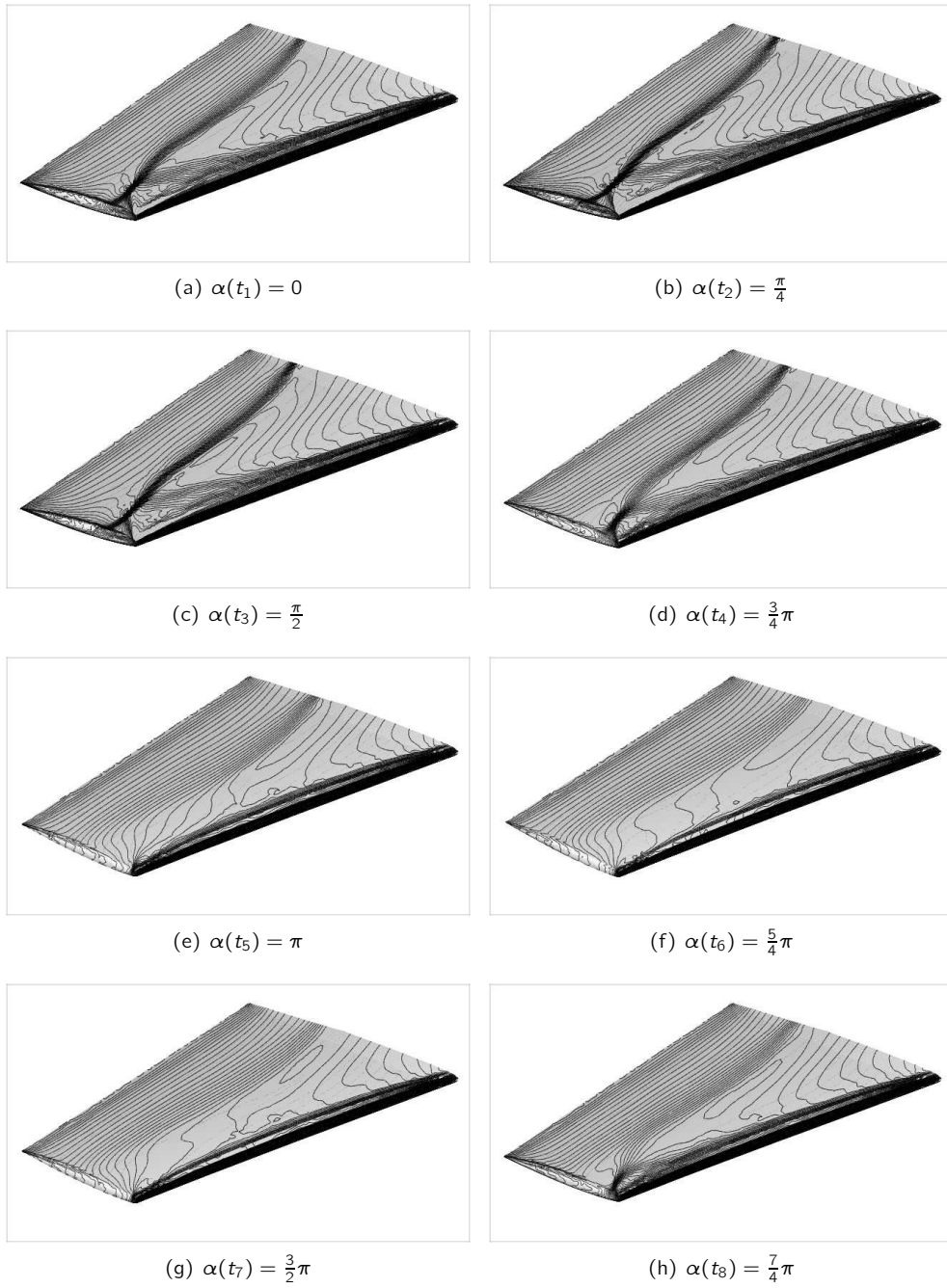
Figure A.3: Pressure contours on the ONERA-M6 wing in sinusoidal pitching motion at M_\infty = 0.8 and \alpha = 3.6^\circ .
