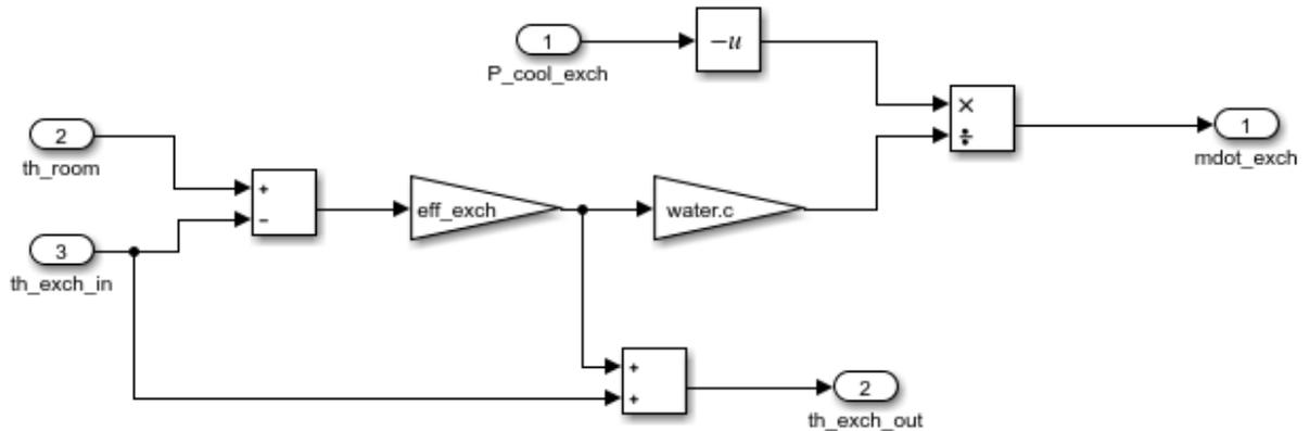
Figure B-8-11. Simulink blocks related to the heat exchanger.
