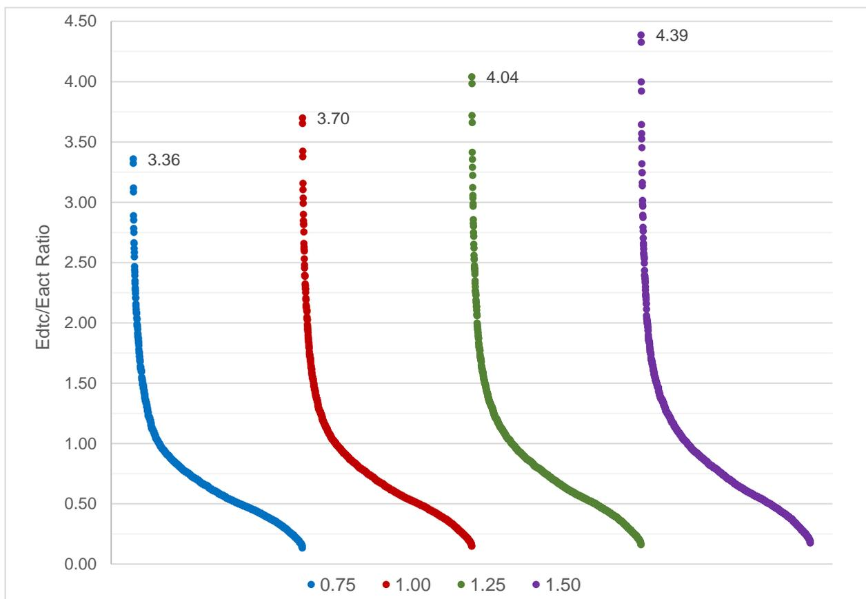
Figure 7-26. The  $E_{dtc}/E_{act}$  ratio of the simulations grouped by the value of the height of the water tank (m).
