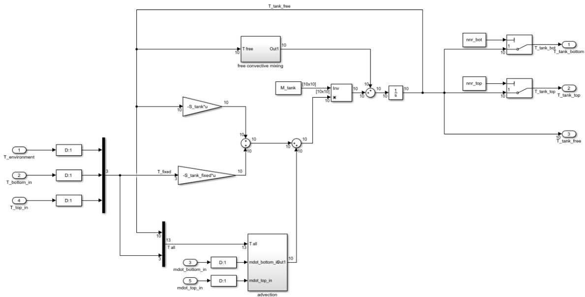
Figure B-8-12. Subsystem calculating the temperature at the top and bottom of the water tank
