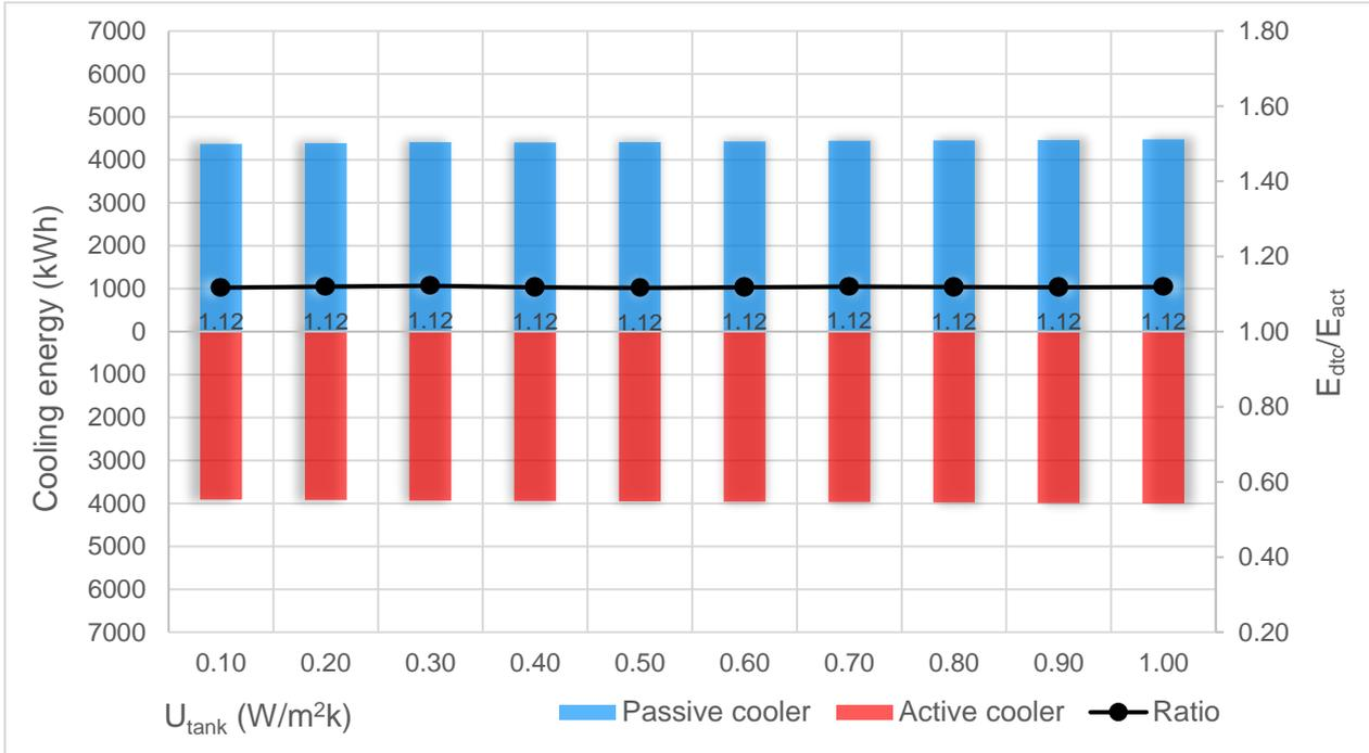
Figure 7-18. The sensitivity of the system to the U-value of the water storage tank.
