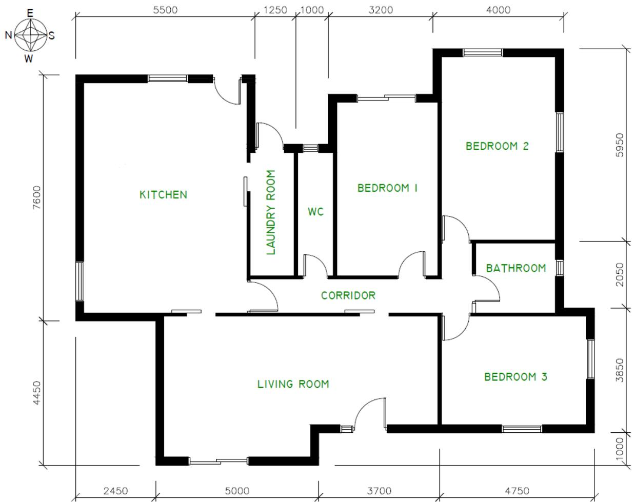
Figure 5-7. The conventional dwelling to be used as a case study (dimensions in mm).
