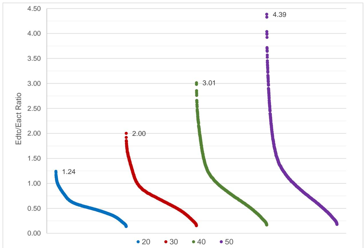
Figure 7-27. The  $E_{d_{tc}}/E_{act}$  ratio of the simulations grouped by the value of the surface of the passive cooler (% of the roof area).
