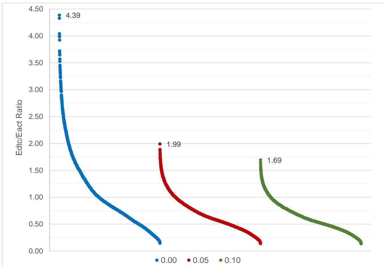
Figure 7-28. The  $E_{d_{tc}}/E_{a_{ct}}$  ratio of the simulations grouped by the value of the shortwave transmission coefficient.
