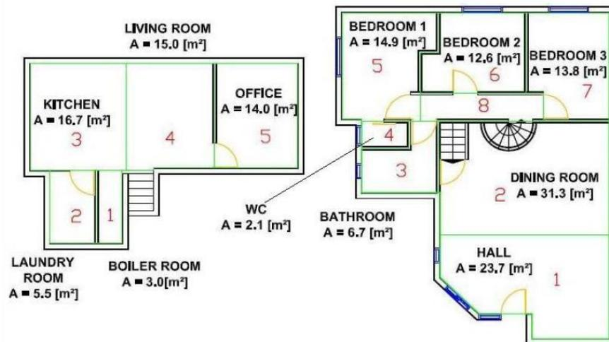
Figure 4-7. Floorplan of reference dwelling 2; detached building in Limassol, coastal zone (Panayiotou *et al*, 2010). Ground floor is on left side and first floor on the right side.
