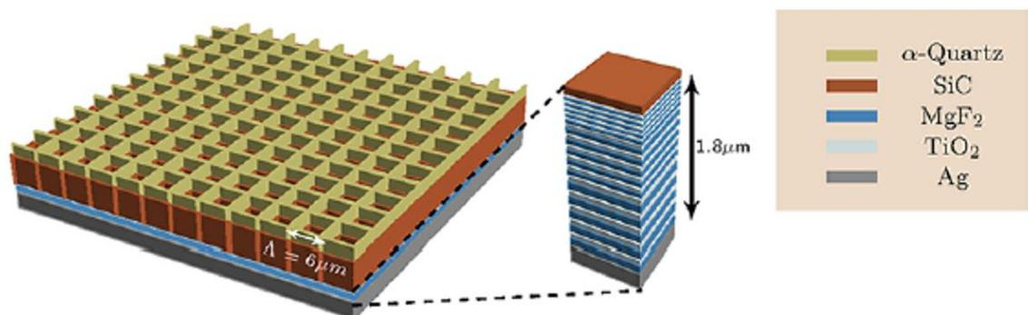
Figure 2-6. The metal-dielectric photonic structure presented by Rephaeli *et al.* (2013).
