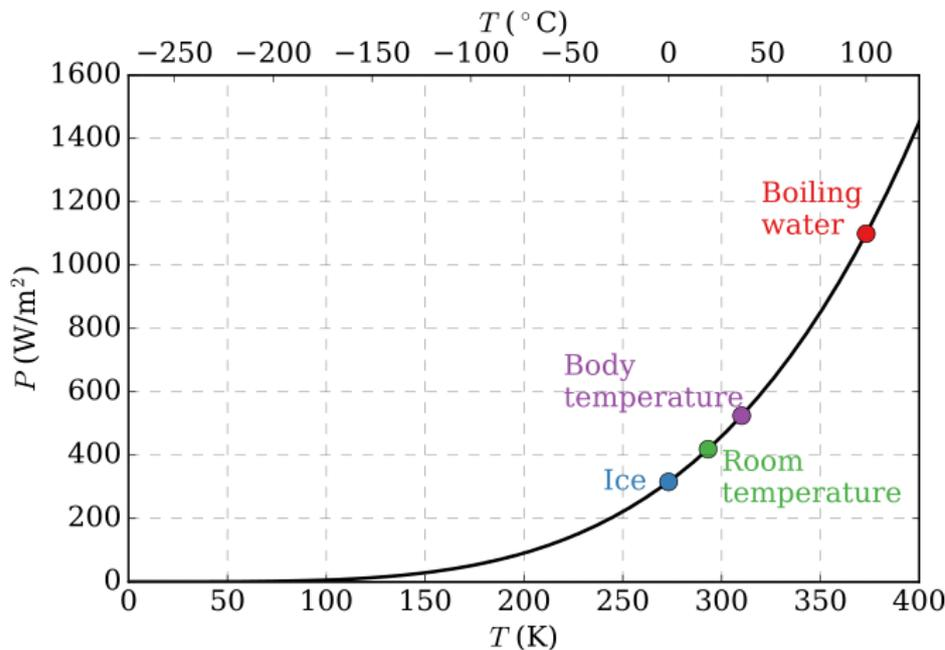
Figure 2-1. The radiative power emitted by a black body plotted against its temperature according to Steffan Boltzmann's law (Wikimedia Commons, 2016).
