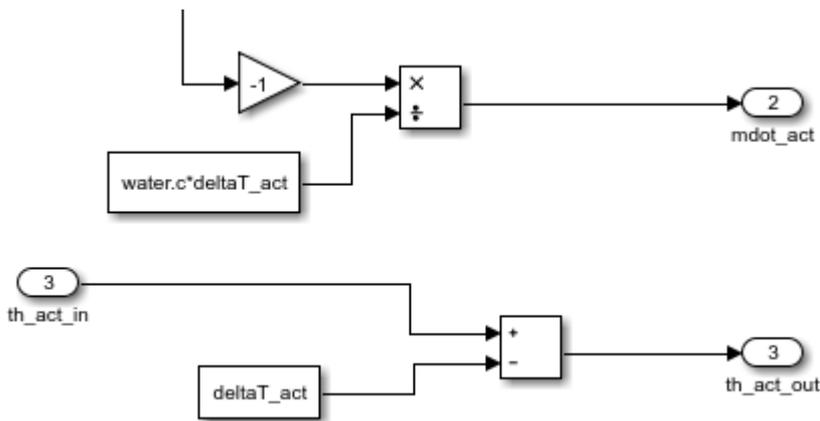
Figure B-8-9. Calculation of mass flow and outgoing water temperature of the active cooler.
