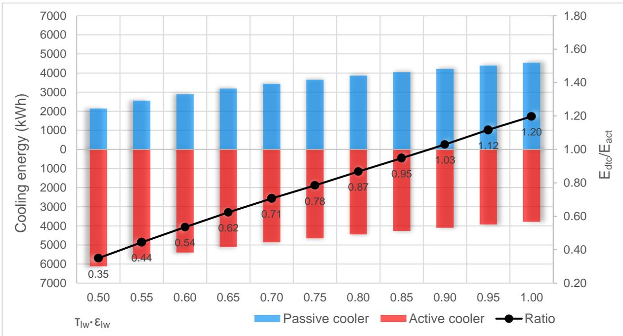
Figure 7-12. The sensitivity of the system to the product of the longwave transmission and emissivity coefficients
