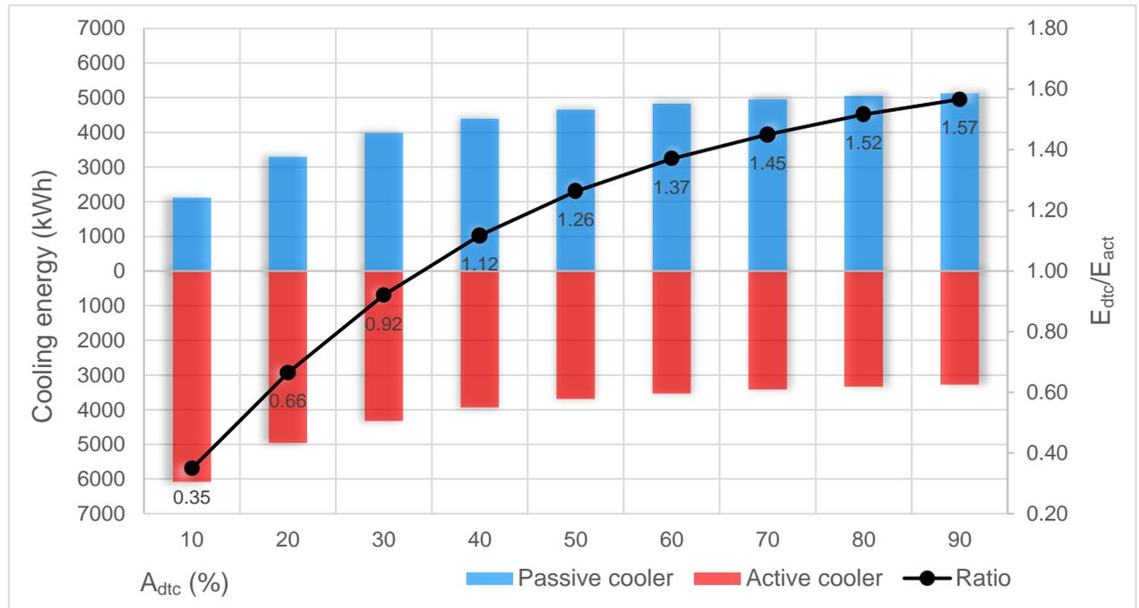
Figure 7-10. The sensitivity of the system to the area (as percentage of the roof area) of the radiative cooler.
