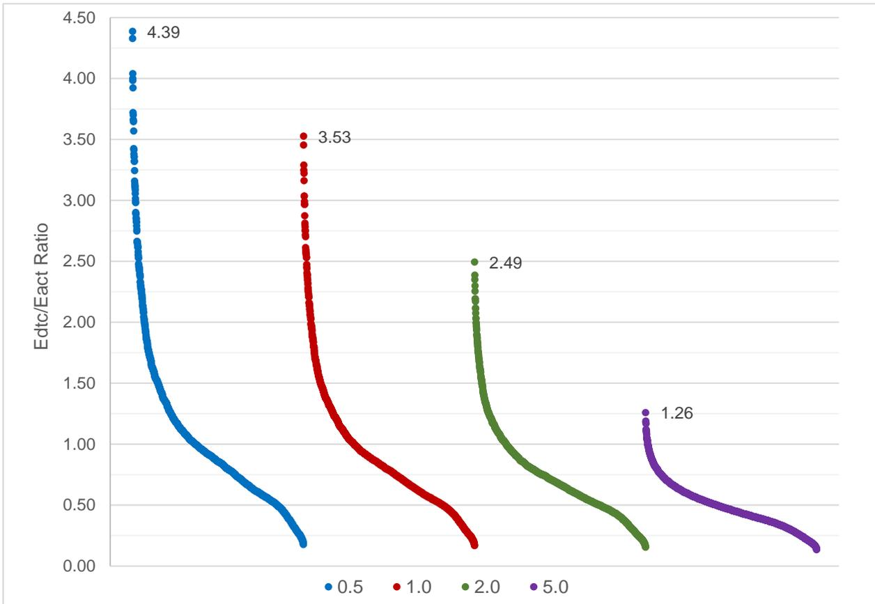
Figure 7-30. The  $E_{d_{tc}}/E_{act}$  ratio of the simulations grouped by the value of the effective heat transfer coefficient ( $W/m^2$ ).
