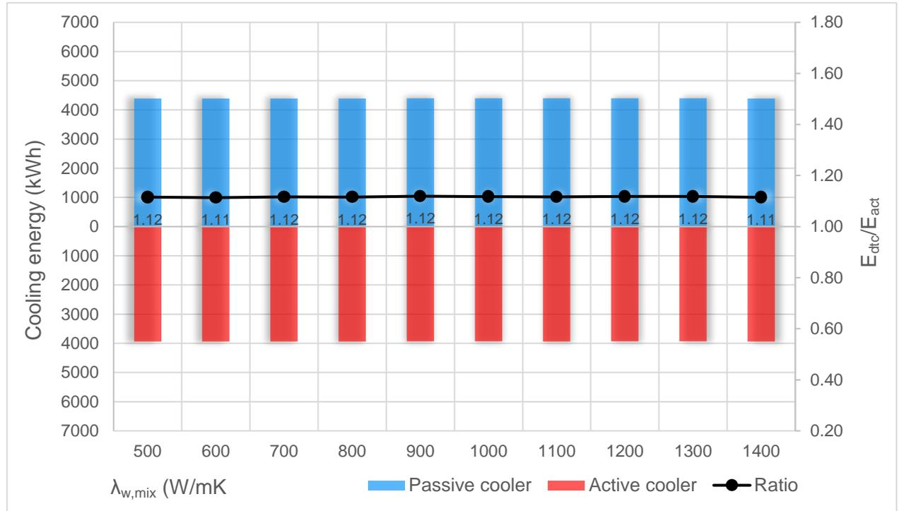
Figure 7-20. The sensitivity of the system to the effective free conduction coefficient for free convective mixing of water.
