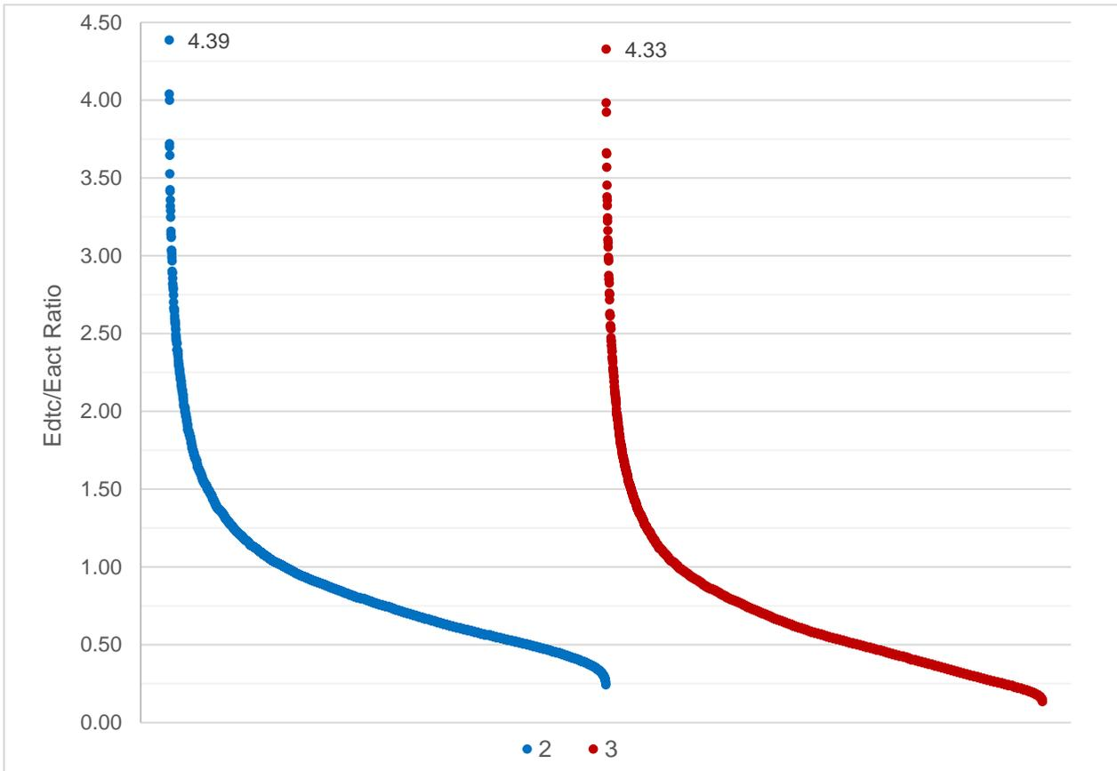
Figure 7-32. The Edtc/Eact ratio of the simulations grouped by the value of the minimum required temperature difference between the buffer tank and the daytime cooler (°C).
