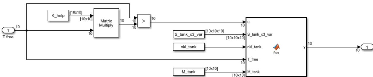
Figure B-8-14. Free convective flows subsystem of the water tank.
