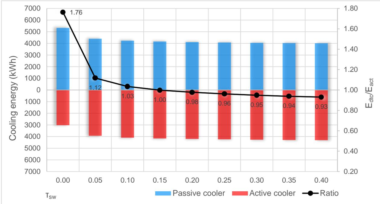
Figure 7-11. The sensitivity of the system to the shortwave transmission coefficient.
