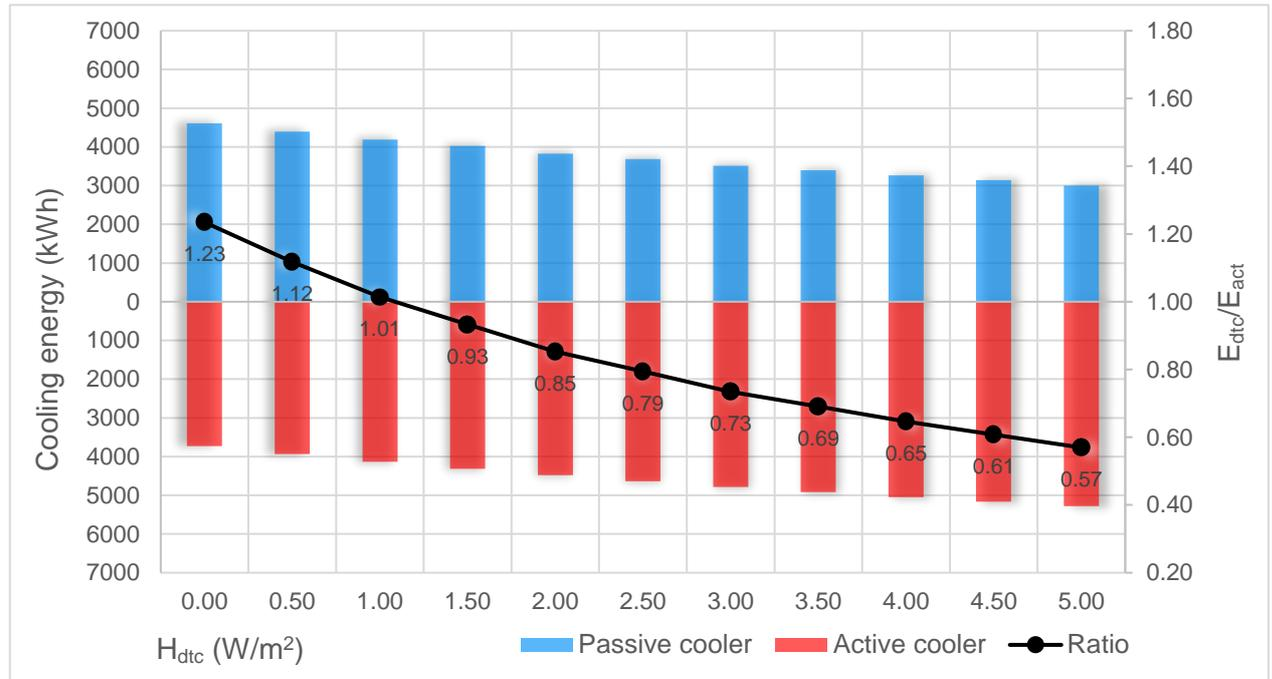
Figure 7-13. The sensitivity of the system to the effective heat transfer coefficient for values between 0 and  $5 \text{ W/m}^2$
