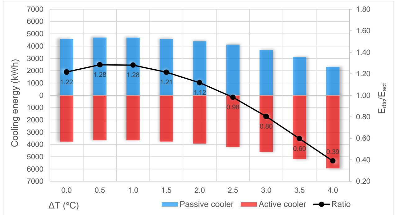
Figure 7-17. The sensitivity of the system to the minimum required temperature difference between the buffer tank and the passive cooler.
