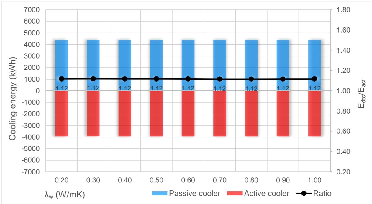
Figure 7-19. The sensitivity of the system to the heat conduction coefficient of water in the tank.
