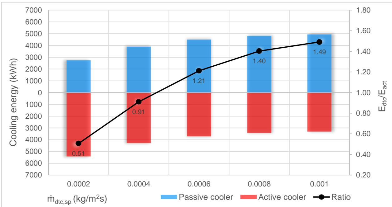
Figure 7-16. The sensitivity of the system to the mass flow rate of water within the passive cooler (< 0.001 kg/m<sup>2</sup>/s).
