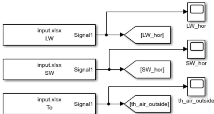
Figure B-8-1. Input of EnergyPlus hourly weather data from Excel file.
