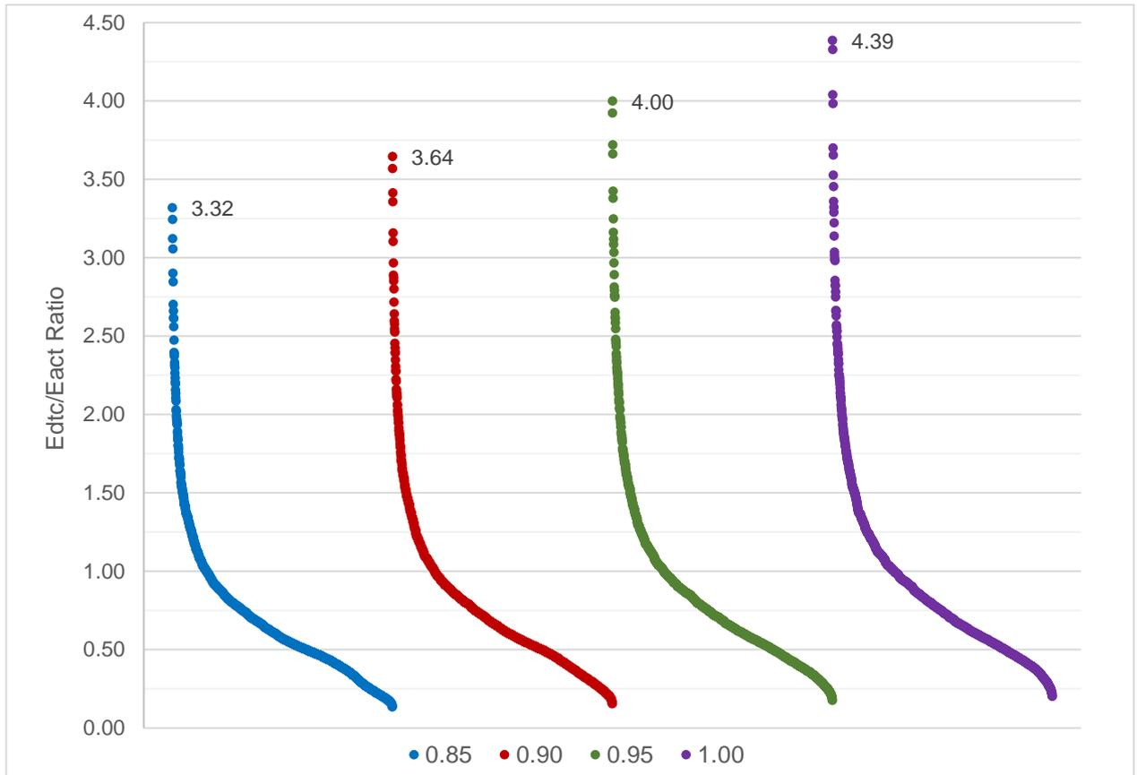
Figure 7-29. The  $E_{d_{tc}}/E_{act}$  ratio of the simulations grouped by the value of the product of the longwave radiation transmission coefficient and the longwave emissivity coefficient.
