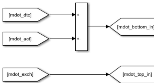
Figure B-8-3. Mass flow rates into the buffer tank.
