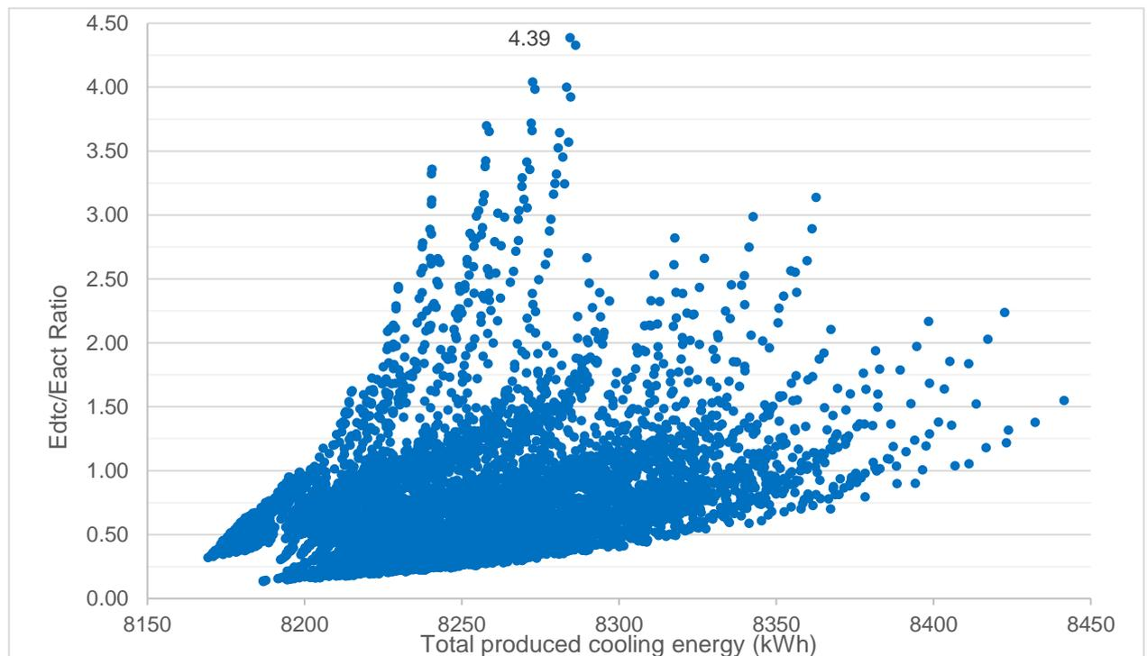
Figure 7-25. The ratio of the 6144 cases investigated plotted against the total cooling energy produced by the two coolers.
