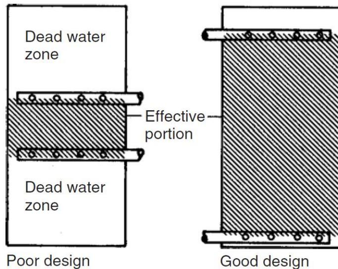
Figure 3-8. A poor and a good design of a water energy storage tank and the effective water portion in each case (Dincer and Rosen, 2011).
