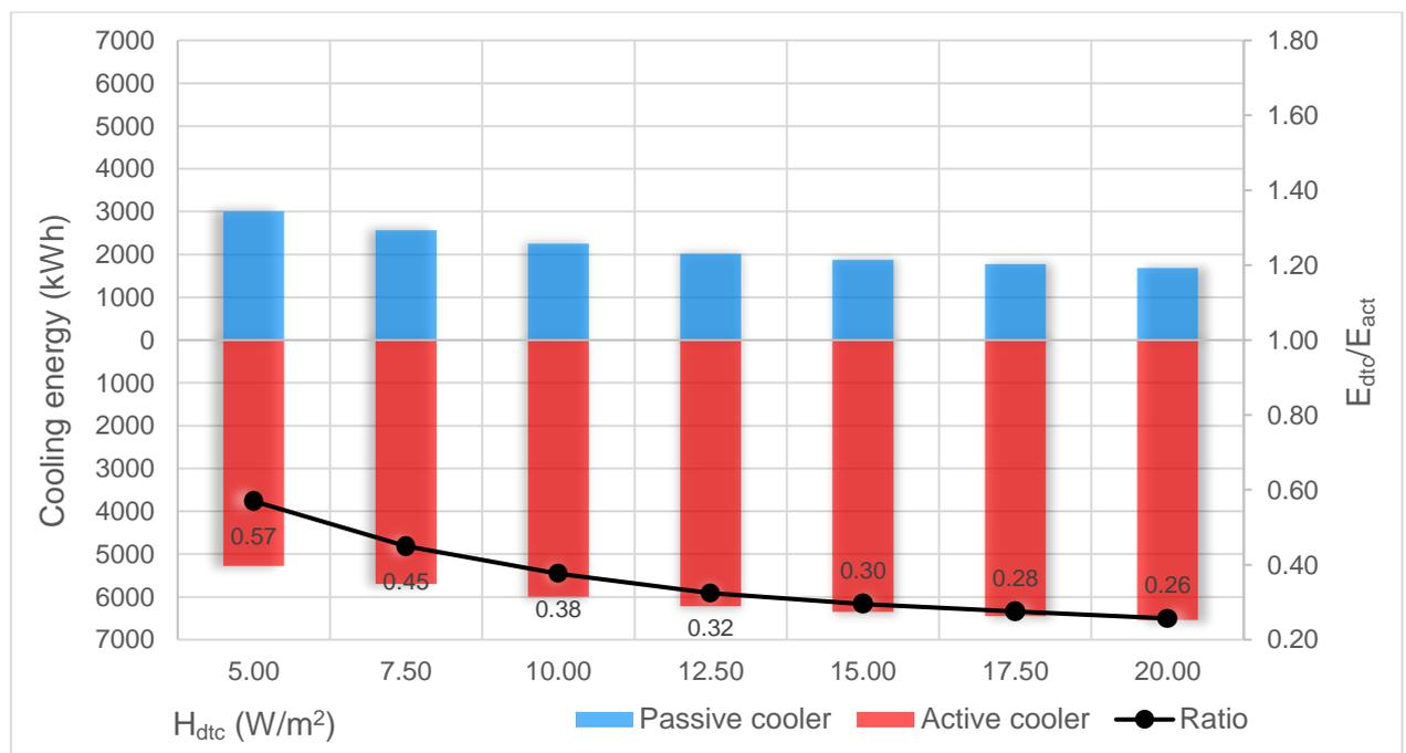
Figure 7-14. The sensitivity of the system to the effective heat transfer coefficient for values between 5 and  $20 \text{ W/m}^2$
