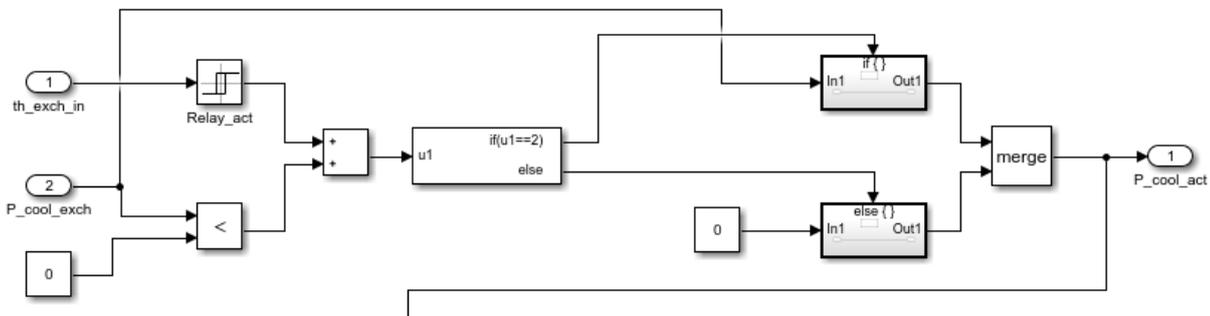
Figure B-8-10. Control mechanism of the active cooler.
