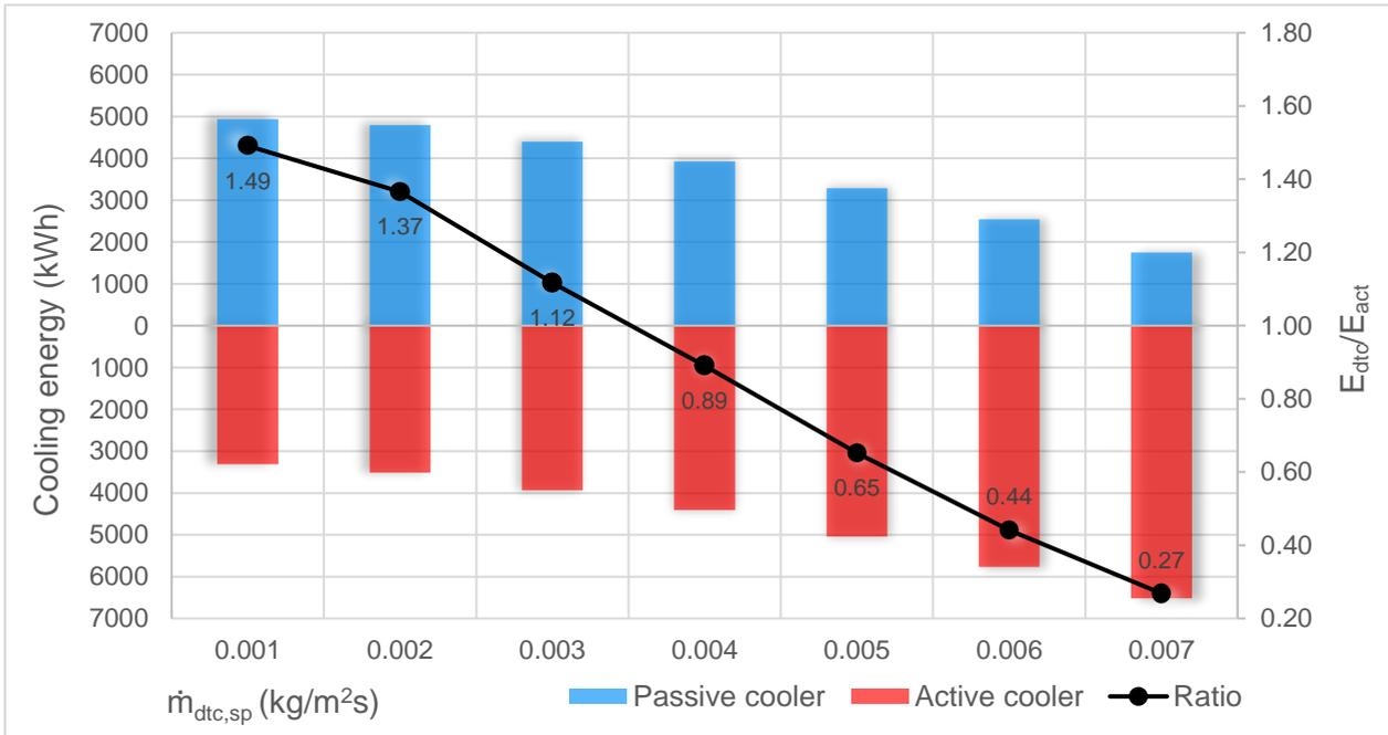
Figure 7-15. The sensitivity of the system to the mass flow rate of water within the passive cooler (> 0.001 kg/m<sup>2</sup>/s).
