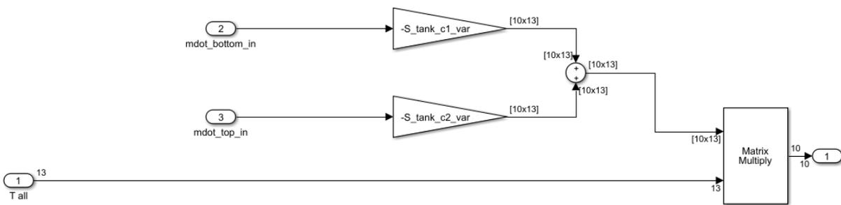
Figure B-8-13. Subsystem calculating the advective flows in the water tank.
