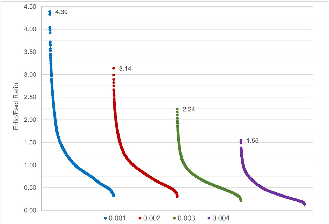
Figure 7-31. The Edtc/Eact ratio of the simulations grouped by the value of the specific mass flow rate within the daytime cooler (kg/m²s).
