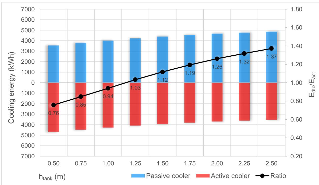
Figure 7-9. The sensitivity of the system to the height of the buffer tank.
