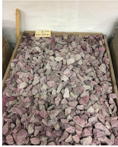
(b) Filter Material ( D_{N50}=3\text{cm} )
