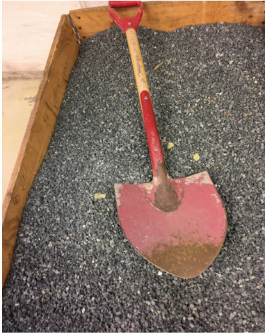
(a) Core Material ( D_{N50}=1.2\text{cm} )
