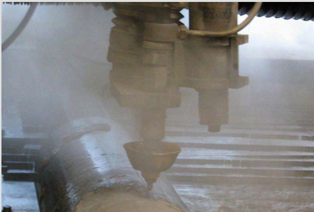
Figure 66: Marking the reference line on blade material
