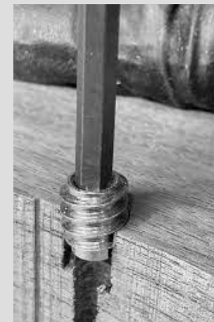
Figure 81: Partial insert in sandwich material & spar cap material & section view partial insert
