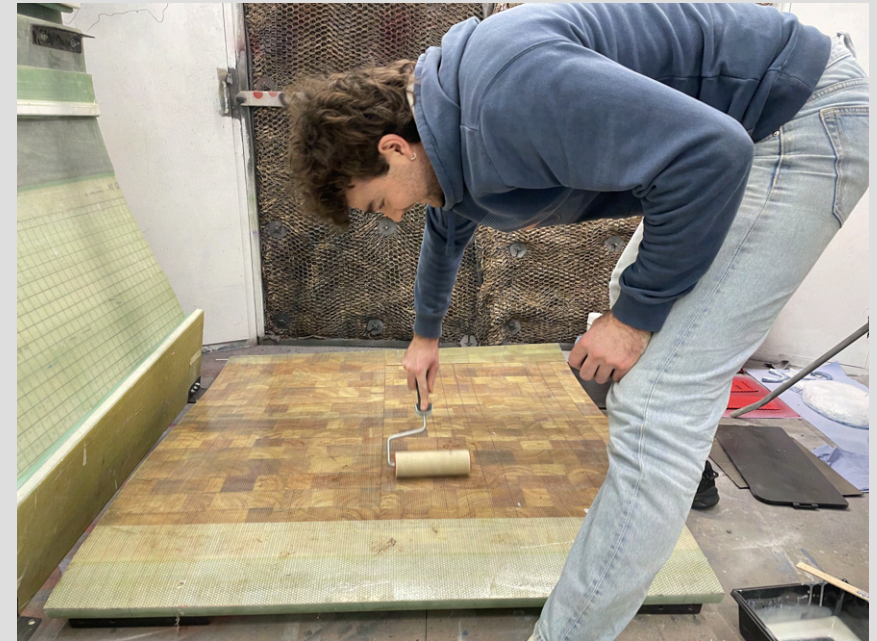
Figure 90.1: Applying bio based coating
