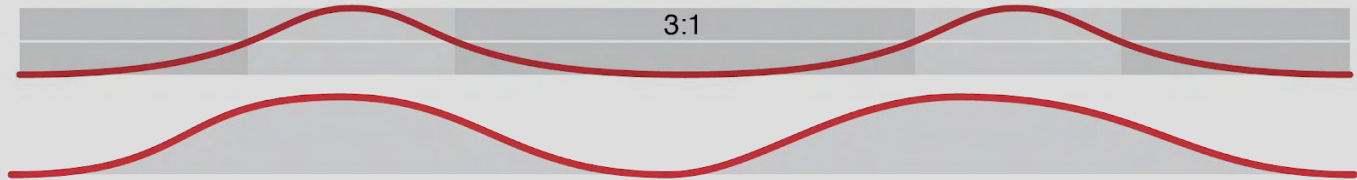
Figure 114: Pointy roller & shorter 'jumpable' rollers (Source: McCormack, 2019)
