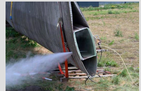
Figure 65: Echidna Diamond Saw (Source: Echidna.com.au), Diamond wire cutting (Source: Evan Wright, 2021), Waterjet cutting (Source: TNO),
