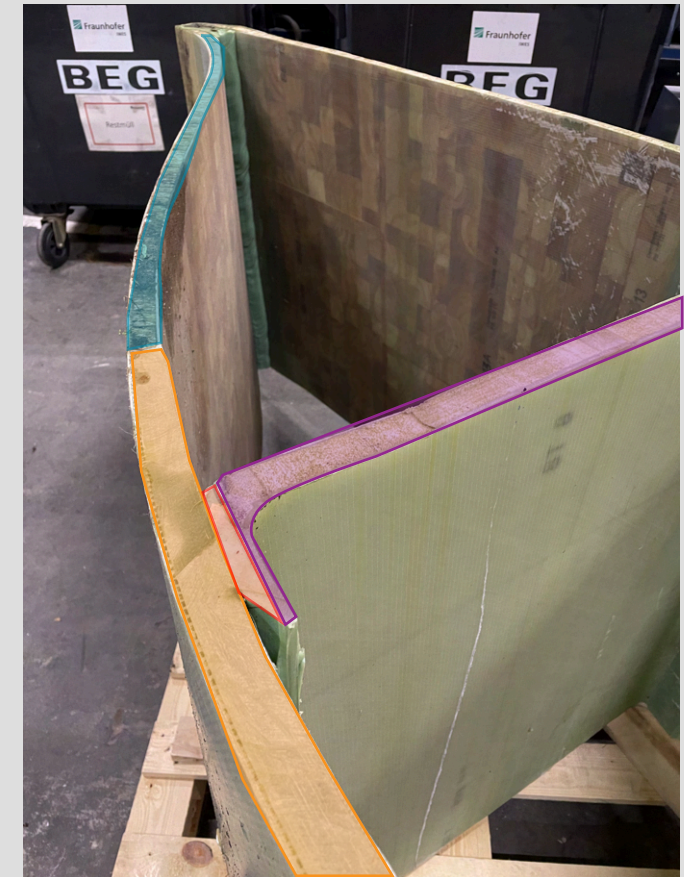
Figure 38 : spar cap glued to sandwich
