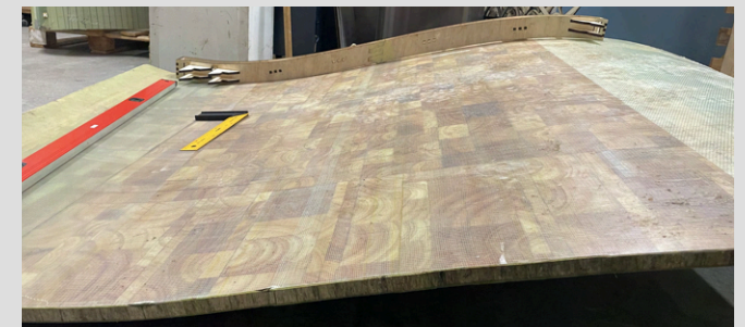
Figure 68: Matching the reference jig curve with the blade curve
