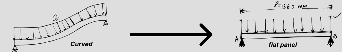
Figure 93: Simplification of distributed load on module
