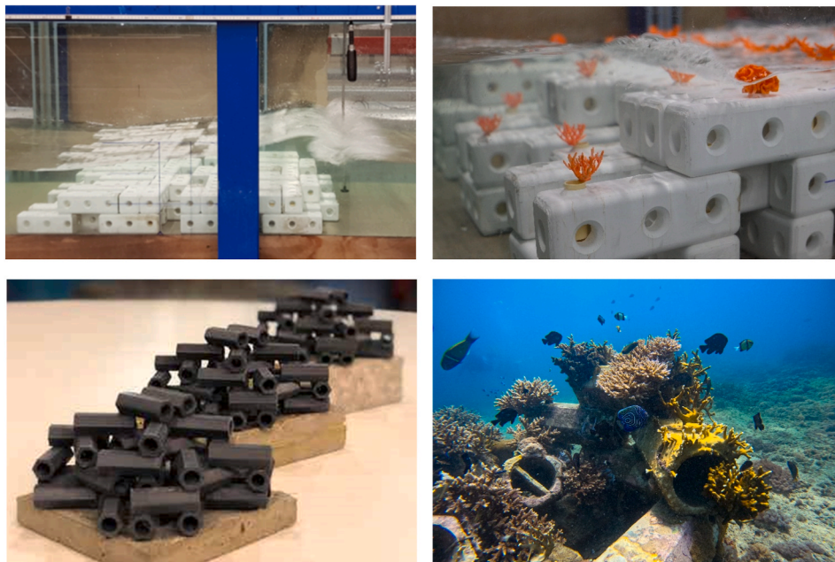
Fig. 1. Examples of artificial reef units: Upper: Reef enhancing breakwater by Reefy in wave flume (source: Van den Brekel, 2021); Lower: Moses by ReefSystems (Lower left: model tests by Van Diederren, 2022; Lower-right: application in practice).
