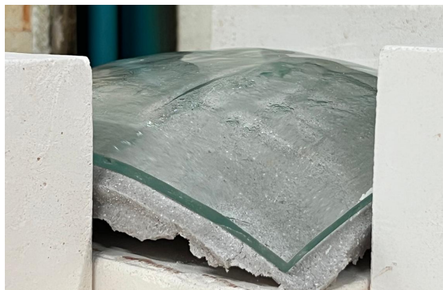
Fig. 4.30. In the two-step fusing process, after the second firing, the solid glass layer successfully slumped and conformed to the curved shape of the underlying foamed layer. However, the two layers did not bond together.
