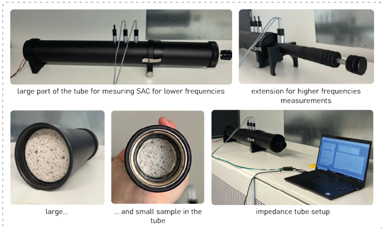
Fig. 3.30. Impedance tube setup used for measuring the sound absorption coefficient (SAC) of glass samples. The system includes a large-diameter tube for low-frequency measurements and an extension for higher frequencies. Both large and small cylindrical samples were tested by inserting them into the tube. The setup was connected to a laptop for data collection and analysis.
