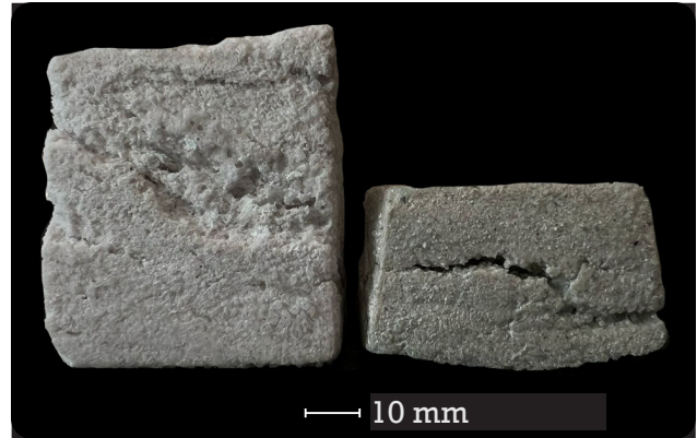
Fig. 3.25. From the left: SL10CCT1 and AM5CCT1. Horizontal cracks are visible on both samples. Additionally, shrinkage is observed on the automotive glass sample (AM5CCT1).
