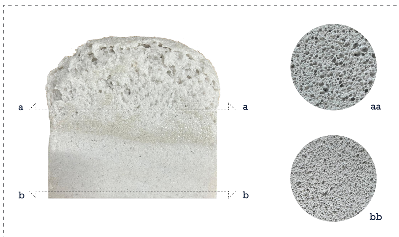
Fig. 3.23. Variation in pore size within a single sample, depending on the height of the section. Pores are typically smaller near the surface – where expansion is constrained by the mould – and larger in areas where the mixture was able to foam and expand freely outside the mould.
