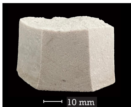
Fig. 4.32. Low-iron soda-lime glass after refoaming; no visible pores formed, but the sample retained a smooth and uniform internal structure.
