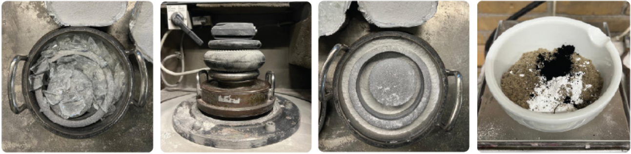
Fig. 3.7. a) Low iron soda lime cullet before and after milling in the Herzog milling machine. The cullet for almost all of the samples was milled for 6 seconds unless specified differently, b) Cyclon mix weighed with carbon black and dicalcium phosphate before mixing
