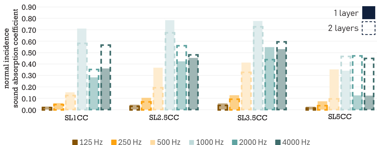
Fig. 3.41. Sound absorption comparison between single-layer and glued double-layer foam glass samples. The SAC values are generally comparable, with the double-layered samples occasionally showing slightly improved performance. SAC curves for these samples are shown in the Appendix.
