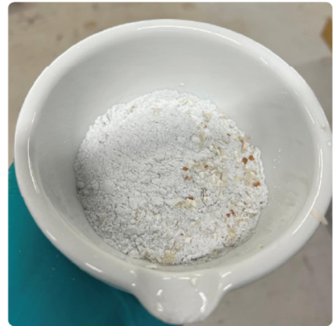
Fig. 3.16. Glass mixed with eggshells – larger particles of the foaming agent can be observed in the mixture
