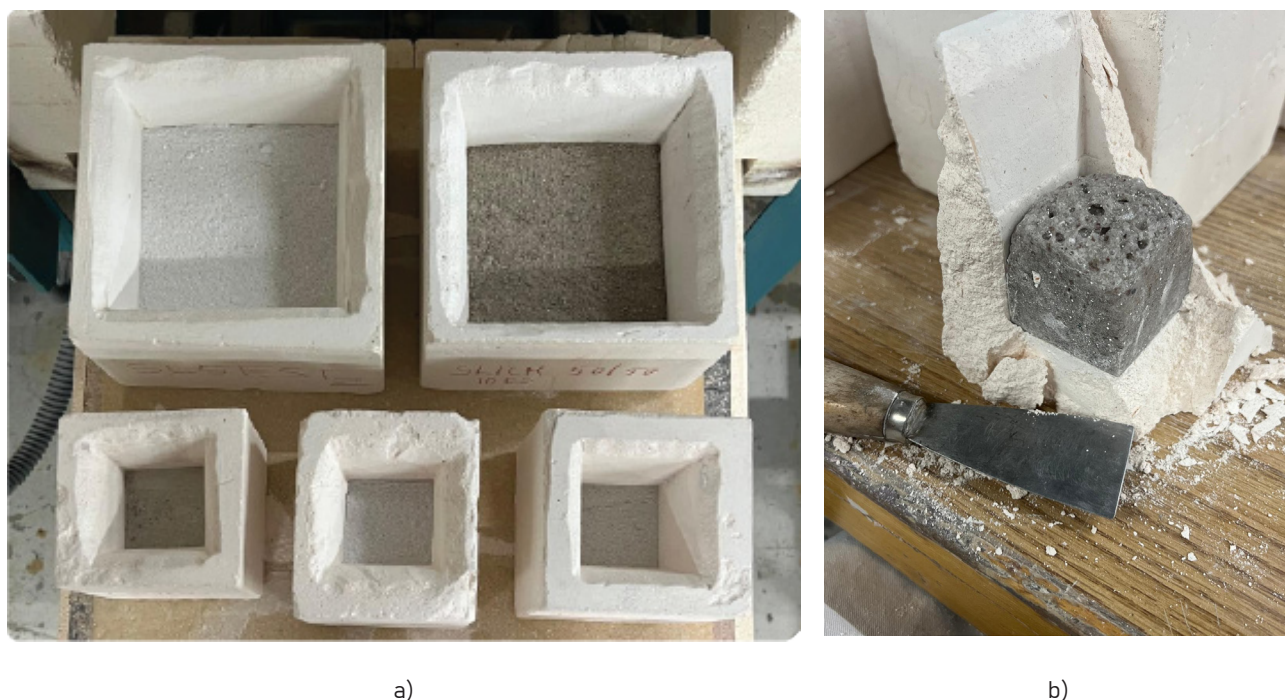
Fig. 3.5. a) Two types of mould used in the project; the small one (5 x 5 x 5 cm) for samples initial testing and the large one (12 x 12 x 6 cm) for development of larger samples for impedance tube testing, b) Extraction of the sample after firing.
