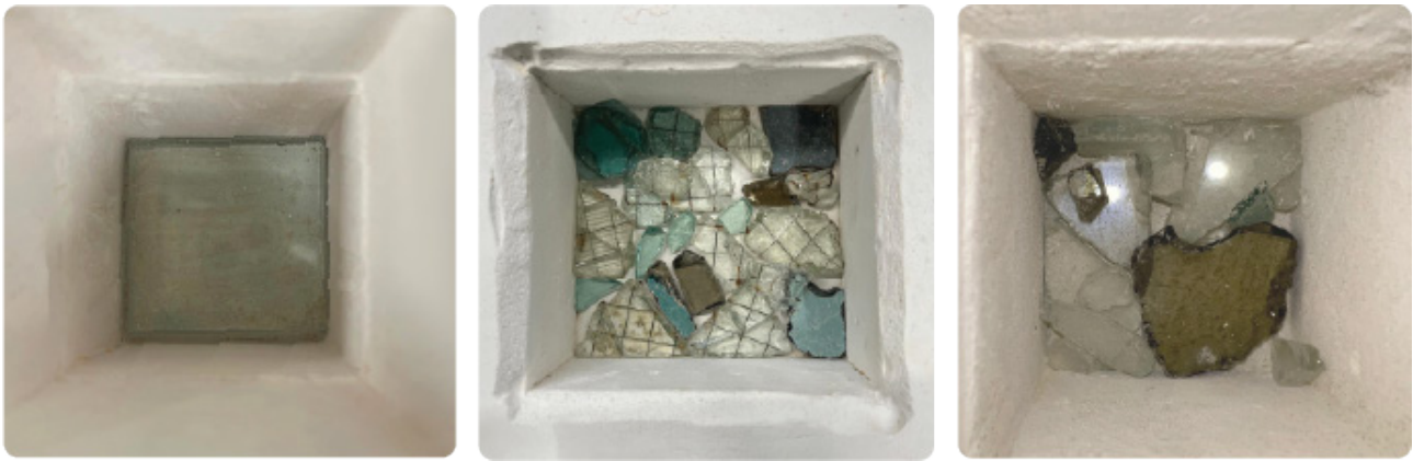
Fig. 3.26. Glass placed at the bottom of the mould to serve as the base layer for the foaming glass; a) Soda lime glass, later covered with foaming mixture, b) Mixed cullet, manually selected to include wiring and colorful glass pieces, then covered with foaming mixture, c) Mixed cullet, covered with foaming mixture (without manual selection)
