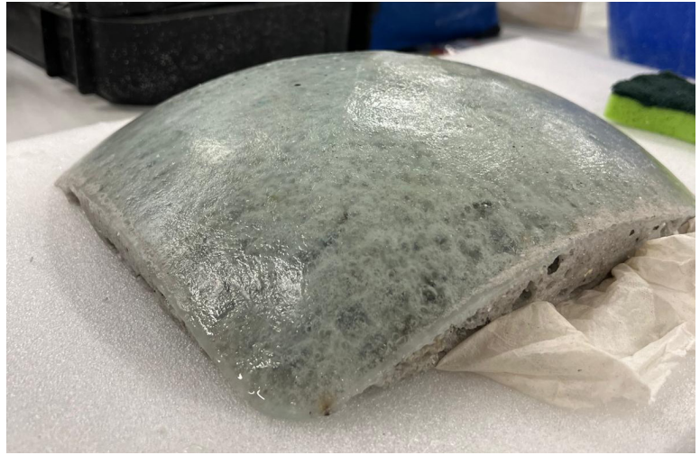
Fig. 4.27. Prototype of a single-step fused and foamed panel before post-processing. A curved panel produced by placing solid glass at the bottom of the mould and the foaming mixture on top. This image shows the result prior to polishing the solid surface.
