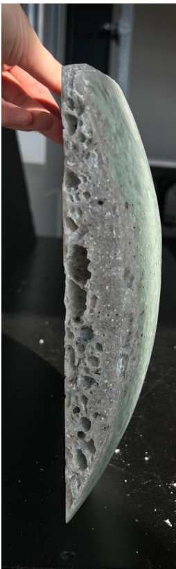
Fig. 4.28. Final prototype after post-processing. The single-step fused and foamed panel after polishing the solid glass surface. The result is a unified, curved element combining a transparent solid layer with a porous backing, demonstrating both structural integrity and acoustic potential.
