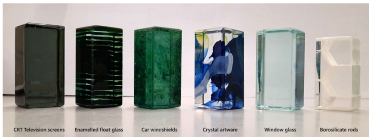
Fig. 2.12. Samples produced by kiln casting glass, incorporating glasses from various waste streams; source: Glass up-casting: A review on the current challenges in glass recycling and a novel approach for recycling 'as-is' glass waste into volumetric glass components," by T. Bristogianni & F. Oikonomopoulou, 2023, Glass Structures & Engineering , 8(2), p. 299 ( https://doi.org/10.1007/s40940-022-00206-9 ). Copyright 2023 by Springer Nature.
