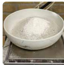
mixing glass with foaming agent
