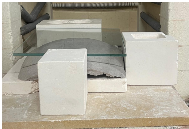
Fig. 4.29. Setup for two-step fabrication approach using a curved mould (own work). The foamed porous layer was first created separately, then reinserted into the kiln with a solid glass sheet on top for slumping and tack fusing.
