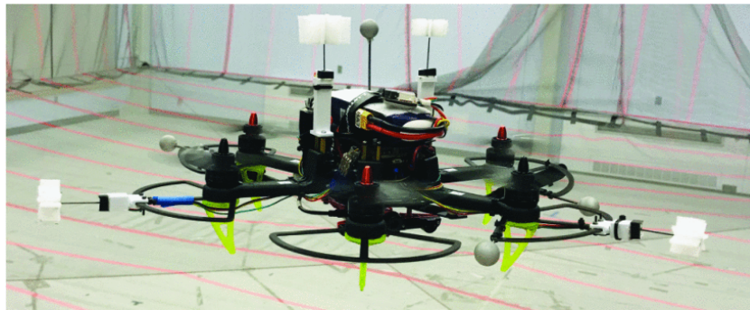
Figure 3.11: Airflow sensing on a multirotor equipped with four bio-inspired whisker-like sensors, enabling estimation of a 3D wind vector to distinguish aerodynamic drag from other forces. Adapted from [71].
