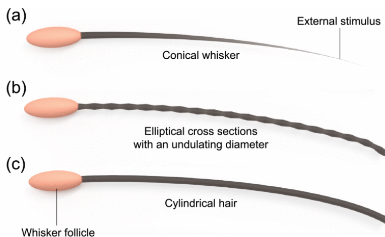
Figure 3.3: Overview of whisker shapes. (a) Rodents and large terrestrial mammals typically have conical whiskers. (b) Aquatic mammals, such as seals, possess whiskers with elliptical cross-sections and undulating diameters. (c) Cylindrical whisker sensors are sometimes used in whiskered robots. Adapted from [83].
