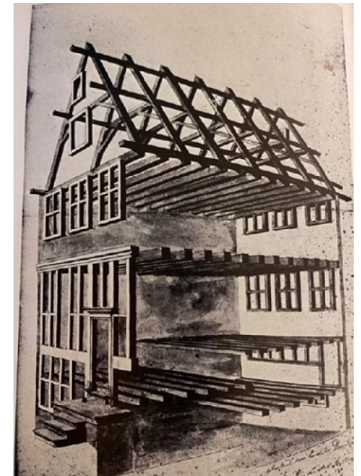
17th Century Carpentry Dutch Townhouse Construction Drawing, Source: Lecture Material of Dick van Gameren (2021)
