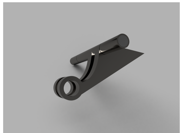
(b) Root hinge final design.
