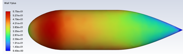
Figure A.1: Wall y^+ distribution of the fuselage selected after the trade-off prepared for the trade-off stimulation using k - \epsilon model.
