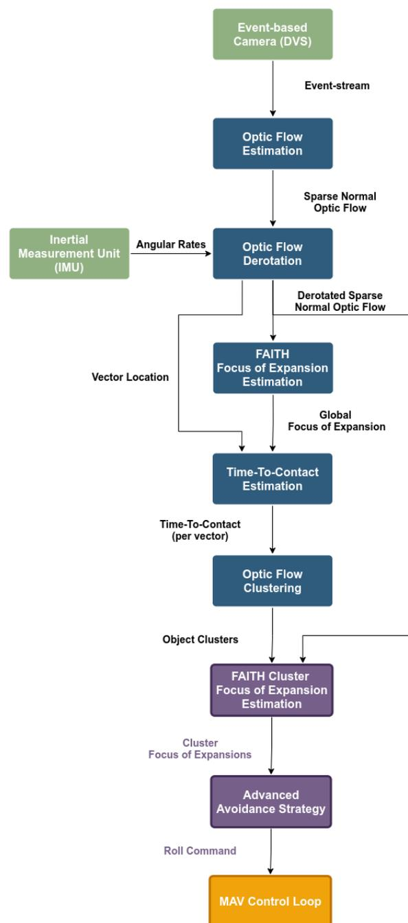
Figure 5.1: Processing flow for the obstacle avoidance system, using an advanced obstacle avoidance strategy. Green elements are sensors onboard the MAV, blue elements are processing steps, the purple elements are the advanced obstacle avoidance strategy and the yellow element is the MAV control loop. The arrows with labels show the output from functions and their connection to other functions.
