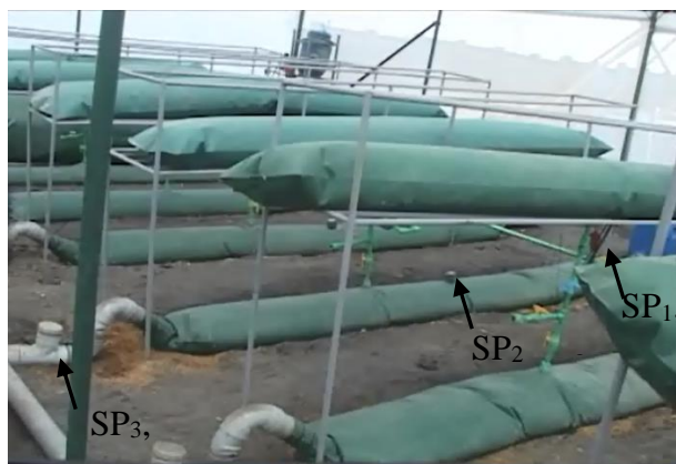
Figure 5.1 Plug flow digester layout; digesters on the floor, biogas collection bags directly above; sampling points at different length of the digester are indicated as SP_1 , SP_2 and SP_3 , respectively.
