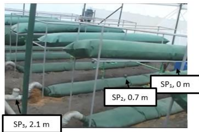
Figure 4.1: Plug flow digester layout: reactors on the floor, biogas collection bags directly above; sampling points are indicated (SP1, 2 and 3)
