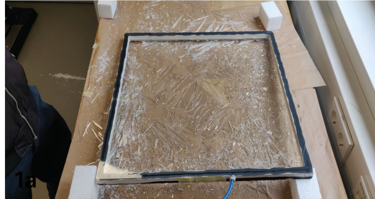
Shards from pane without film spread in all directions
