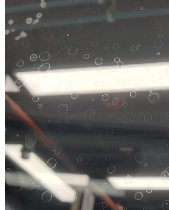
Safety film application errors made it unfit for testing
