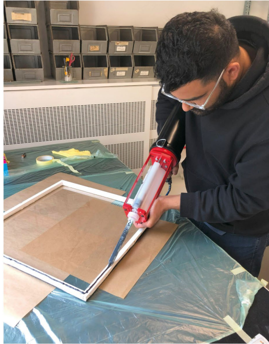
Applying glue using a pneumatic gun
