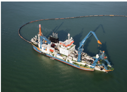
(a) Cutter Suction Dredger Athena
