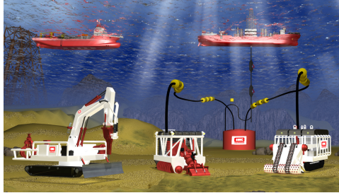
Figure 1.2: Preliminary designs of deep sea mining vehicles, courtesy of Royal IHC
