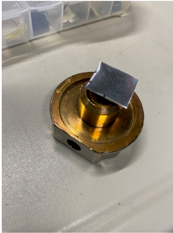
Figure 3.15: LASHPOL specimen A03 fixed in the SEM sample holder
