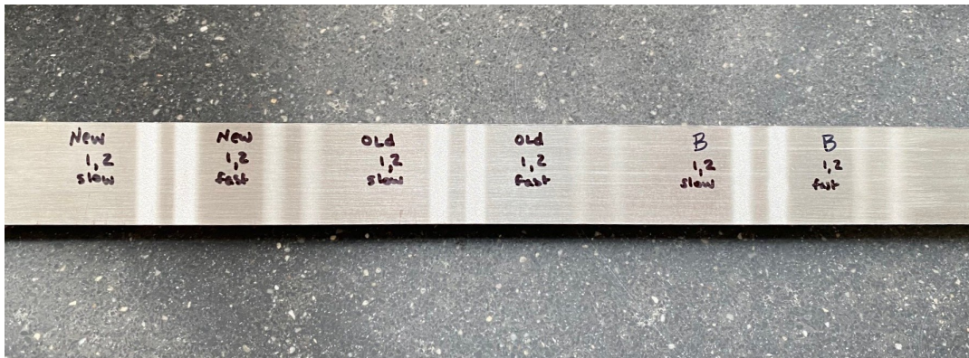
Figure 4.51: AA6061 plate sprayed with each of the AA6061 powders at different traverse speeds: slow is 20 mm/s, fast is 500 mm/s. The numbers 1 and 2 indicate the first and second deposits for each section according to the programmed path
