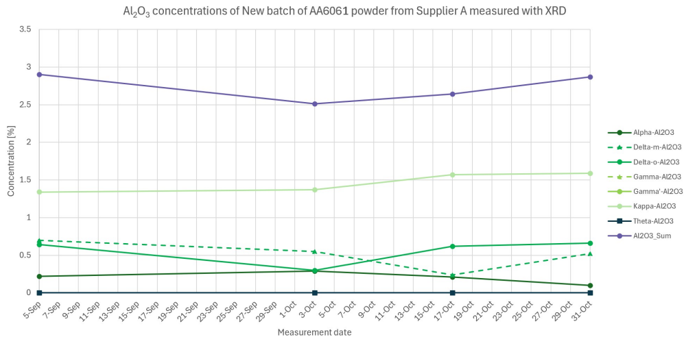
Figure 4.17: Concentration of Al 2 O 3 forms present in XRD refinement of the New batch of AA6061 powder from Supplier A by measurement date, with the sum of all contributions also plotted
