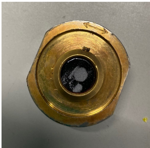
Figure 3.3: Powder from the New batch of AA6061 from Supplier A prepared in the sample holder for measurement from October 6 2025
