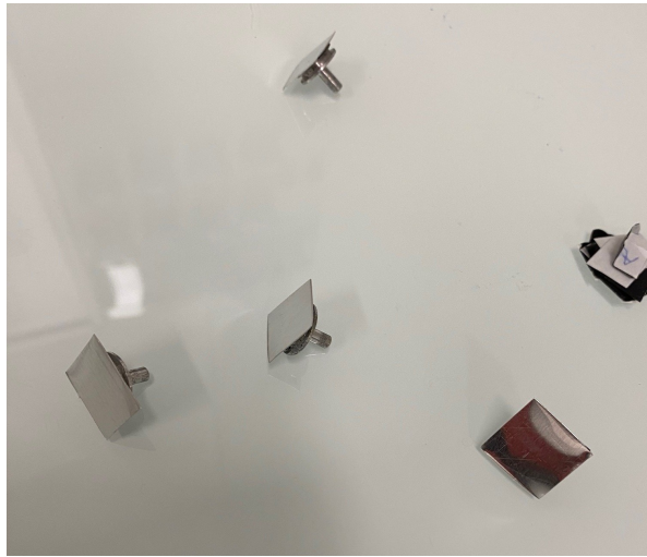
Figure 3.9: Receivers prepared with thin sheet 1xxx aluminum
