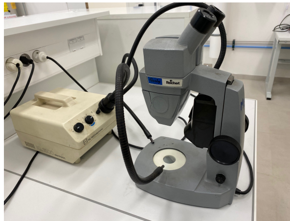
Figure 3.5: Microscope for single particle placement and alignment on particle launchers
