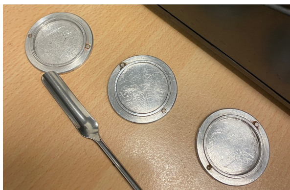
Figure 3.1: Empty powder sample holders for the XRD
