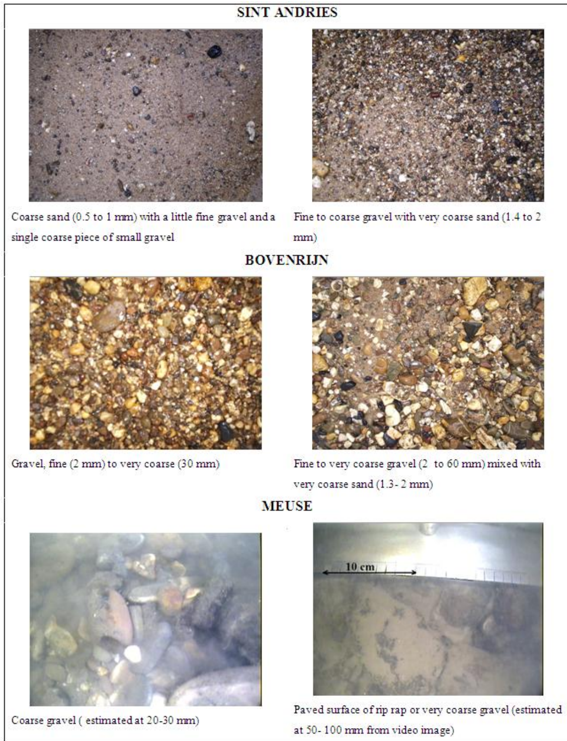
FIG. 6.3. Pictures of grab samples taken from the surveyed areas.
