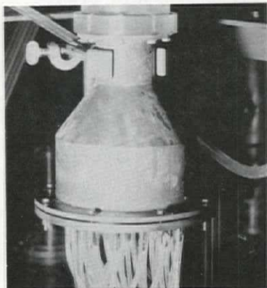
FIGURE 20. A- The bottom of the shock tube. The cone enables the mounting of the bottom plate with a number of capillary tubes. B- Detail of the bottom plate. The capillary tubes have an inner diameter of 10^{-4} m, an outer diameter of 5 \times 10^{-3} m and a length of 2.5 \times 10^{-2} m.
